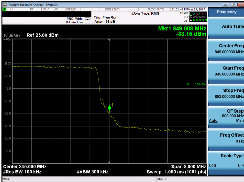
Plot 7-25. Upper Band Edge Plot (Band 5 – 10.0MHz QPSK – RB Size 50)
