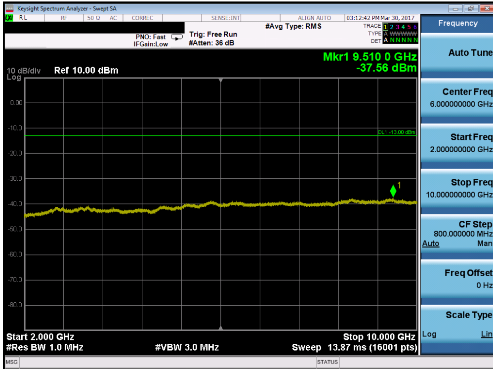
Plot 7-22. Conducted Spurious Plot (Cellular WCDMA Mode – Ch. 4233)
