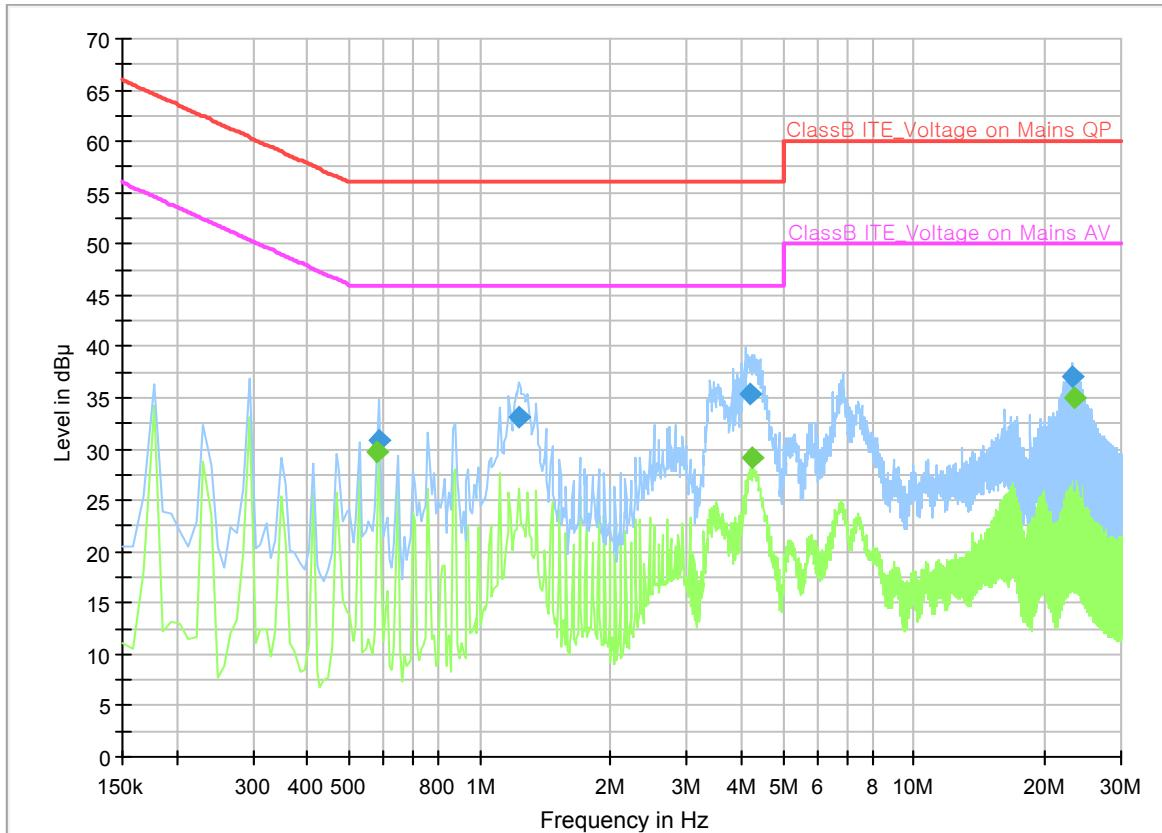
Note 1) Two graphs measured for both Live(L1) and Neutral(N) of the LISN are combined into one graph.
