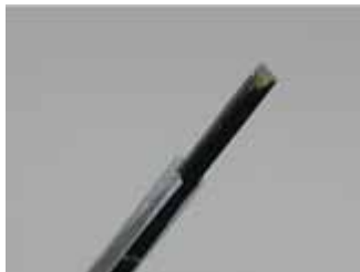
Figure 6. EX3DV4 E-field Probe
