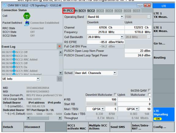
Select the SCC1/SCC2 tab, set operating band, BW, channel and RB configurations for SCC1/SCC2
