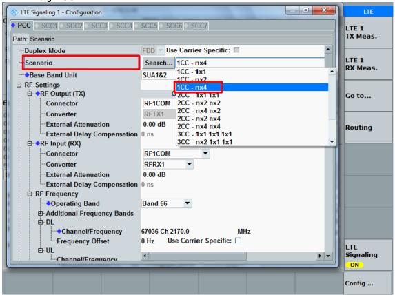
Set the RF Output/Input Connector and Converter for PCC.
