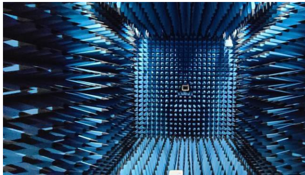
Figure 2: Geometry of Anechoic Chamber for Radiation patterns.
