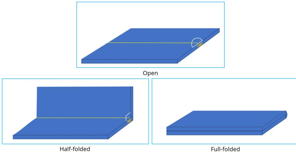
The fundamentals of the EUT were investigated in three orthogonal orientations X, Y and Z on 2TX MIMO mode. It was determined that X orientation and Open condition were the worst-case for 2TX MIMO mode.
