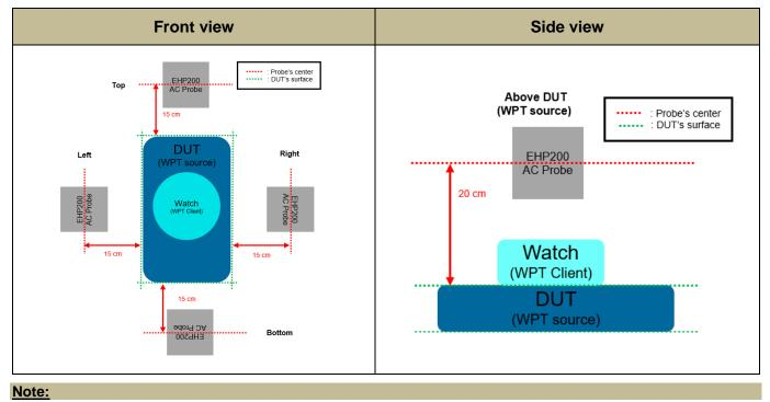
Test distance is the distance between DUT's surface to center of probe.
