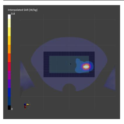
Measurement Report for SM-F946U, RIGHT TOUCH, Wi-Fi (U-NII Bands), IEEE 802.11ac WiFi (80MHz, MCS0, 90pc duty cycle), Channel 5855000 (5855.0 MHz)
