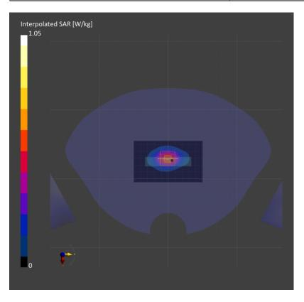
Measurement Report for SM-F946U, EDGE TOP, Band 41, LTE-TDD (SC-FDMA, 50% RB, 20 MHz, QPSK, UL Subframe=2,3,4,7,8,9), Channel 40620 (2593.0 MHz)
