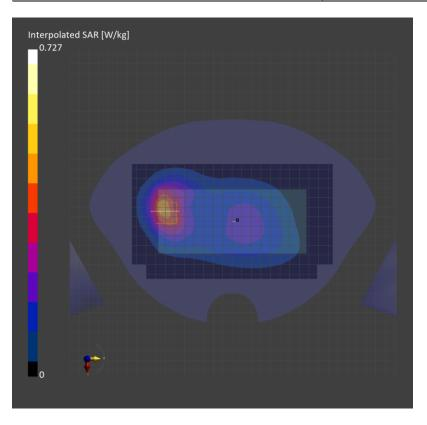
Measurement Report for SM-F946U, CHEEK, Band 7, LTE-FDD (SC-FDMA, 1 RB, 20 MHz, QPSK) RBPosition:Mid AntennaCfg:SISO, Channel 20850 (2510.0 MHz)
