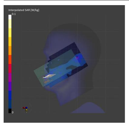
Measurement Report for SM-F946U, EDGE BOTTOM, Band n41 (Voice/data/SRSRO), 5G NR (DFT-s-OFDM, 50% RB, 100 MHz, QPSK, 30 kHz), Channel 518598 (2593.0 MHz)
