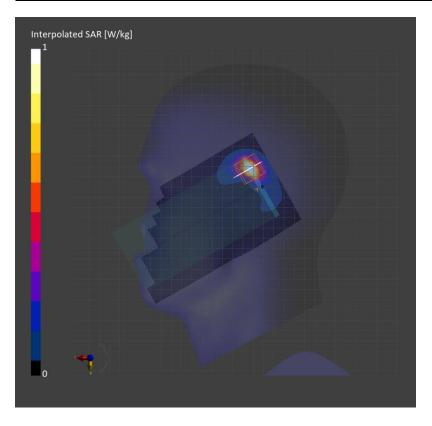
Measurement Report for SM-F946U, EDGE TOP, Band n48(Voice/data/SRS0), 5G NR (DFT-s-OFDM, 50% RB, 40 MHz, QPSK, 30 kHz), Channel 645332 (3680.0 MHz)
