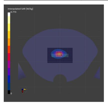
Measurement Report for SM-F946U, TILT, Band 7, LTE-FDD (SC-FDMA, 1 RB, 20 MHz, QPSK) RBPosition:High AntennaCfg:SISO, Channel 21350 (2560.0 MHz)
