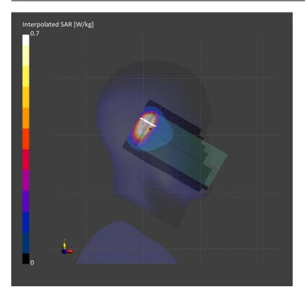
Measurement Report for SM-F946U, BACK, Band 7, LTE-FDD (SC-FDMA, 50% RB, 20 MHz, QPSK) RBPosition:High AntennaCfg:SISO, Channel 21350 (2560.0 MHz)
