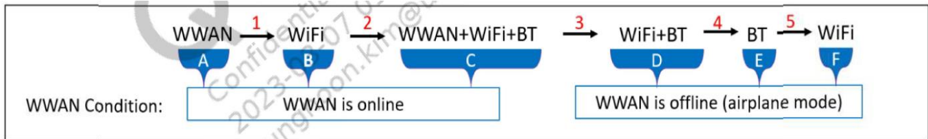
Figure S-1 Schematic of technology transitions for system level compliance continuity test.
