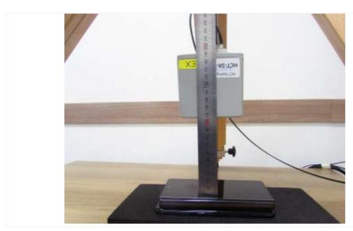
**Bottom : 15 cm** (The distance between the DUT and the center of the probe is 15 cm.)
