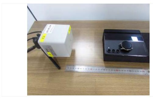
**Edge 1 : 15 cm** (The distance between the DUT and the center of the probe is 15 cm.)
