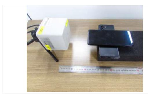
**Edge 4:15 cm** (The distance between the DUT and the center of the probe is 15 cm.)
