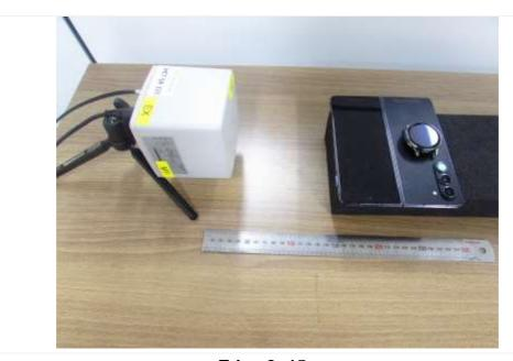
**Edge 2: 15 cm** (The distance between the DUT and the center of the probe is 15 cm.)
