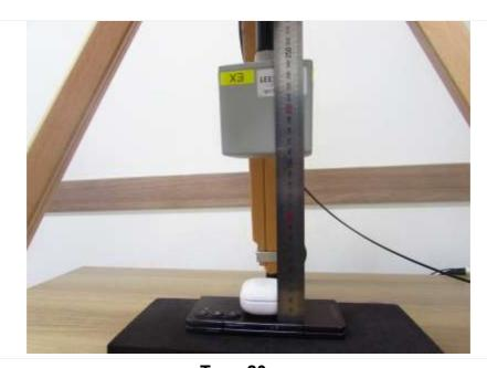
$\begin{tabular}{ll} \textbf{Top:20 cm} \\ \textbf{(The distance between the DUT and the center of the probe is 20 cm.)} \\ \end{tabular}$
