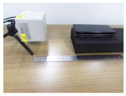
**Edge 1 : 15 cm** (The distance between the DUT and the center of the probe is 15 cm.)
