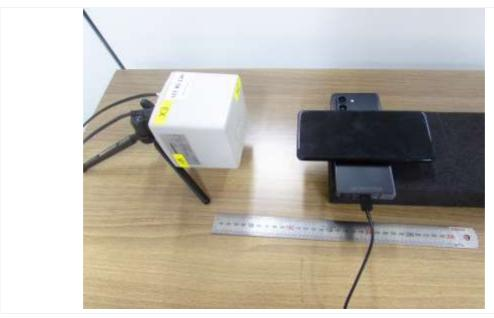
Edge 4 + TA : 15 cm (The distance between the DUT and the center of the probe is 15 cm.)
