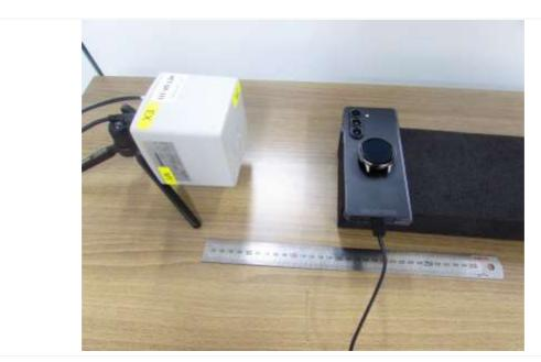
Edge 4 + TA : 15 cm (The distance between the DUT and the center of the probe is 15 cm.)
