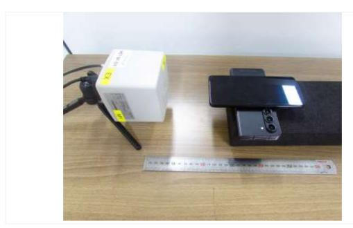
**Edge 2: 15 cm** (The distance between the DUT and the center of the probe is 15 cm.)
