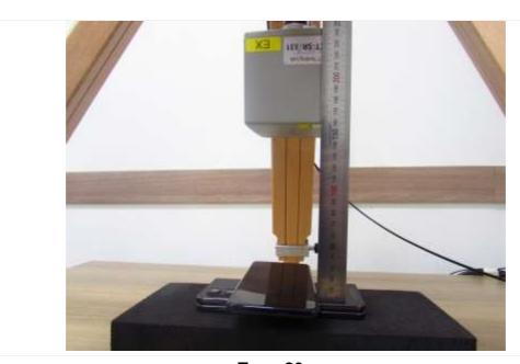
**Top: 20 cm** (The distance between the DUT and the center of the probe is 20 cm.)
