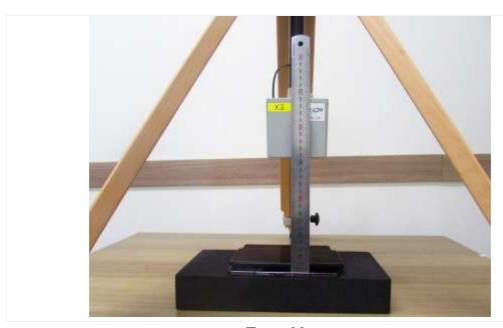
$\begin{tabular}{ll} \textbf{Top:20 cm} \\ \textbf{(The distance between the DUT and the center of the probe is 20 cm.)} \end{tabular}$
