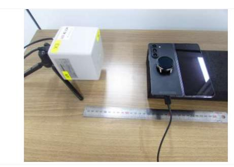
Edge 4 + TA : 15 cm (The distance between the DUT and the center of the probe is 15 cm.)
