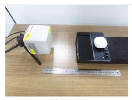
**Edge 2: 15 cm** (The distance between the DUT and the center of the probe is 15 cm.)
