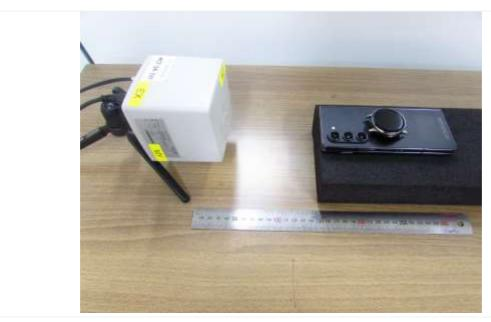
**Edge 1 : 15 cm** (The distance between the DUT and the center of the probe is 15 cm.)
