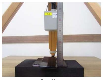
**Top: 20 cm** (The distance between the DUT and the center of the probe is 20 cm.)
