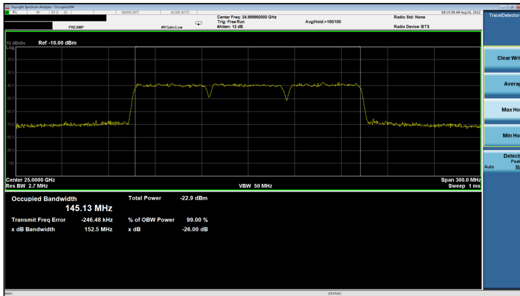
Plot 7-11. Occupied Bandwidth Plot (50MHz-3CC – 16QAM – Mid Channel)
