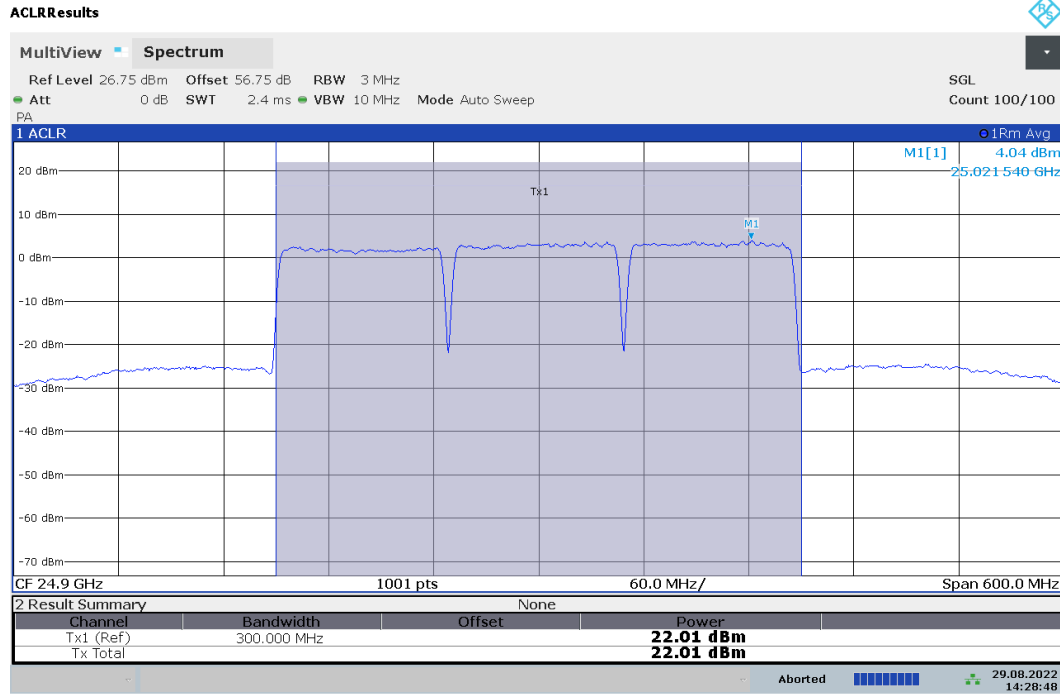
Plot 7-63. Ant1 EIRP Plot (Band n258-R2 - 100MHz-3CC - \pi/2 -BPSK - Low Channel)
