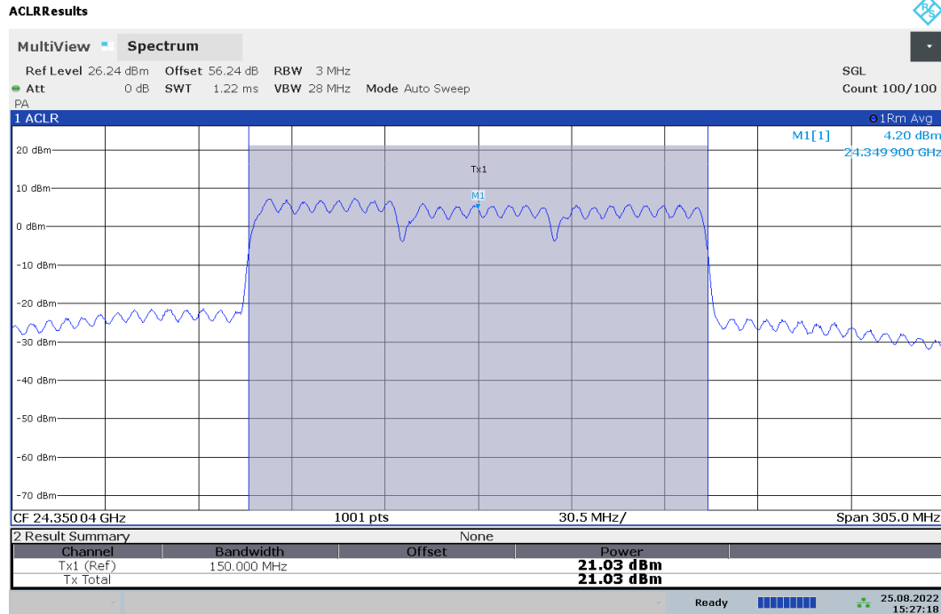
Plot 7-59. Ant2 EIRP Plot (Band n258-R1 - 50MHz-3CC - QPSK - Mid Channel)
