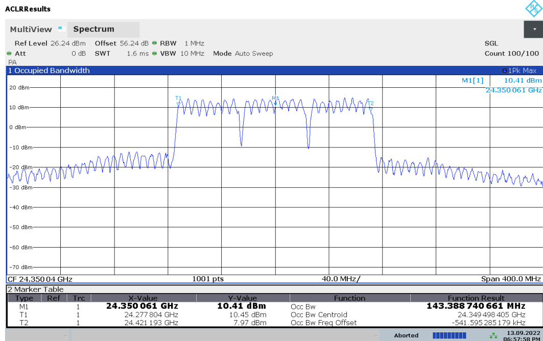
Plot 7-2. Occupied Bandwidth Plot (50MHz-3CC – \pi/2 -BPSK – Mid Channel)
