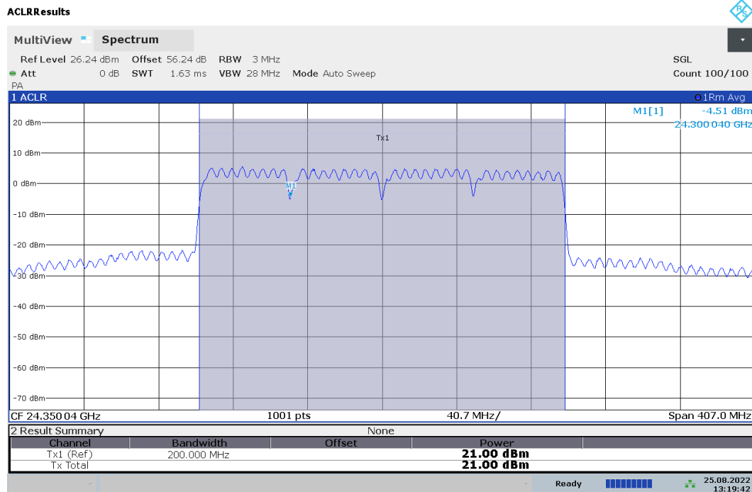
Plot 7-60. Ant2 EIRP Plot (Band n258-R1 - 50MHz-4CC - \pi/2 -BPSK - Mid Channel)
