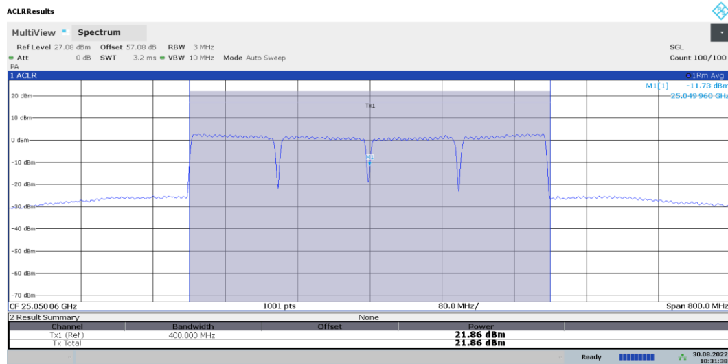
Plot 7-64. Ant1 EIRP Plot (Band n258-R2 - 100MHz-4CC - QPSK - High Channel)
