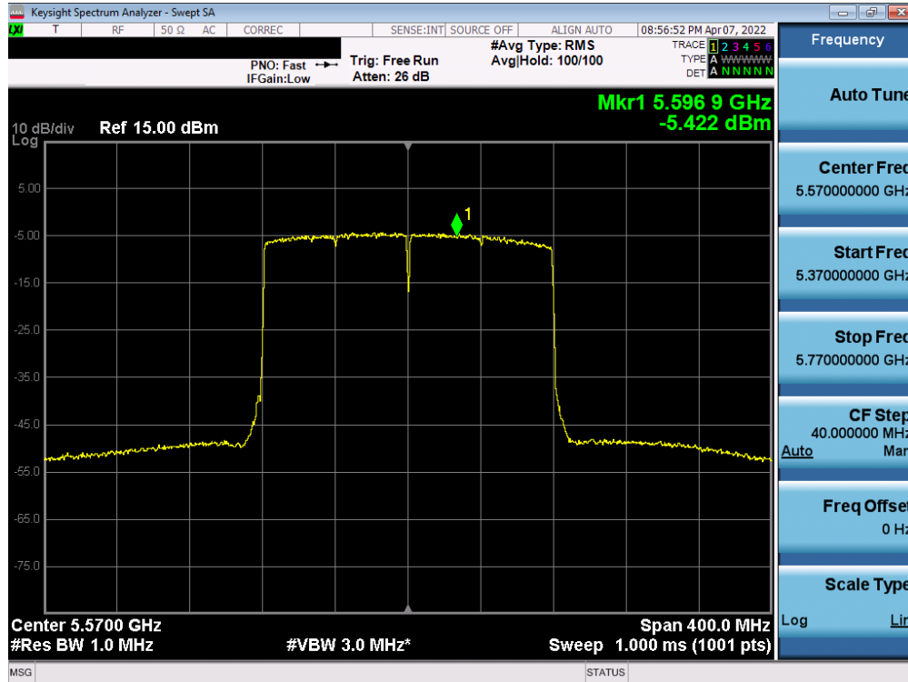
Plot 7-229. Power Spectral Density Plot MIMO ANT1 (160MHz BW 802.11ax (UNII Band 2C) – Ch. 114)
