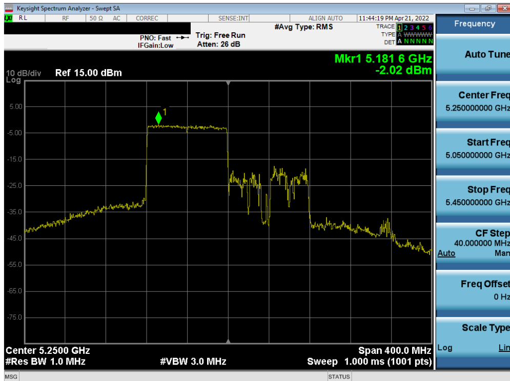
Plot 7-272. Power Spectral Density Plot MIMO ANT2 (160MHz (L) BW 802.11ax – Full Tones (UNII Band 1/2A) – Ch. 50)
