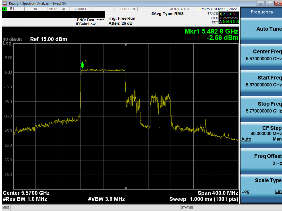
Plot 7-289. Power Spectral Density Plot MIMO ANT2 (160MHz BW (L) 802.11ax – Full Tones (UNII Band 3/4) – Ch. 163)
