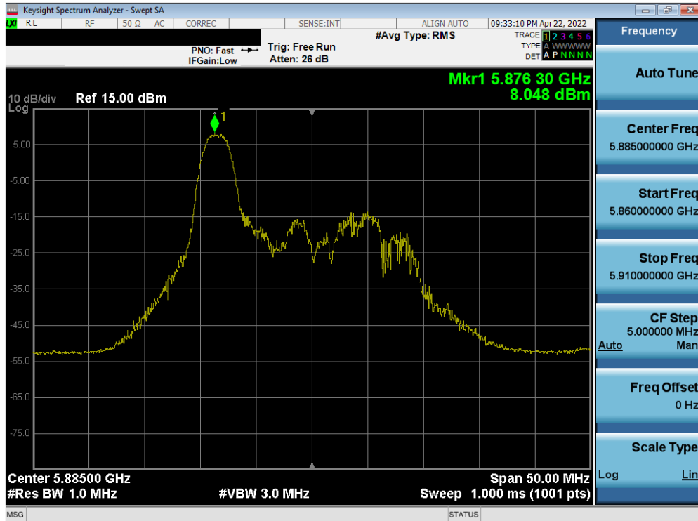
Plot 7-221. Power Spectral Density Plot MIMO ANT2 (20MHz BW 802.11ax – 26 Tones (UNII Band 4) – Ch. 177)
