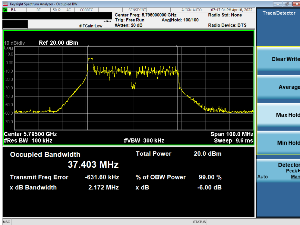
Plot 7-97. 6dB Bandwidth Plot MIMO ANT1 (40MHz BW 802.11ax – 26 Tones (UNII Band 3) – Ch. 159)
