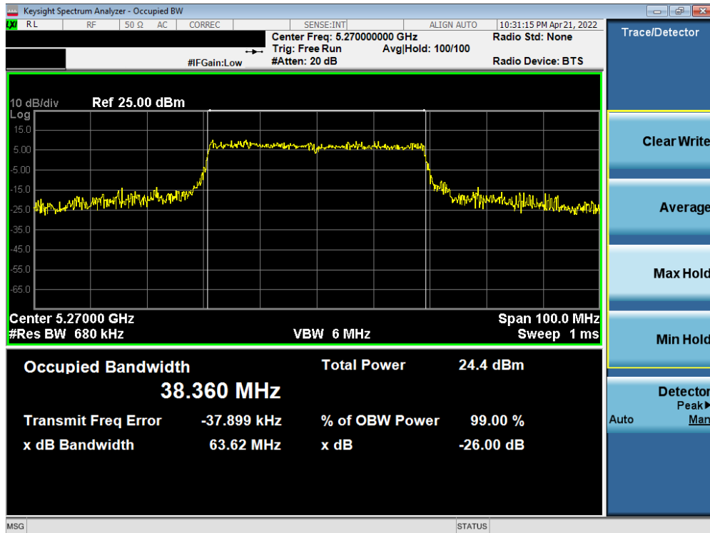
Plot 7-81. 26dB Bandwidth Plot MIMO ANT2 (40MHz BW 802.11ax – 484 Tones (UNII Band 2A) – Ch. 54)
