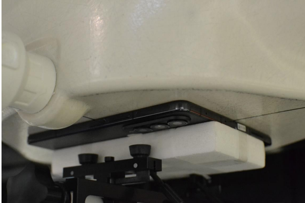
SAR Test Setup Photo 25– Open Configuration (UMPC), UMPC Extremity, Front Side, 0 mm
