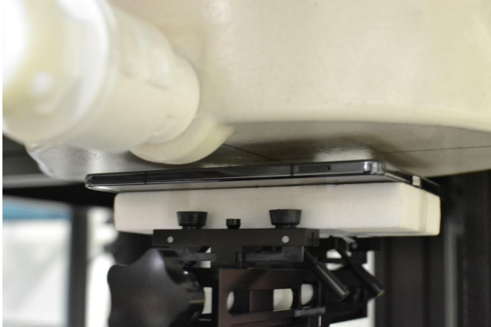
SAR Test Setup Photo 21– Open Configuration (UMPC), UMPC Body, Back Side, 10 mm
