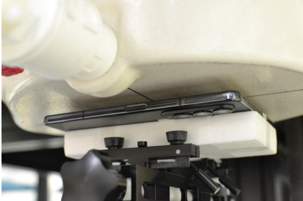
SAR Test Setup Photo 23– Open Configuration (UMPC), UMPC Body/Extremity, Front Side, 12 mm
