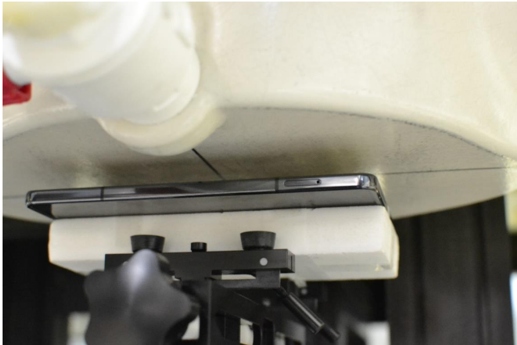
SAR Test Setup Photo 20– Open Configuration (UMPC), UMPC Body/Extremity, Back Side, 14 mm
