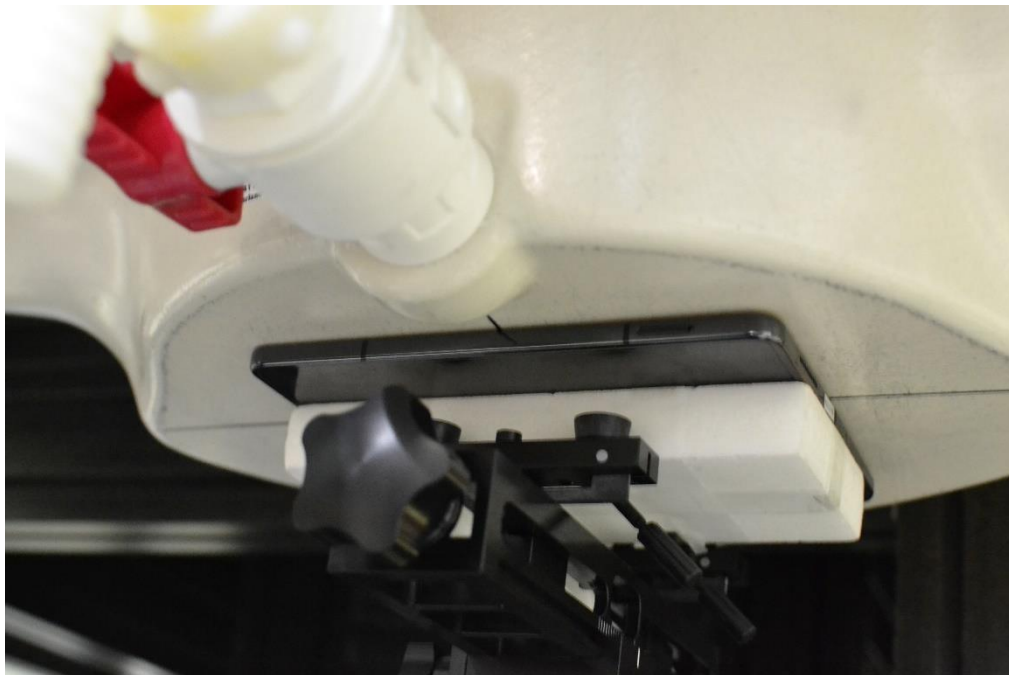
SAR Test Setup Photo 22– Open Configuration (UMPC), UMPC Extremity, Back Side, 0 mm
