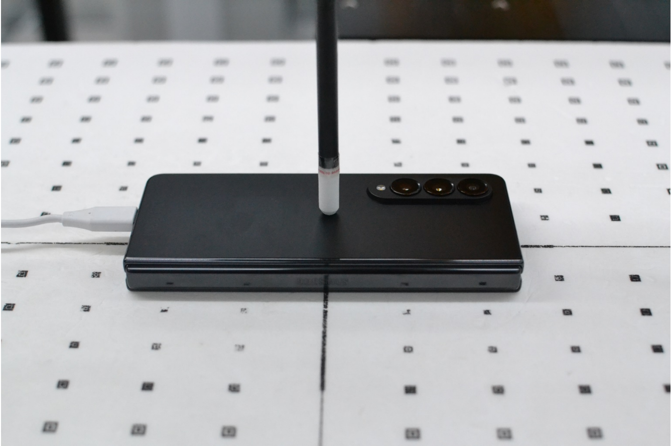
Figure E-4 Near Field Power Density Test Setup Photo – Back Side Closed at 2 mm
