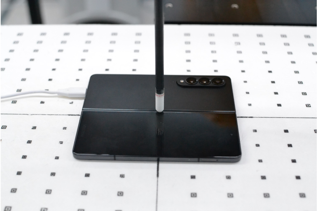
Figure E-6 Near Field Power Density Test Setup Photo – Back Side Open at 2 mm
