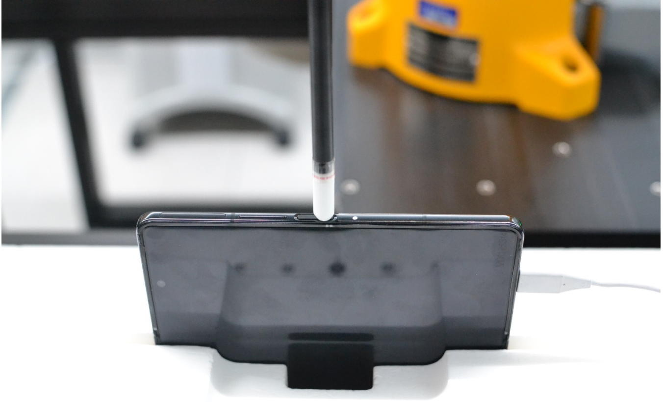
Figure E-8 Near Field Power Density Test Setup Photo – Right Edge Open at 2 mm
