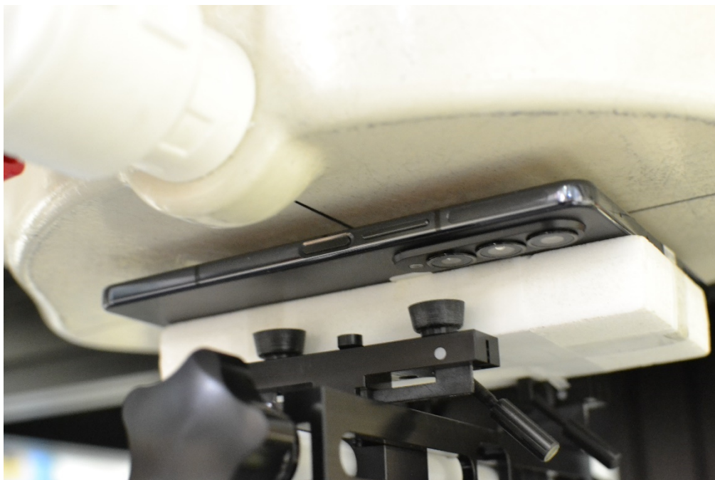
Figure F-17 SAR Test Setup Photo— Open Configuration (UMPC), UMPC Body, Front Side, 10 mm
