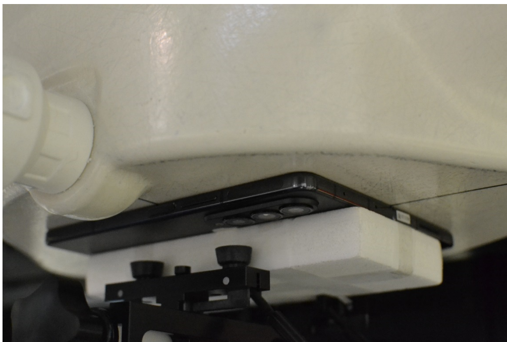
Figure F-18 SAR Test Setup Photo— Open Configuration (UMPC), UMPC Extremity, Front Side, 0 mm
