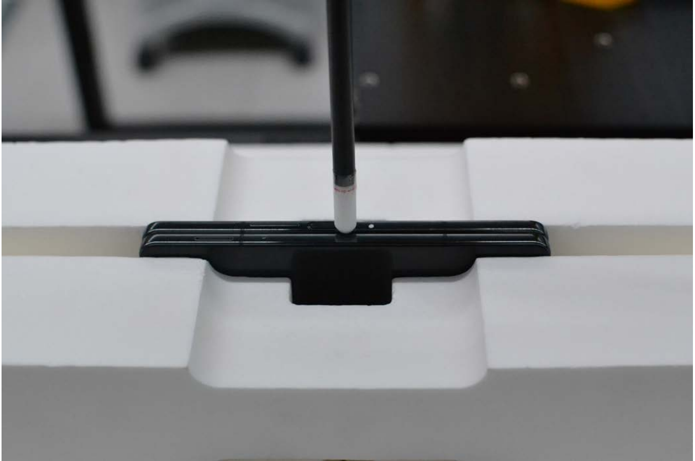
Figure F-35 Near Field Power Density Test Setup Photo – Right Edge Closed at 2 mm
