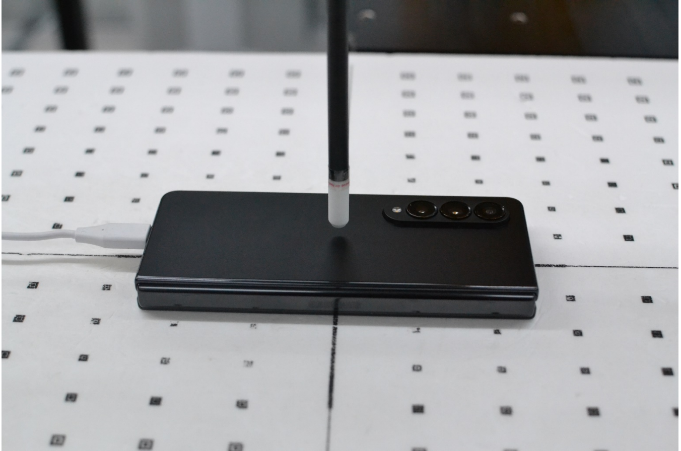
Figure F-27 Near Field Power Density Test Setup Photo – Back Side Closed at 9.89 mm
