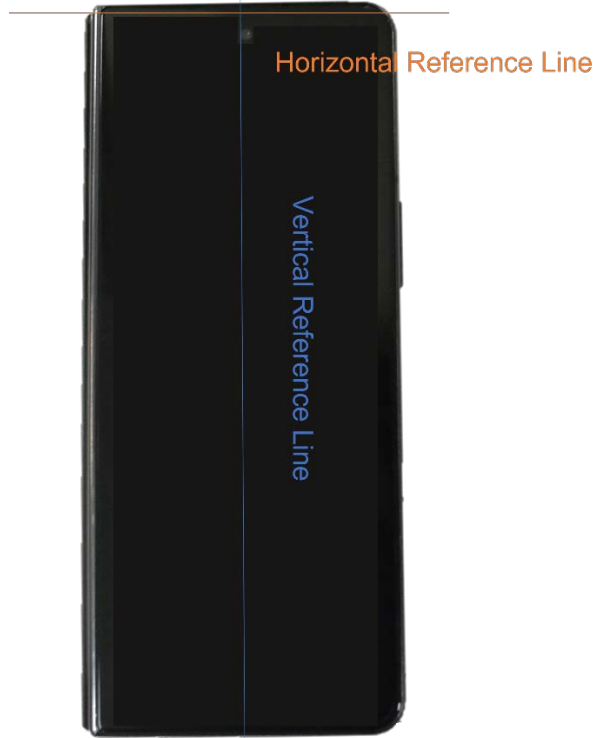
Figure F-25 SAR Test Setup Photo– Closed Configuration (Handset) Horizontal and Vertical Reference Lines
