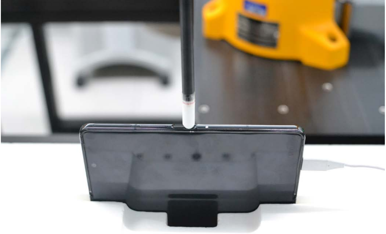
Figure F-36 Near Field Power Density Test Setup Photo – Right Edge Open at 2 mm
