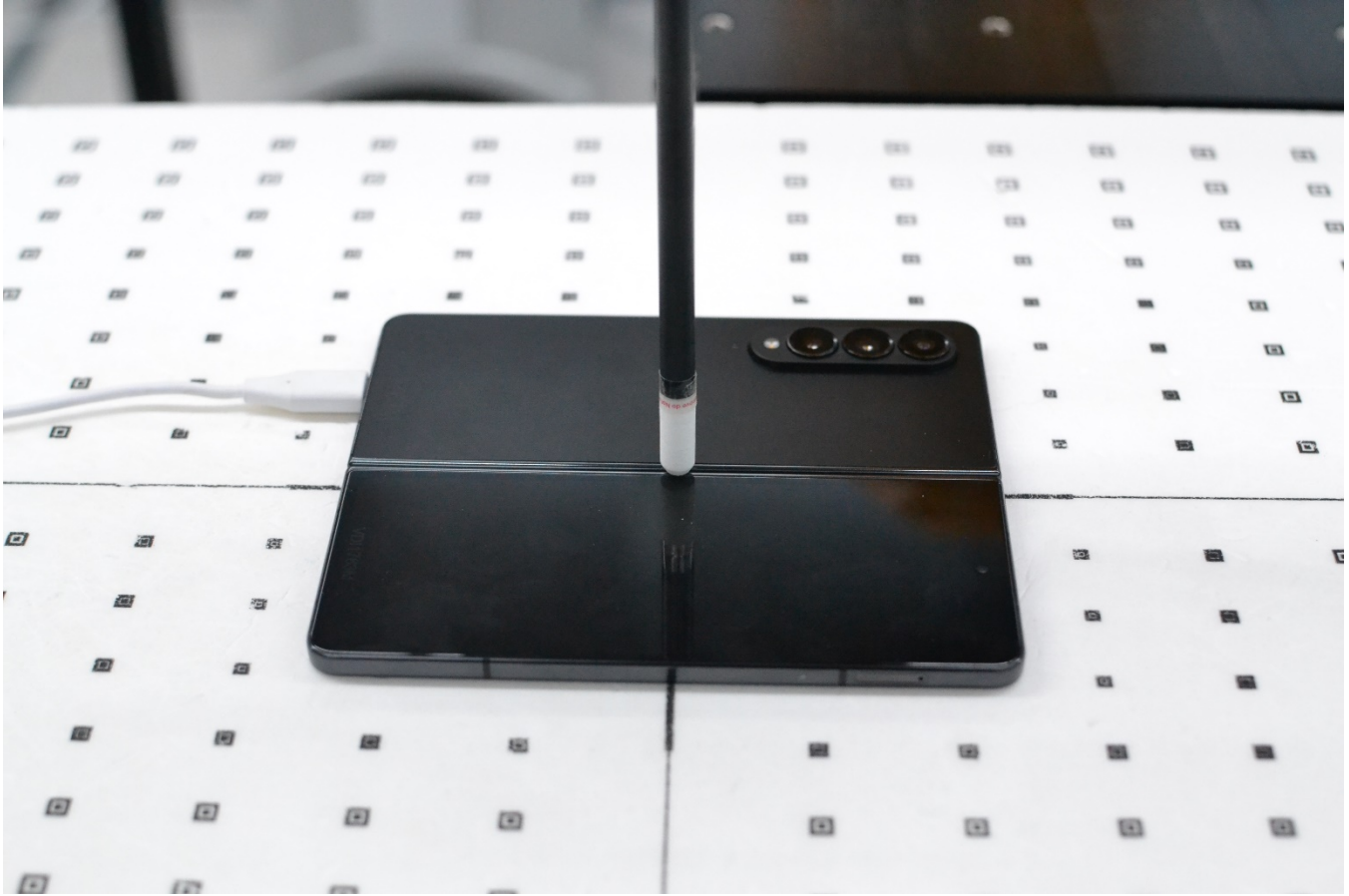
Figure F-28 Near Field Power Density Test Setup Photo – Back Side Open at 2 mm
