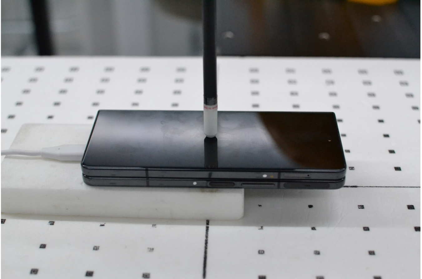
Figure F-29 Near Field Power Density Test Setup Photo – Front Side Closed at 2 mm
