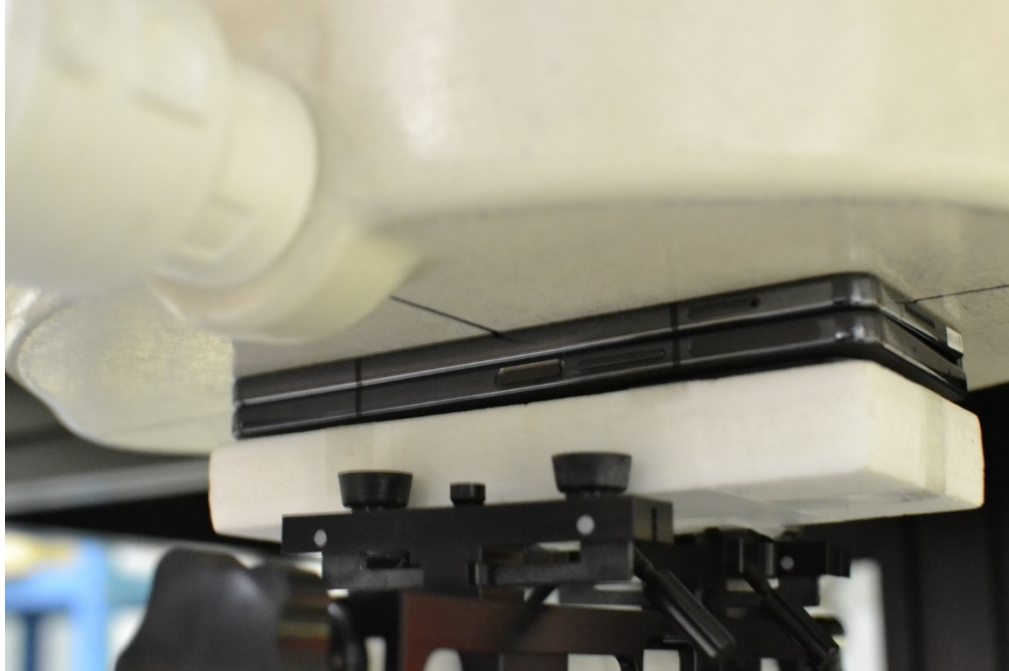
Figure F-10 SAR Test Setup Photo– Closed Configuration (Handset), Phablet, Front Side, 0 mm
