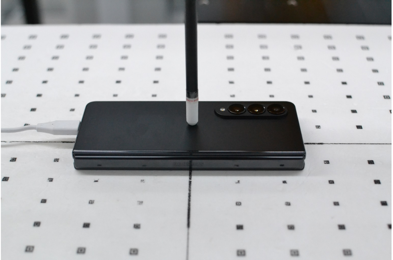
Figure F-26 Near Field Power Density Test Setup Photo – Back Side Closed at 2 mm
