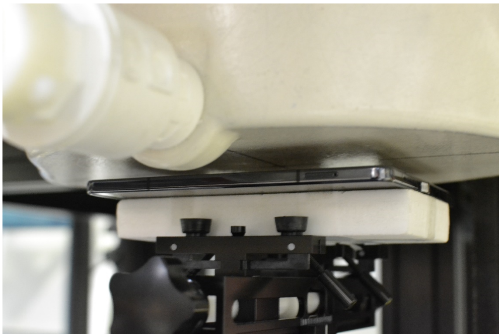
Figure F-15 SAR Test Setup Photo– Open Configuration (UMPC), UMPC Body, Back Side, 10 mm
