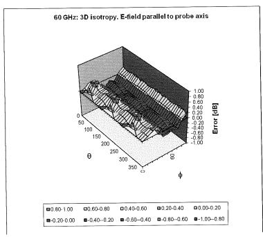
Probe isotropy for  $E_{tot}$ : probe rotated  $\phi$  = 0° to 360°, tilted from field propagation direction  $\vec{k}$  Parallel to the field propagation ( $\psi$  =0° - 90°) at 30 GHz: deviation within ± 0.45 dB Parallel to the field propagation ( $\psi$  =0° - 90°) at 60 GHz: deviation within ± 0.36 dB
