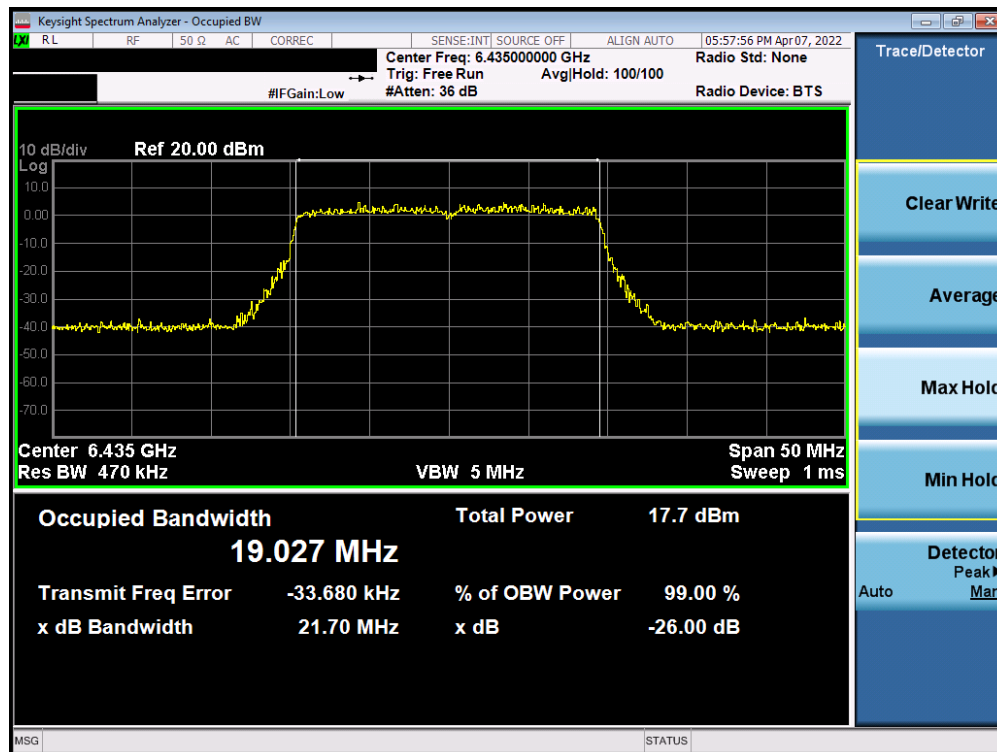
Plot 7-19. 26dB Bandwidth Plot MIMO ANT1 (20MHz 802.11ax (UNII Band 6) – Ch. 97)
