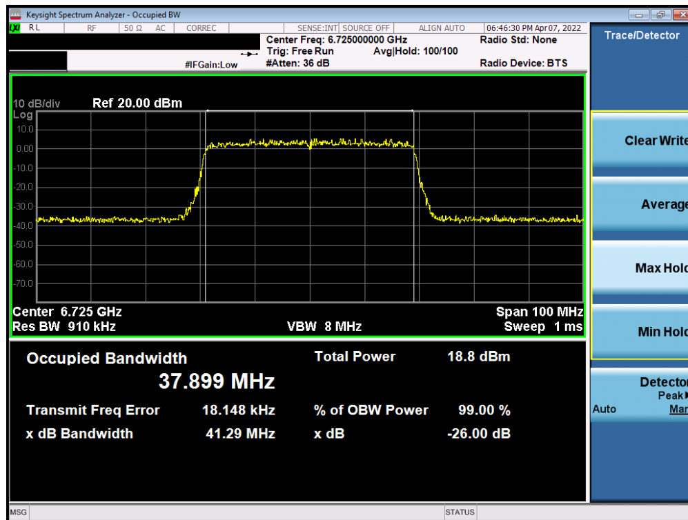
Plot 7-86. 26dB Bandwidth Plot MIMO ANT2 (40MHz 802.11ax (UNII Band 7) – Ch. 155)
