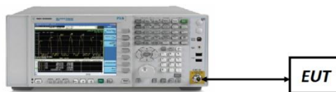
Figure 7-3. Test Instrument & Measurement Setup
