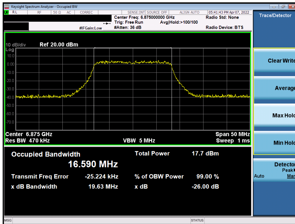
Plot 7-81. 26dB Bandwidth Plot MIMO ANT2 (20MHz 802.11a (UNII Band 7) – Ch. 185)
