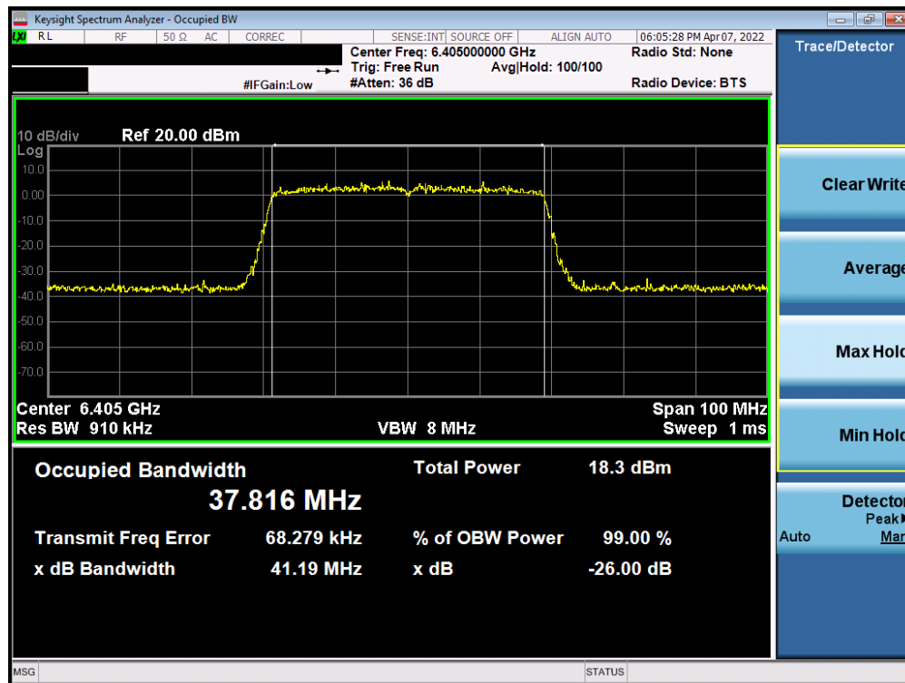
Plot 7-9. 26dB Bandwidth Plot MIMO ANT1 (40MHz 802.11ax (UNII Band 5) – Ch. 91)
