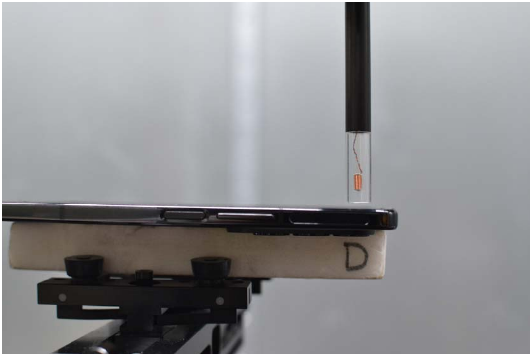
Figure 17-4 Test Setup for Wireless Device - OPEN (FRONT)
