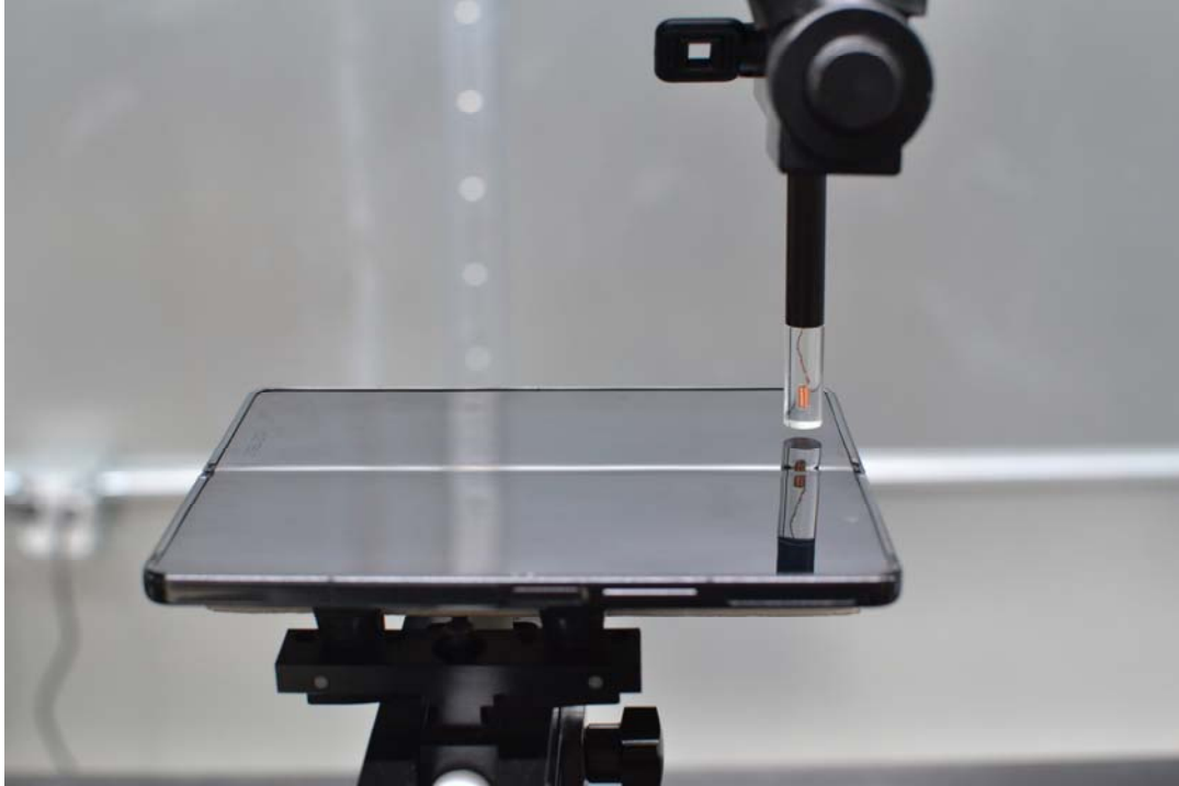
Figure 17-3 Test Setup for Wireless Device - OPEN (FRONT)
