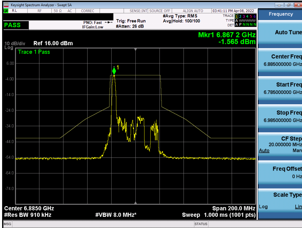
Plot 7-330. In-Band Emission Plot MIMO ANT1 (40MHz BW 802.11ax (26 Tones) (UNII Band 8) – Ch. 187)
