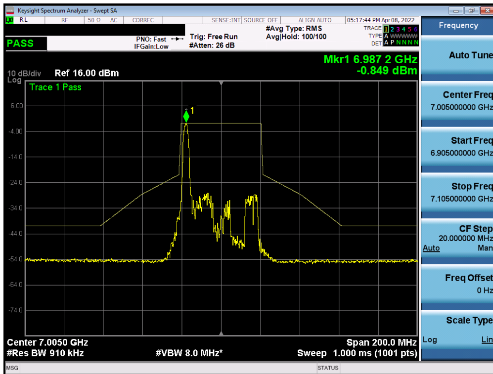
Plot 7-405. In-Band Emission Plot MIMO ANT2 (40MHz BW 802.11ax (26 Tones) (UNII Band 8) – Ch. 211)
