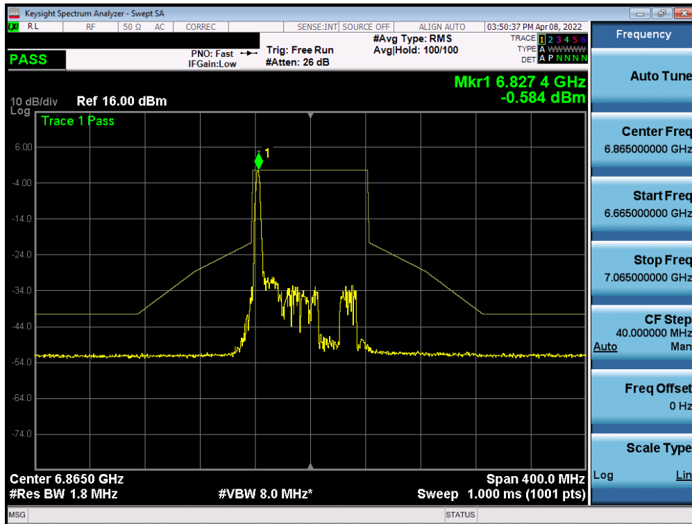
Plot 7-324. In-Band Emission Plot MIMO ANT1 (80MHz BW 802.11ax (26 Tones) (UNII Band 7) – Ch. 183)
