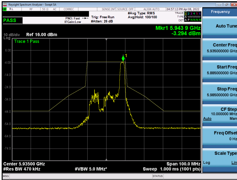
Plot 7-370. In-Band Emission Plot MIMO ANT2 (20MHz BW 802.11ax (26 Tones) UNII Band 5) – Ch. 2)
