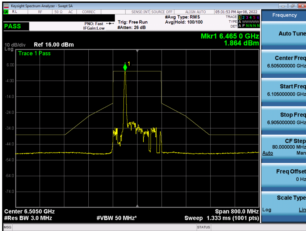
Plot 7-389. In-Band Emission Plot MIMO ANT2 (160MHz BW 802.11ax (26 Tones) (UNII Band 6) – Ch. 111)
