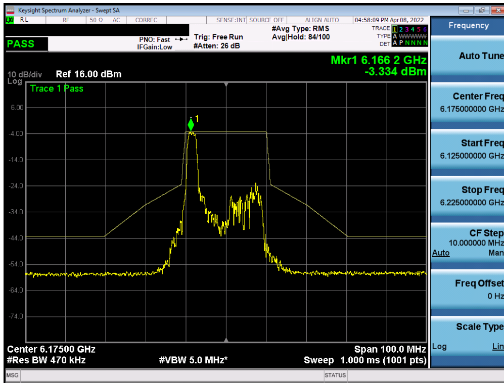
Plot 7-371. In-Band Emission Plot MIMO ANT2 (20MHz BW 802.11ax (26 Tones) (UNII Band 5) – Ch. 45)
