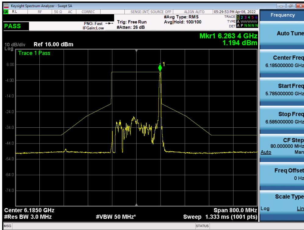
Plot 7-380. In-Band Emission Plot MIMO ANT2 (160MHz BW 802.11ax (26 Tones) (UNII Band 5) – Ch. 47)
