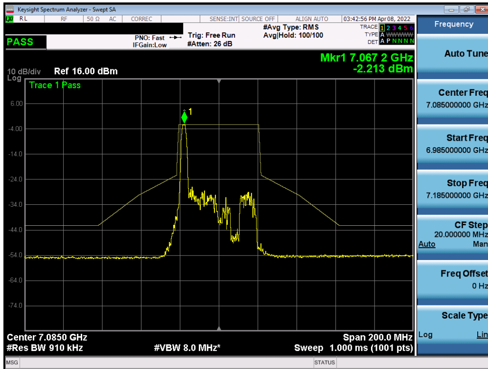
Plot 7-332. In-Band Emission Plot MIMO ANT1 (40MHz BW 802.11ax (26 Tones) (UNII Band 8) – Ch. 227)
