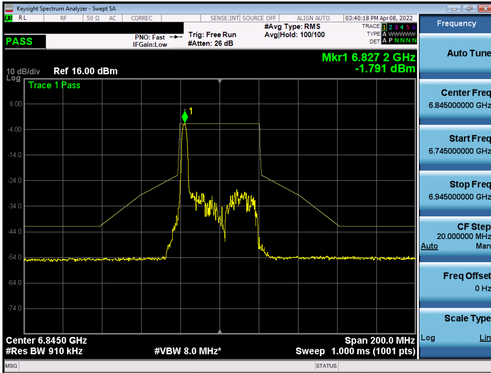
Plot 7-321. In-Band Emission Plot MIMO ANT1 (40MHz BW 802.11ax (26 Tones) (UNII Band 7) – Ch. 179)
