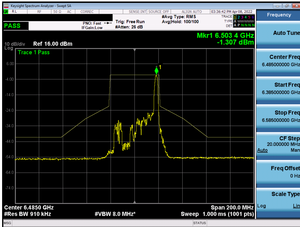
Plot 7-312. In-Band Emission Plot MIMO ANT1 (40MHz BW 802.11ax (26 Tones) (UNII Band 6) – Ch. 107)
