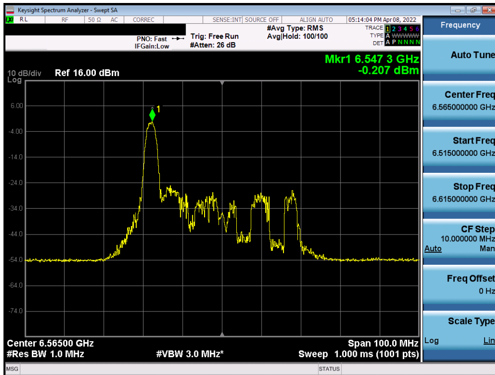
Plot 7-246. Power Spectral Density Plot MIMO ANT2 (40MHz BW 802.11ax (26 Tones) (UNII Band 7) – Ch. 123)
