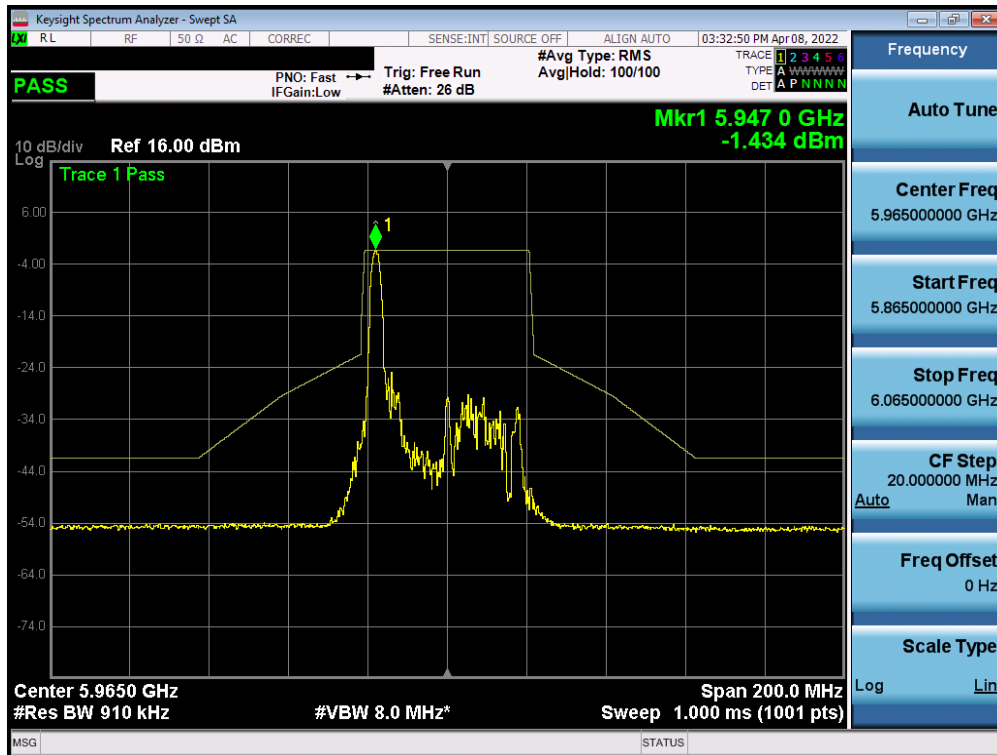
Plot 7-299. In-Band Emission Plot MIMO ANT1 (40MHz BW 802.11ax (26 Tones) (UNII Band 5) – Ch. 3)
