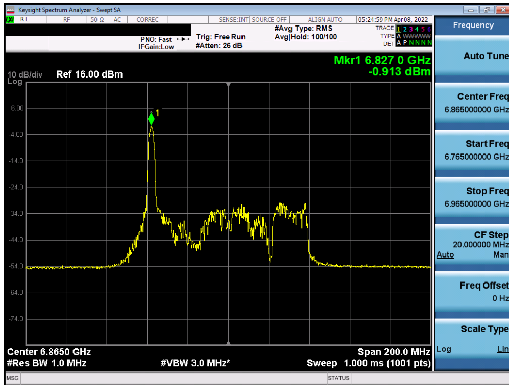
Plot 7-251. Power Spectral Density Plot MIMO ANT2 (80MHz BW 802.11ax (26 Tones) (UNII Band 7) – Ch. 183)
