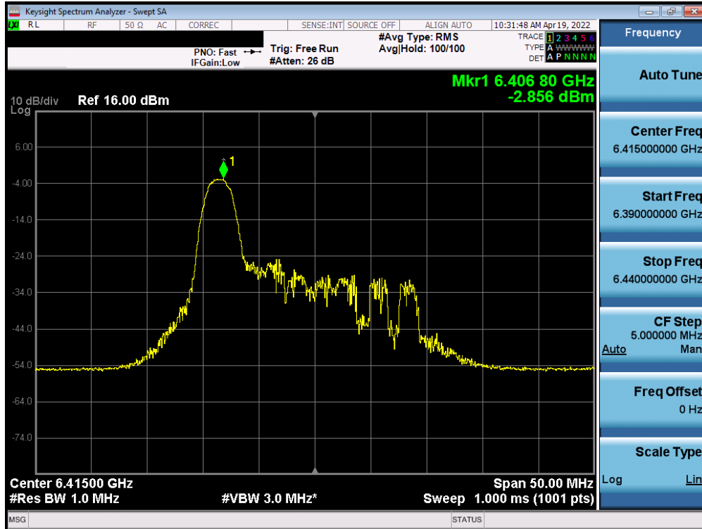
Plot 7-225. Power Spectral Density Plot MIMO ANT2 (20MHz BW 802.11ax (26 Tones) UNII Band 5) – Ch. 93)
