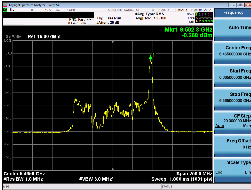
Plot 7-241. Power Spectral Density Plot MIMO ANT2 (80MHz BW 802.11ax (26 Tones) (UNII Band 6) – Ch. 103)
