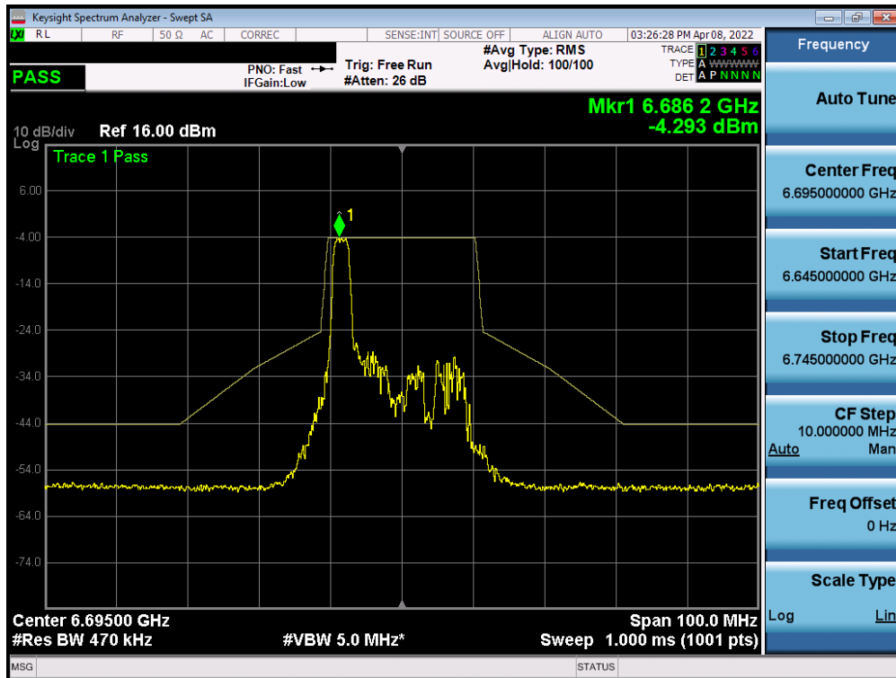
Plot 7-317. In-Band Emission Plot MIMO ANT1 (20MHz BW 802.11ax (26 Tones) (UNII Band 7) – Ch. 149)
