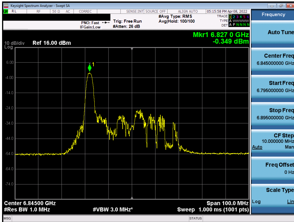
Plot 7-248. Power Spectral Density Plot MIMO ANT2 (40MHz BW 802.11ax (26 Tones) (UNII Band 7) – Ch. 179)
