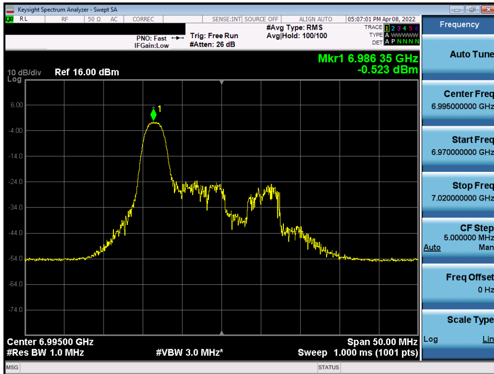
Plot 7-255. Power Spectral Density Plot MIMO ANT2 (20MHz BW 802.11ax (26 Tones) (UNII Band 8) – Ch. 209)
