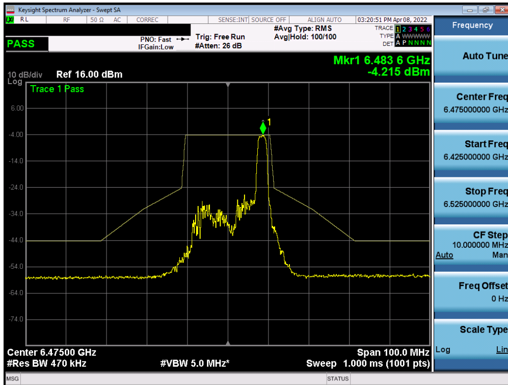
Plot 7-309. In-Band Emission Plot MIMO ANT1 (20MHz BW 802.11ax (26 Tones) (UNII Band 6) – Ch. 105)
