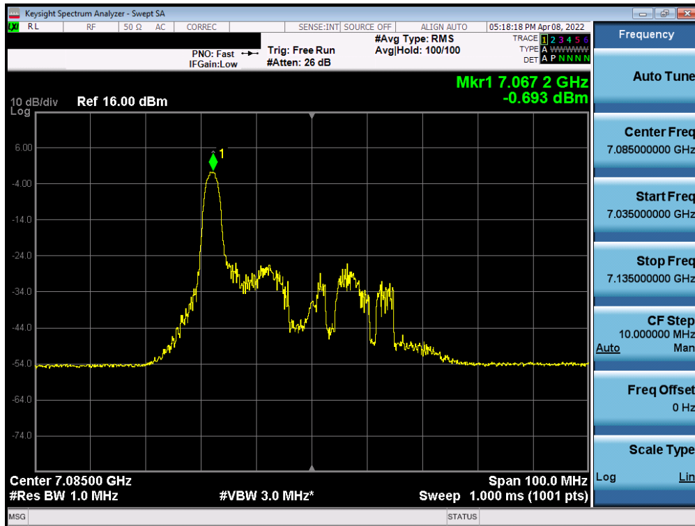
Plot 7-259. Power Spectral Density Plot MIMO ANT2 (40MHz BW 802.11ax (26 Tones) (UNII Band 8) – Ch. 227)
