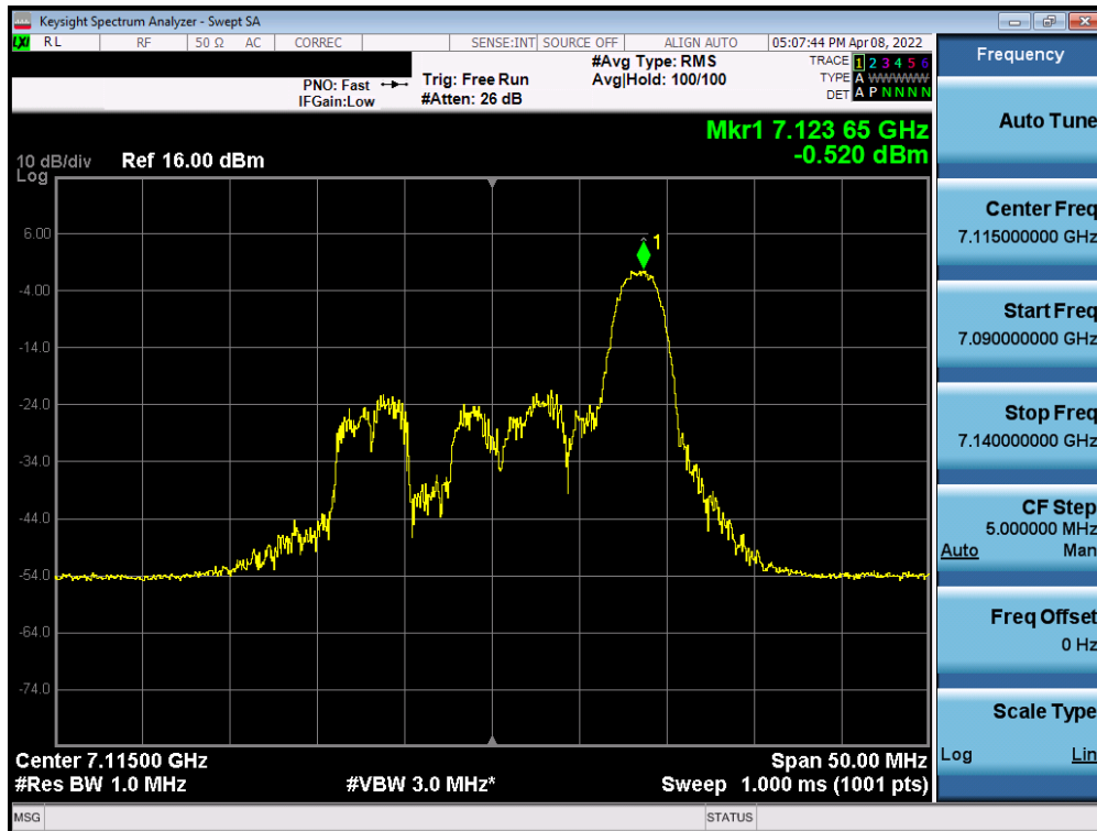
Plot 7-256. Power Spectral Density Plot MIMO ANT2 (20MHz BW 802.11ax (26 Tones) (UNII Band 8) – Ch. 233)
