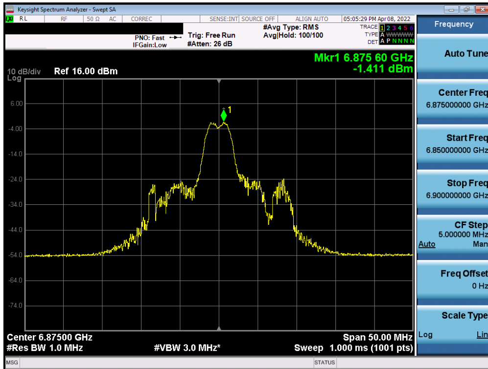
Plot 7-245. Power Spectral Density Plot MIMO ANT2 (20MHz BW 802.11ax (26 Tones) (UNII Band 7) – Ch. 185)
