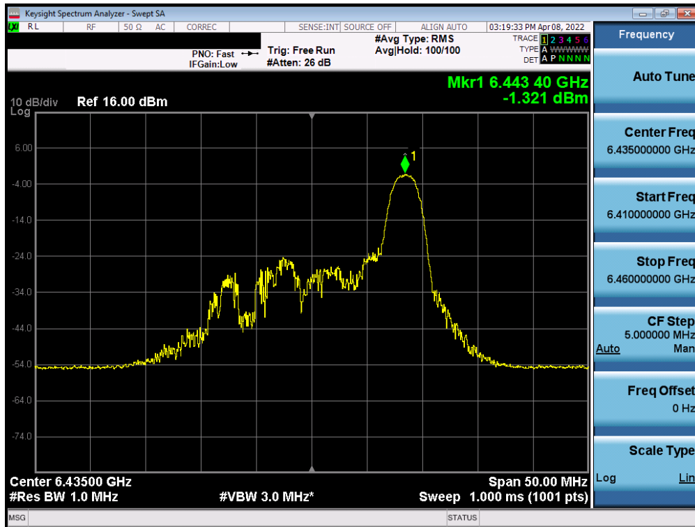
Plot 7-162. Power Spectral Density Plot MIMO ANT1 (20MHz BW 802.11ax (26 Tones) (UNII Band 6) – Ch. 97)
