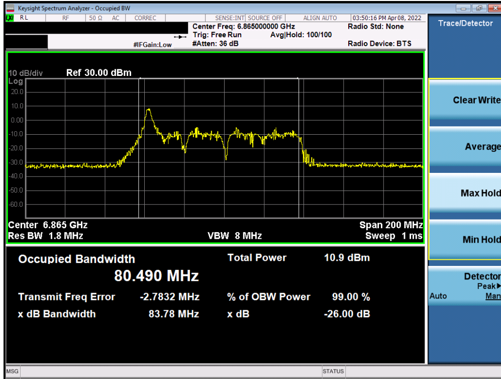
Plot 7-29. Occupied Bandwidth Plot MIMO ANT1 (80MHz BW 802.11ax (26 Tones) (UNII Band 7) – Ch. 183)
