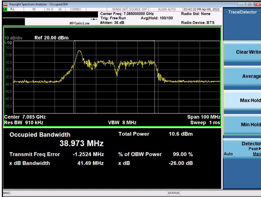
Plot 7-37. Occupied Bandwidth Plot MIMO ANT1 (40MHz BW 802.11ax (26 Tones) (UNII Band 8) – Ch. 227)
