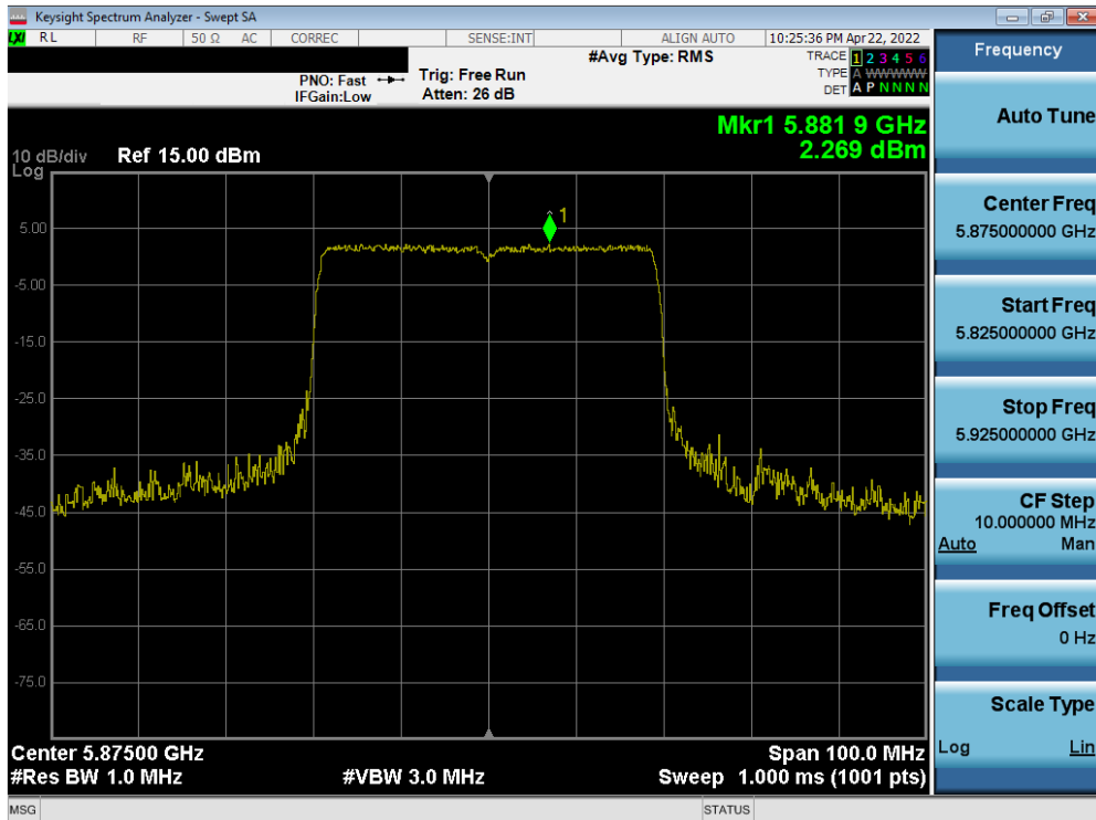
Plot 7-262. Power Spectral Density Plot MIMO ANT1 (40MHz BW 802.11ax – Full Tones (UNII Band 4) – Ch. 175)
