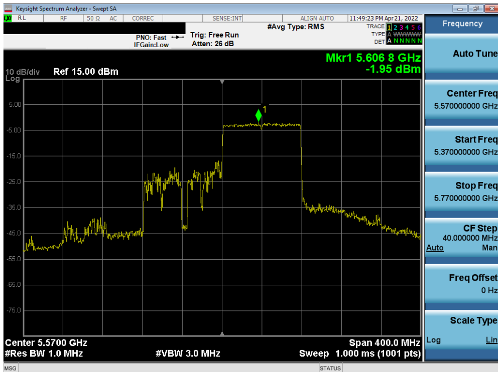
Plot 7-290. Power Spectral Density Plot MIMO ANT2 (160MHz BW (L) 802.11ax – Full Tones (UNII Band 3/4) – Ch. 163)
