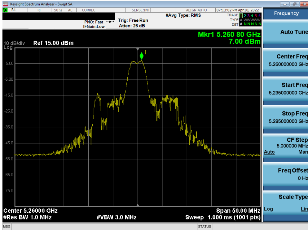
Plot 7-157. Power Spectral Density Plot MIMO ANT1 (20MHz BW 802.11ax – 26 Tones (UNII Band 2A) – Ch. 52)
