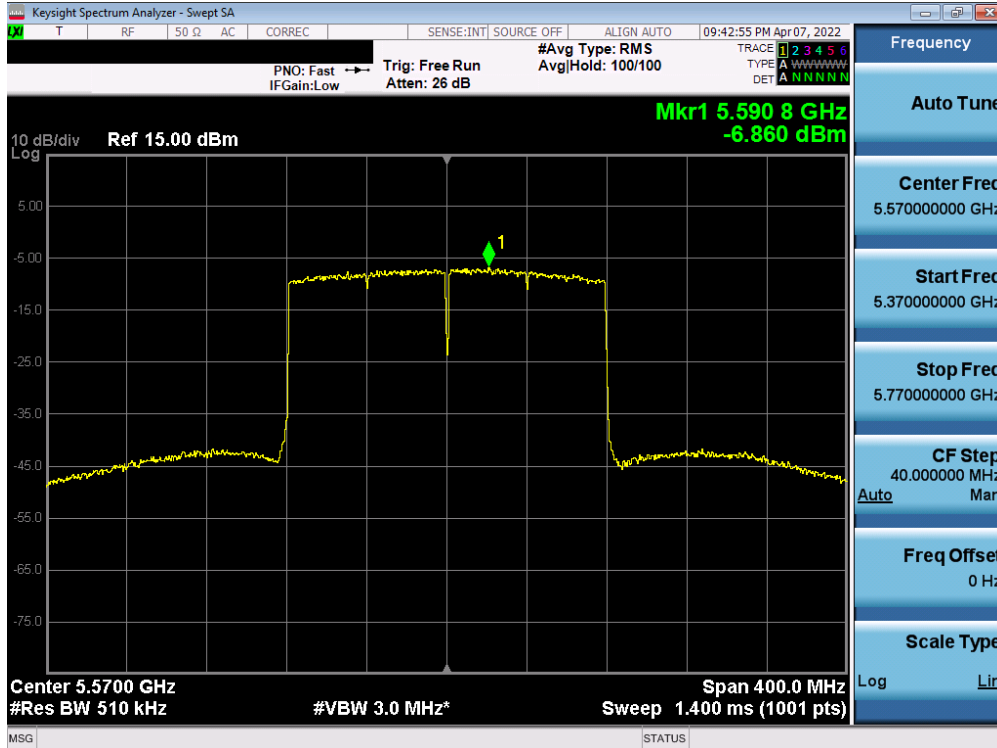
Plot 7-316. Power Spectral Density Plot MIMO ANT2 (160MHz BW 802.11ax (UNII Band 2C) – Ch. 114)
