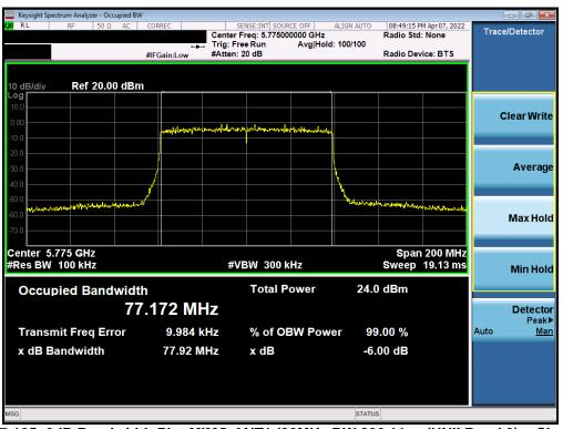
Plot 7-125. 6dB Bandwidth Plot MIMO ANT1 (80MHz BW 802.11ax (UNII Band 3) - Ch. 155)
