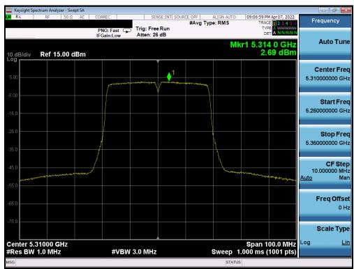
Plot 7-202. Power Spectral Density Plot MIMO ANT1 (40MHz BW 802.11n (UNII Band 2A) - Ch. 62)
