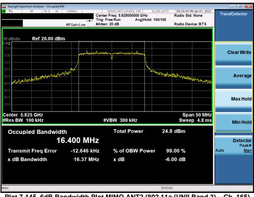
Plot 7-145. 6dB Bandwidth Plot MIMO ANT2 (802.11a (UNII Band 3) - Ch. 165)
