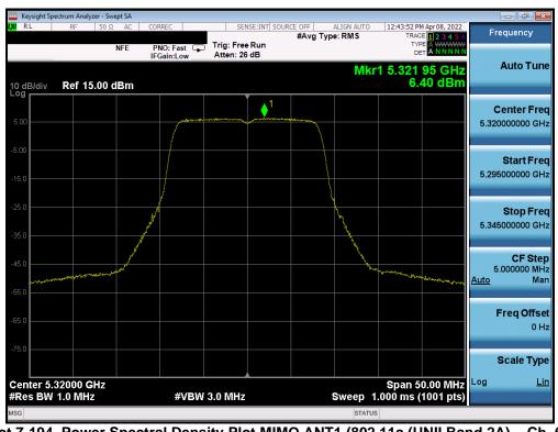
Plot 7-194. Power Spectral Density Plot MIMO ANT1 (802.11a (UNII Band 2A) - Ch. 64)
