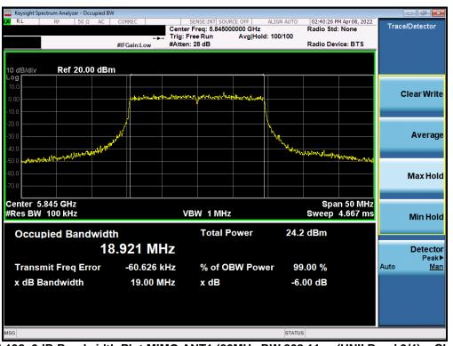
Plot 7-132. 6dB Bandwidth Plot MIMO ANT1 (20MHz BW 802.11ax (UNII Band 3/4) - Ch. 169)
