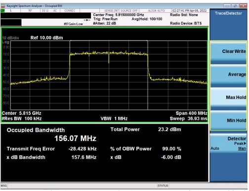
Plot 7-174. 6dB Bandwidth Plot MIMO ANT2 (160MHz BW 802.11ax (UNII Band 3/4) - Ch. 163)
