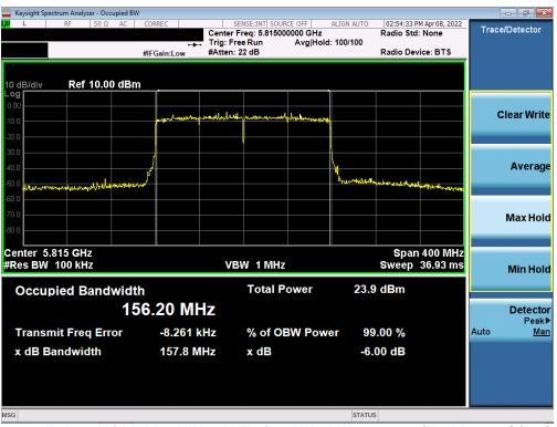
Plot 7-142. 6dB Bandwidth Plot MIMO ANT1 (160MHz BW 802.11ax (UNII Band 3/4) - Ch. 171)
