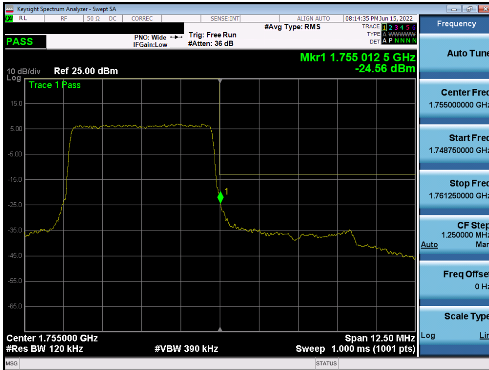
Plot 7-60. Upper Band Edge Plot (LTE Band 4 - 5MHz QPSK – Full RB)
