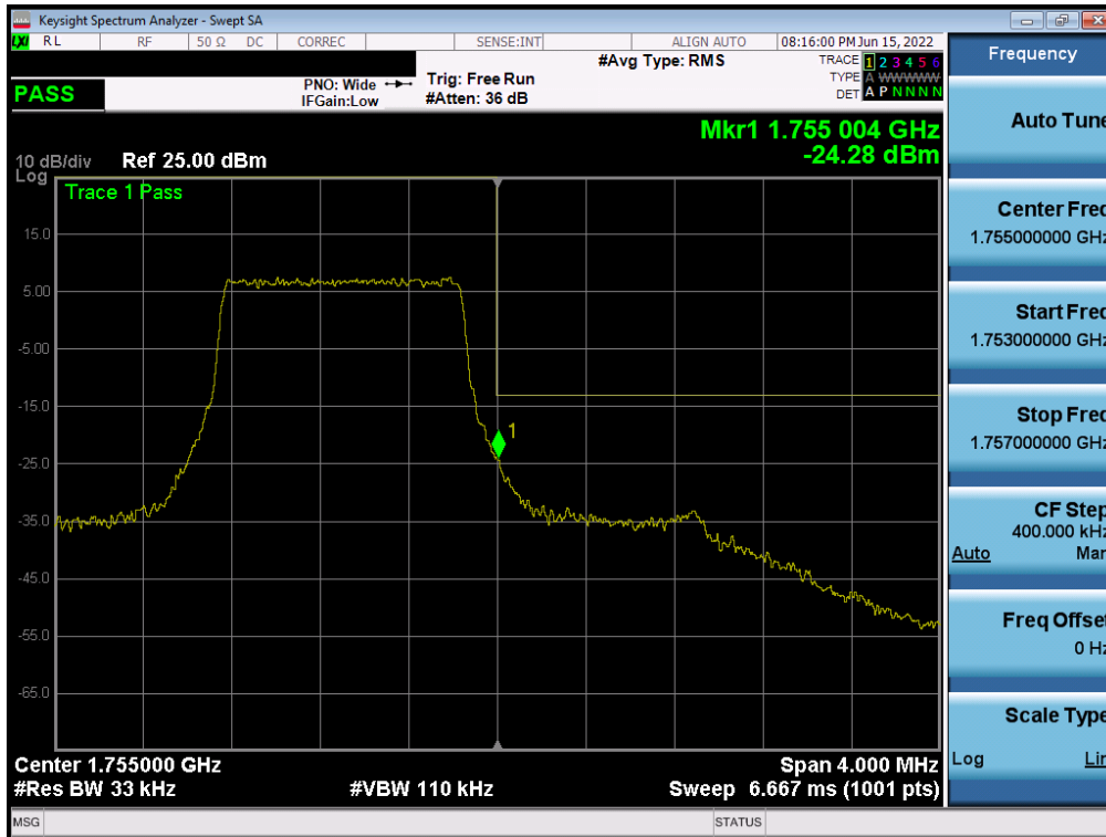
Plot 7-68. Upper Band Edge Plot (LTE Band 4 – 1.4MHz QPSK – Full RB)
