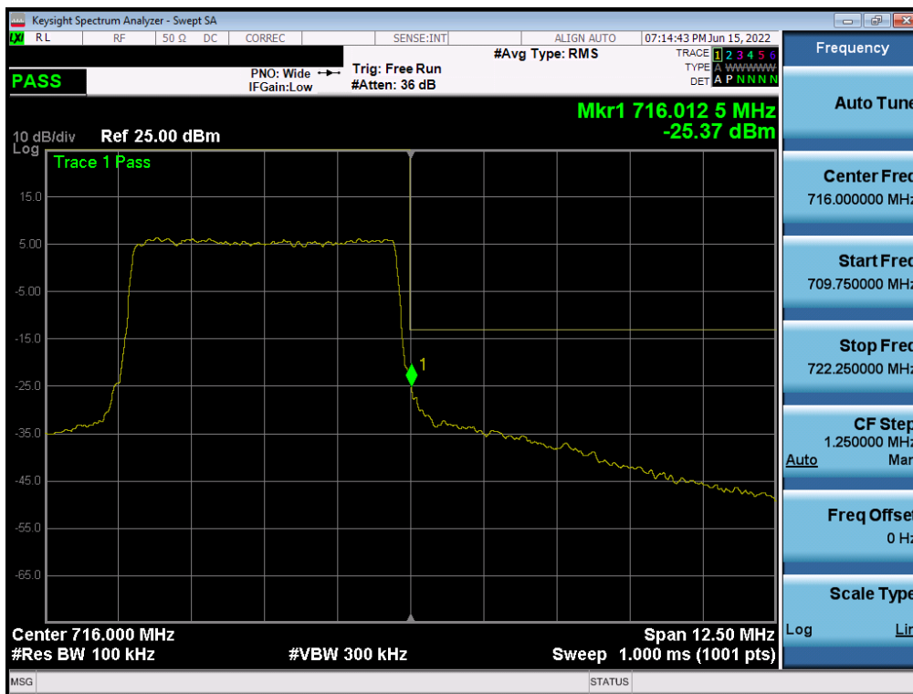
Plot 7-73. Upper Band Edge Plot (LTE Band 12 - 5MHz QPSK – Full RB)
