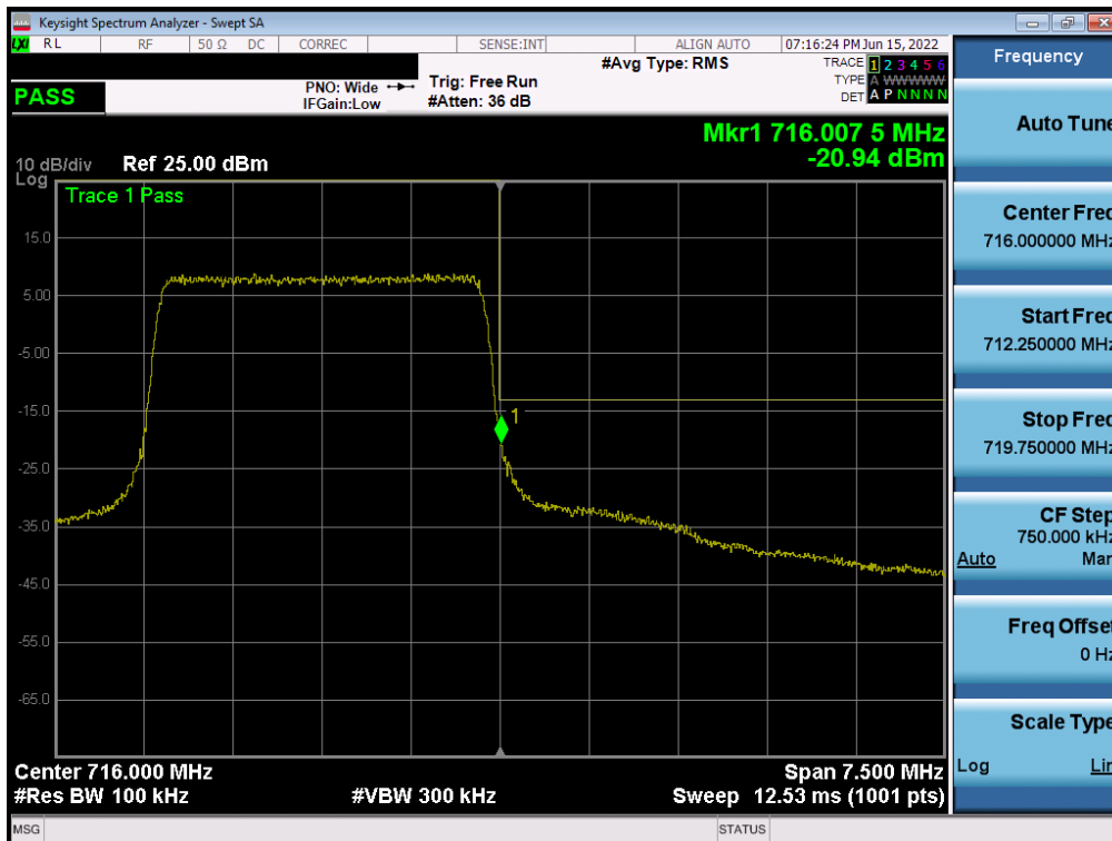
Plot 7-75. Upper Band Edge Plot (LTE Band 12 - 3MHz QPSK – Full RB)
