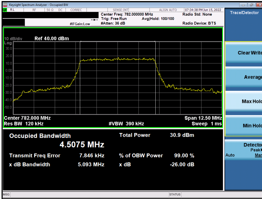
Plot 7-23. Occupied Bandwidth Plot (LTE Band 13 - 5MHz QPSK - Full RB)
