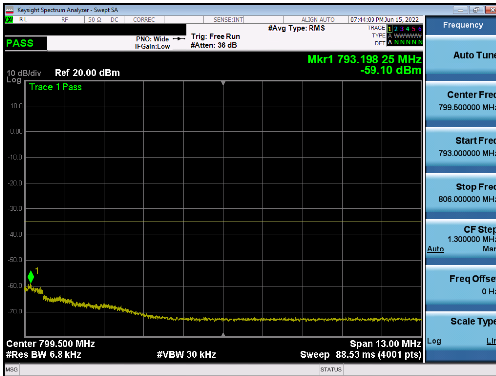
Plot 7-81. Upper Emission Mask Plot (LTE Band 13 - 10MHz QPSK – Full RB)
