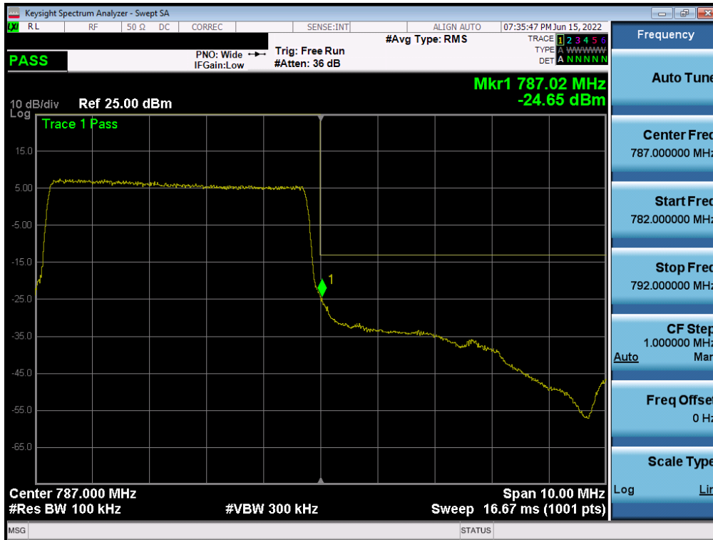
Plot 7-84. Upper Band Edge Plot (LTE Band 13 - 5MHz QPSK – Full RB)
