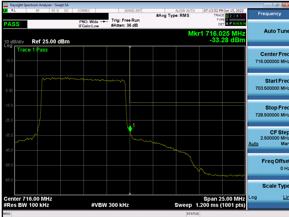
Plot 7-71. Upper Band Edge Plot (LTE Band 12 - 10MHz QPSK – Full RB)
