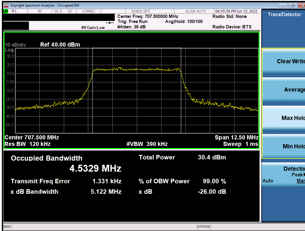
Plot 7-15. Occupied Bandwidth Plot (LTE Band 12 - 5MHz QPSK - Full RB)
