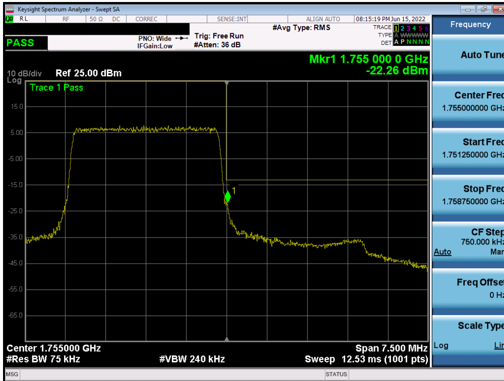
Plot 7-64. Upper Band Edge Plot (LTE Band 4 - 3MHz QPSK – Full RB)
