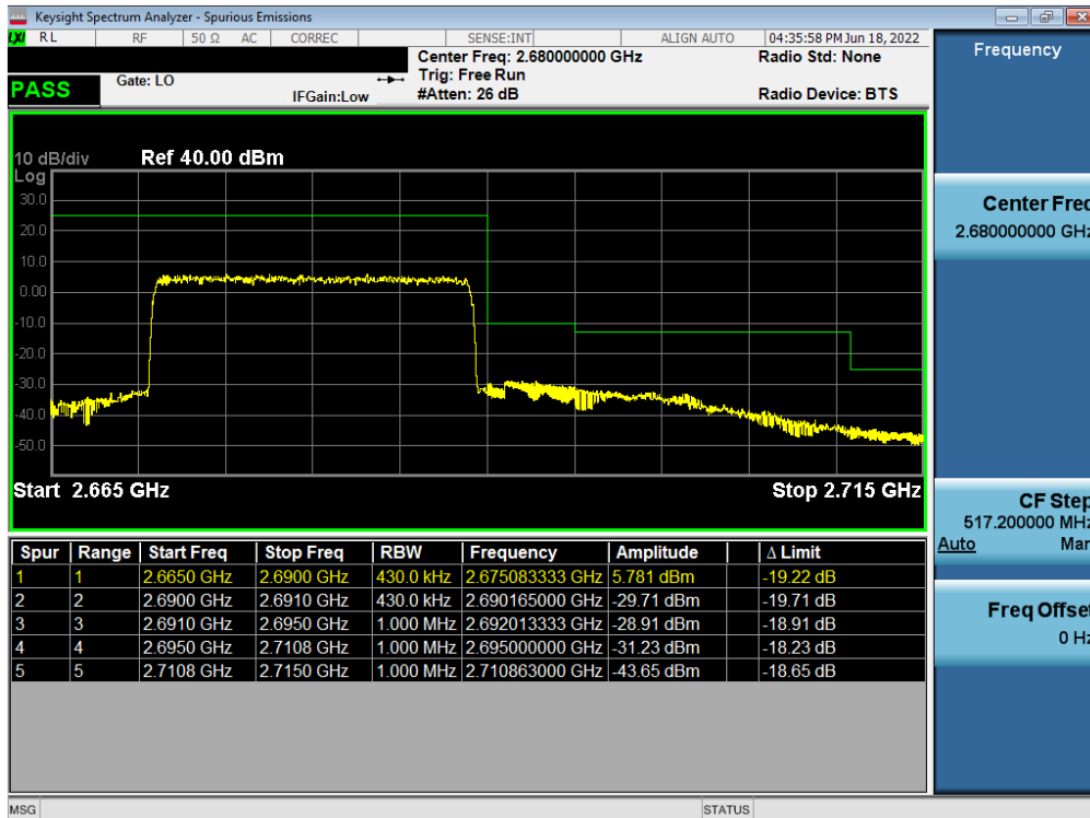
Plot 7-59. Upper ACP Plot (LTE Band 41(PC3) - 20MHz QPSK – Full RB - Ant F)
