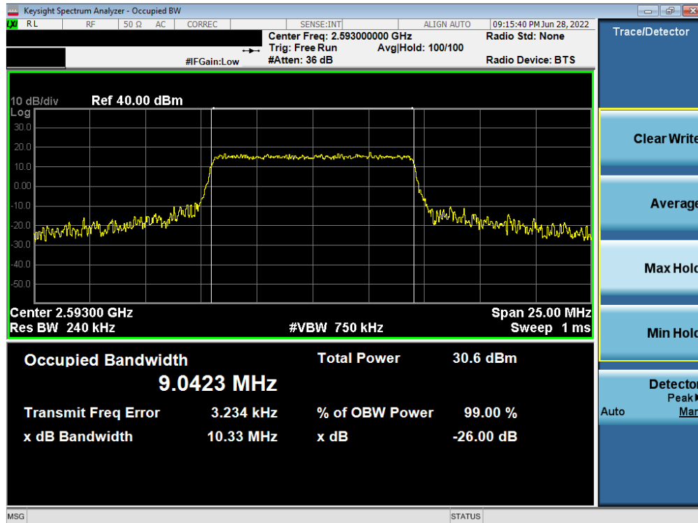
Plot 7-17. Occupied Bandwidth Plot (LTE Band 41(PC3) - 10MHz 16-QAM - Full RB - Ant F)
