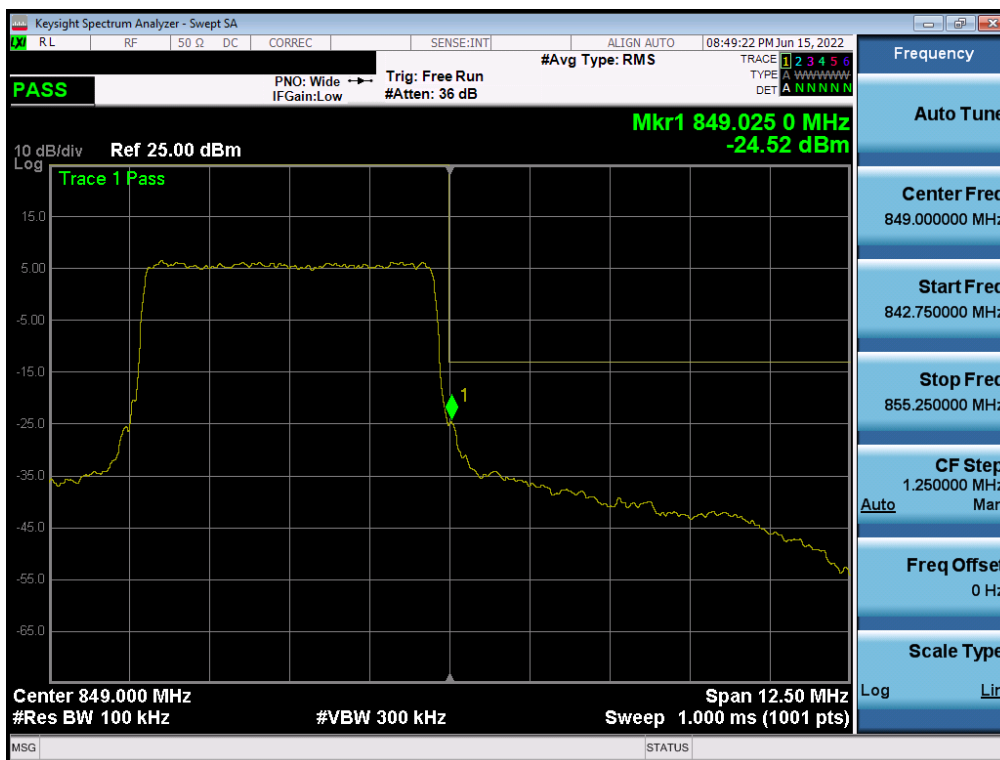
Plot 7-42. Upper Band Edge Plot (LTE Band 5 - 5MHz QPSK – Full RB)
