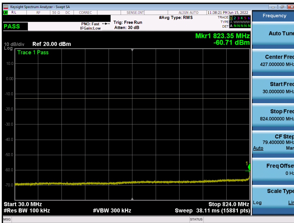
Plot 7-33. Conducted Spurious Plot (WCDMA Ch. 4183)
