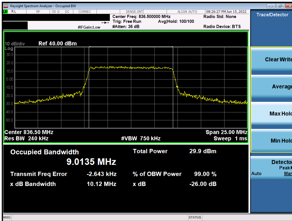
Plot 7-2. Occupied Bandwidth Plot (LTE Band 5 - 10MHz 16-QAM - Full RB)
