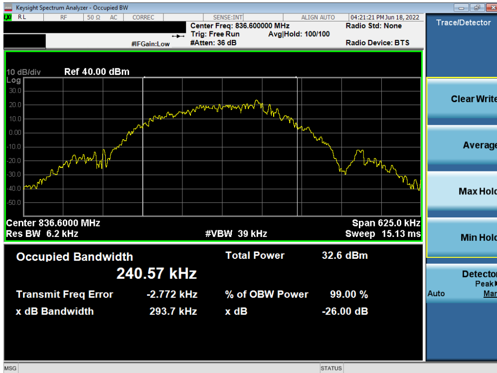
Plot 7-10. Occupied Bandwidth Plot (EDGE, Ch. 190)
