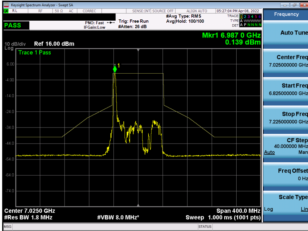
Plot 7-408. In-Band Emission Plot MIMO ANT2 (80MHz BW 802.11ax (26 Tones) (UNII Band 8) – Ch. 215)
