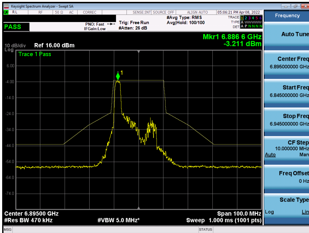
Plot 7-401. In-Band Emission Plot MIMO ANT2 (20MHz BW 802.11ax (26 Tones) (UNII Band 8) – Ch. 189)
