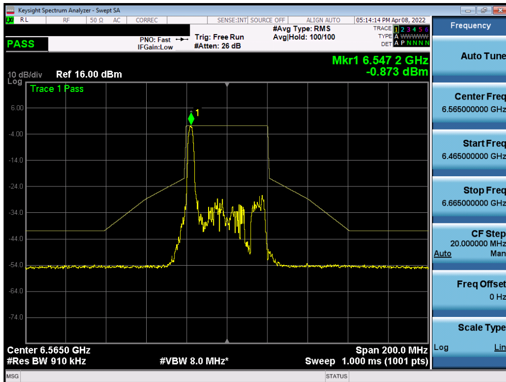
Plot 7-393. In-Band Emission Plot MIMO ANT2 (40MHz BW 802.11ax (26 Tones) (UNII Band 7) – Ch. 123)
