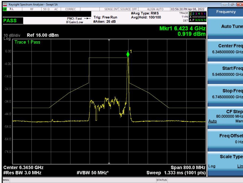
Plot 7-307. In-Band Emission Plot MIMO ANT1 (160MHz BW 802.11ax (26 Tones) (UNII Band 5) – Ch. 79)
