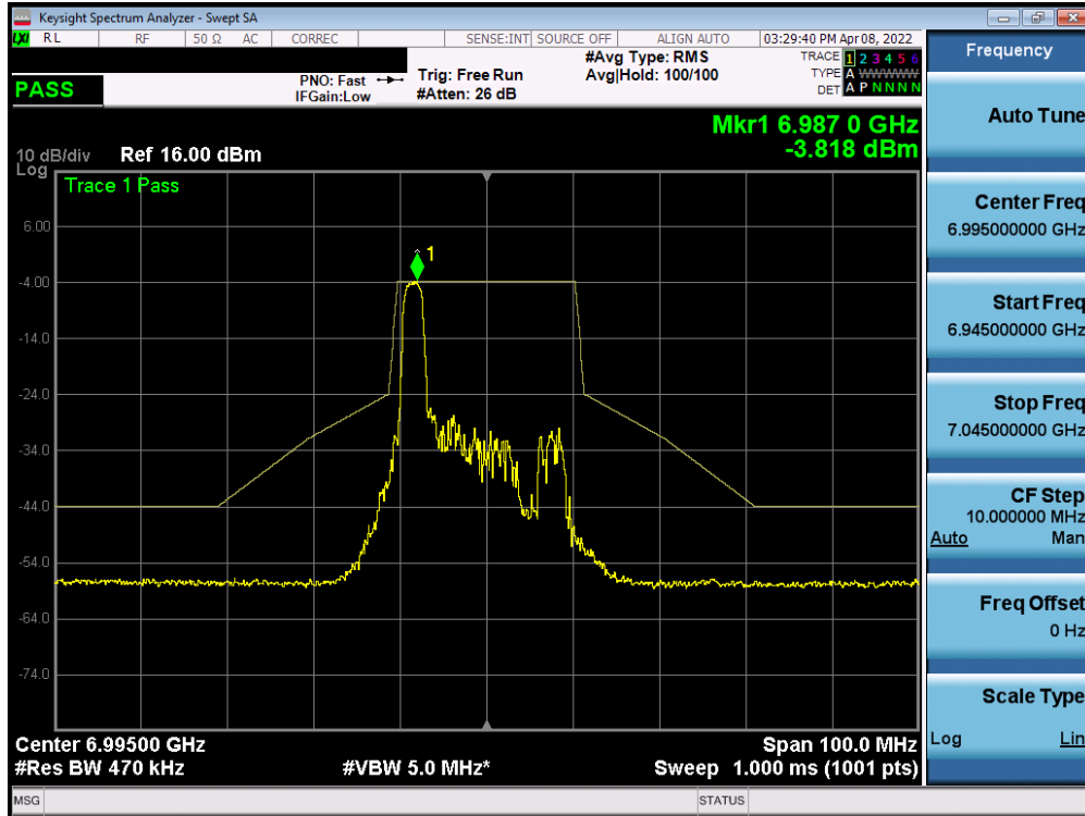
Plot 7-328. In-Band Emission Plot MIMO ANT1 (20MHz BW 802.11ax (26 Tones) (UNII Band 8) – Ch. 209)
