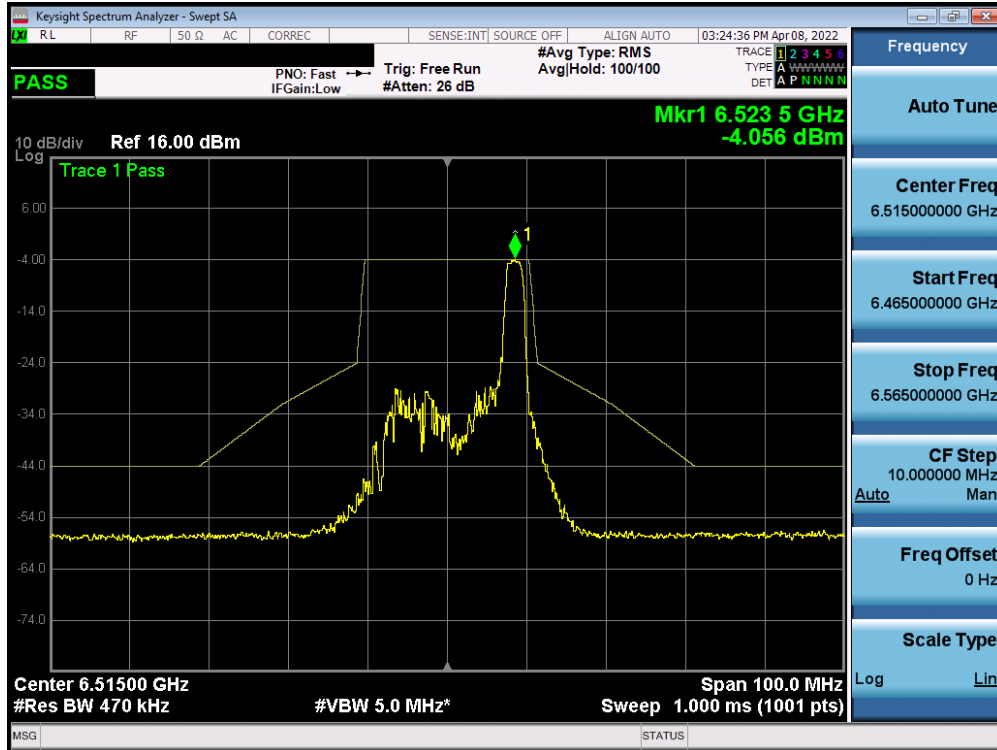
Plot 7-310. In-Band Emission Plot MIMO ANT1 (20MHz BW 802.11ax (26 Tones) (UNII Band 6) – Ch. 113)
