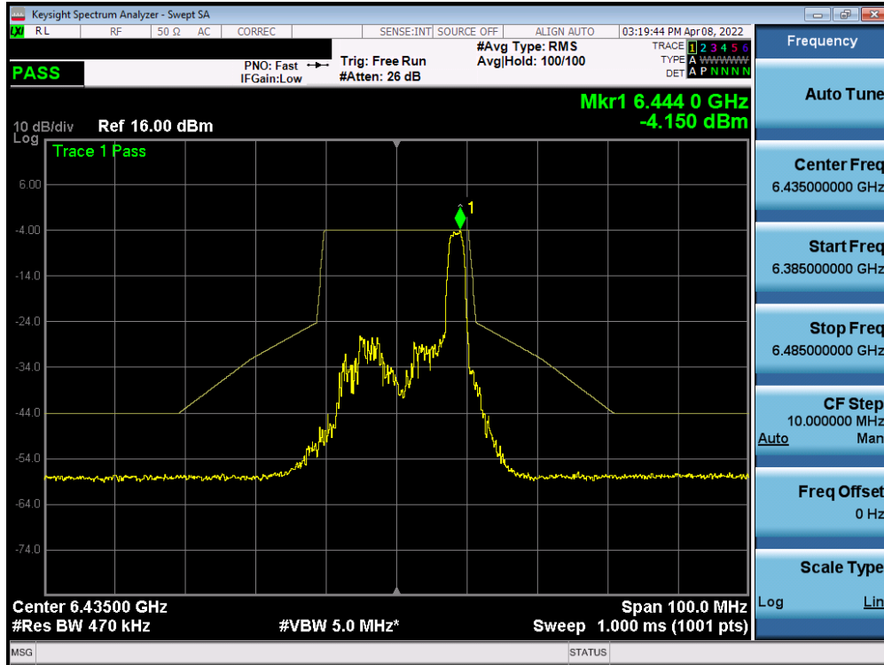
Plot 7-308. In-Band Emission Plot MIMO ANT1 (20MHz BW 802.11ax (26 Tones) (UNII Band 6) – Ch. 97)
