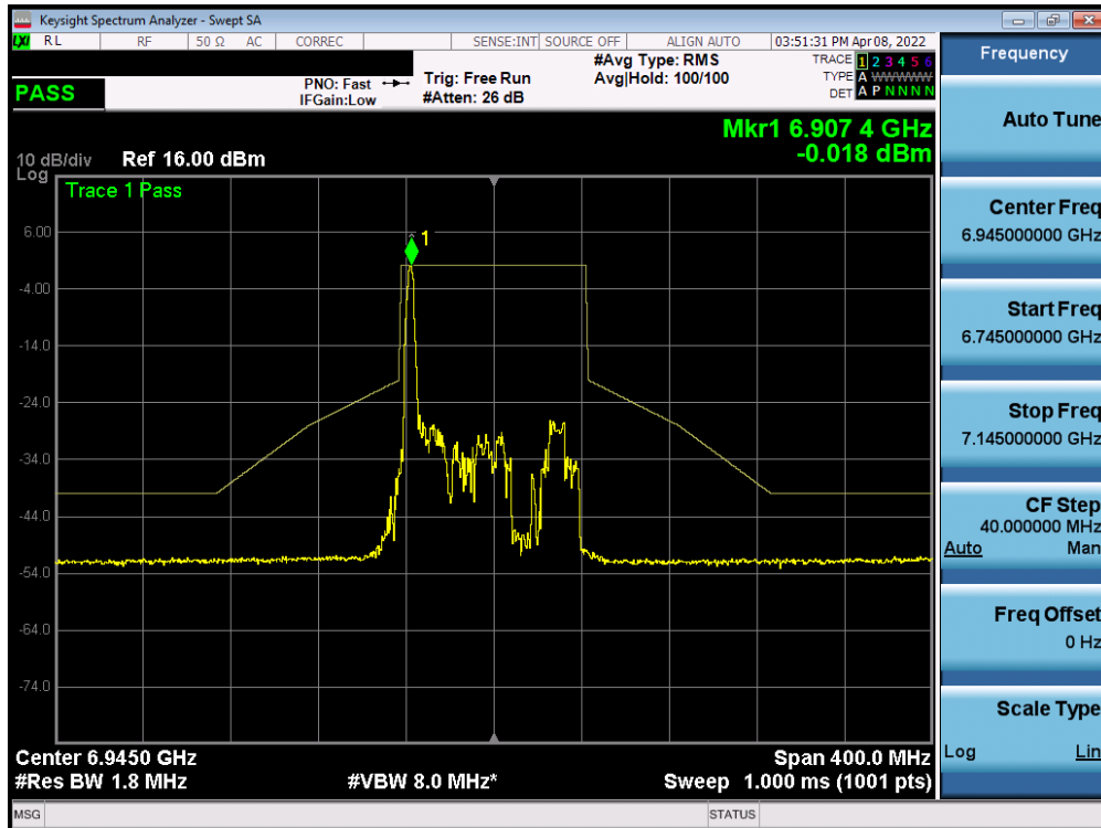
Plot 7-333. In-Band Emission Plot MIMO ANT1 (80MHz BW 802.11ax (26 Tones) (UNII Band 8) – Ch. 199)
