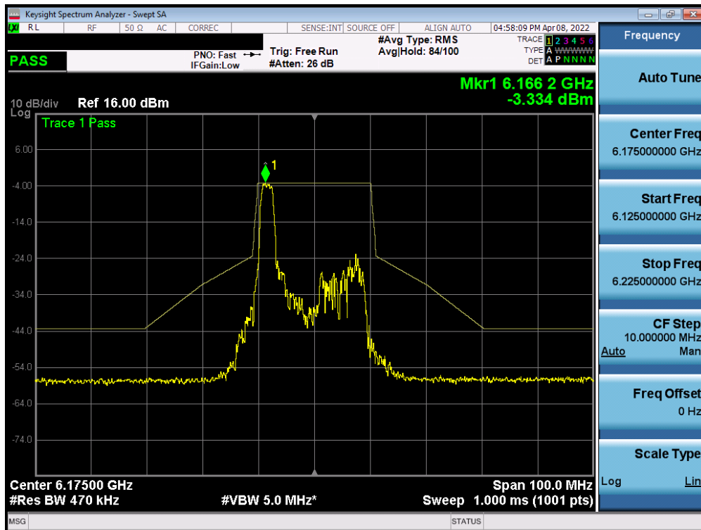
Plot 7-371. In-Band Emission Plot MIMO ANT2 (20MHz BW 802.11ax (26 Tones) (UNII Band 5) – Ch. 45)
