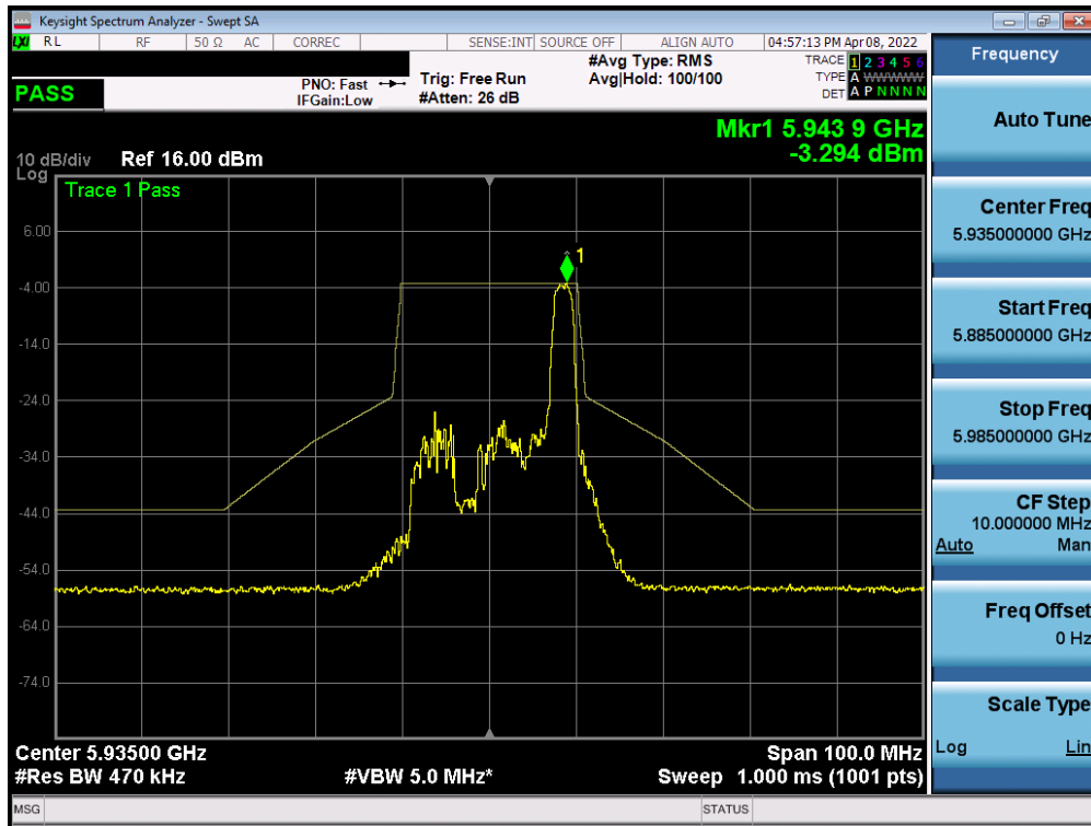
Plot 7-370. In-Band Emission Plot MIMO ANT2 (20MHz BW 802.11ax (26 Tones) UNII Band 5) – Ch. 2)
