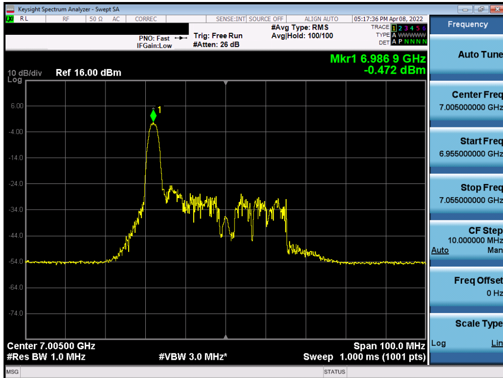
Plot 7-258. Power Spectral Density Plot MIMO ANT2 (40MHz BW 802.11ax (26 Tones) (UNII Band 8) – Ch. 211)
