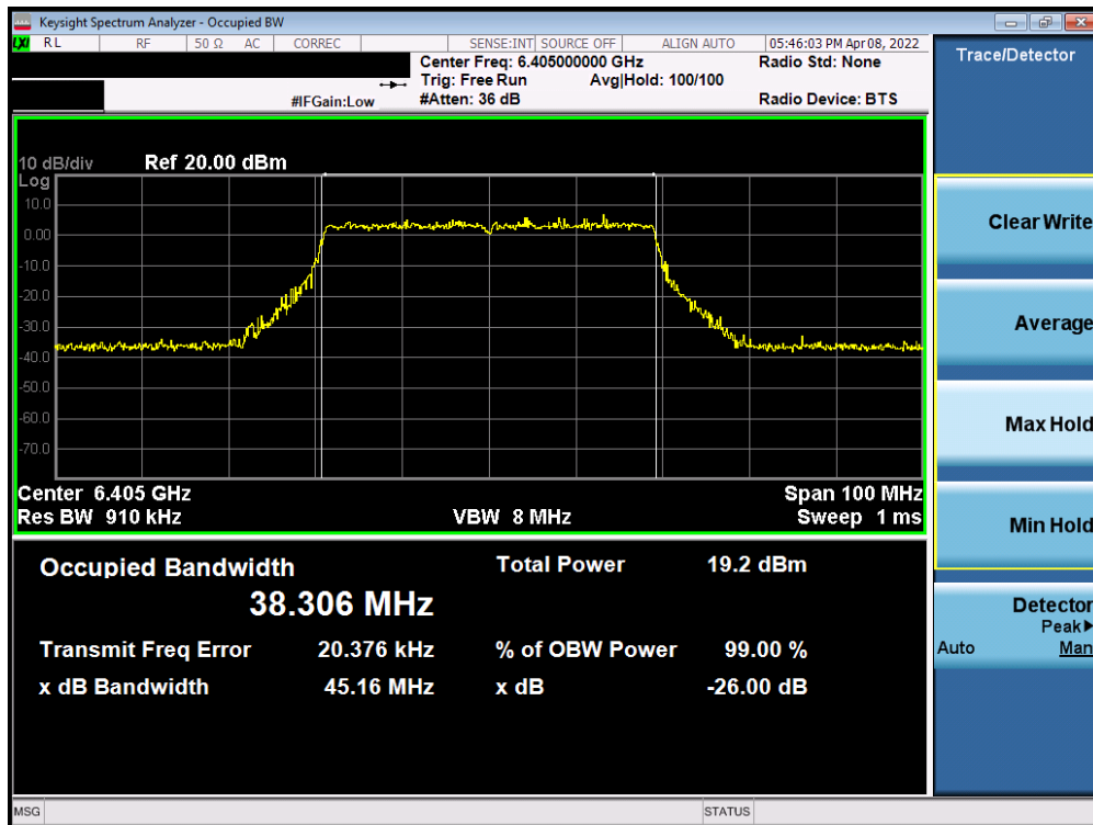
Plot 7-120. Occupied Bandwidth Plot MIMO ANT2 (40MHz BW 802.11ax (Full Tone) (UNII Band 5) – Ch. 91)
