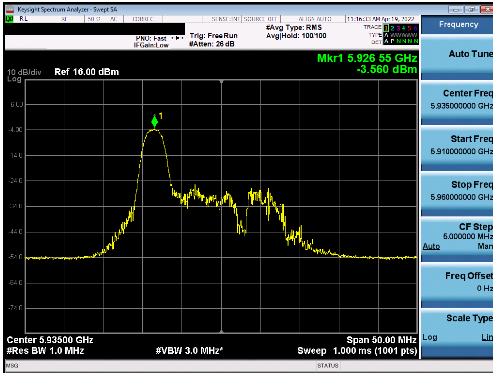
Plot 7-150. Power Spectral Density Plot MIMO ANT1 (20MHz BW 802.11ax (26 Tones) UNII Band 5) – Ch. 2
