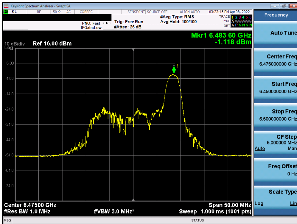
Plot 7-163. Power Spectral Density Plot MIMO ANT1 (20MHz BW 802.11ax (26 Tones) (UNII Band 6) – Ch. 105)
