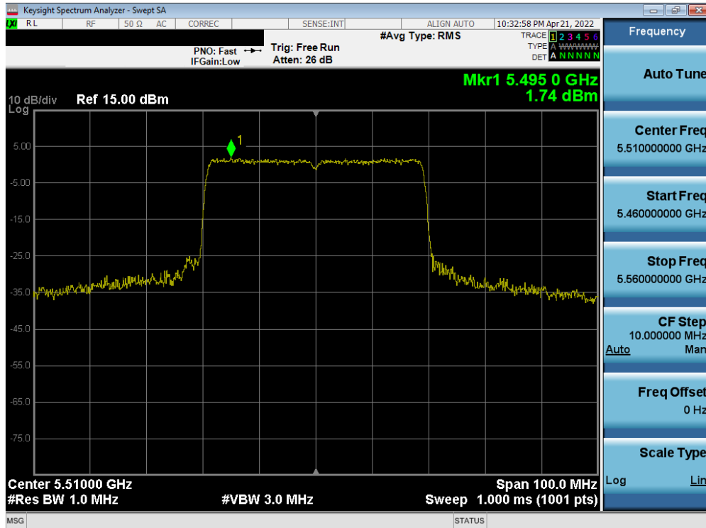
Plot 7-283. Power Spectral Density Plot MIMO ANT2 (40MHz BW 802.11ax – Full Tones (UNII Band 2C) – Ch. 102)
