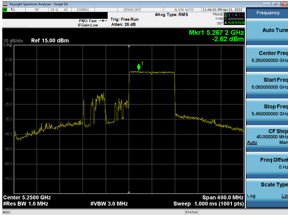
Plot 7-273. Power Spectral Density Plot MIMO ANT2 (160MHz (U) BW 802.11ax – Full Tones (UNII Band 1/2A) – Ch. 50)
