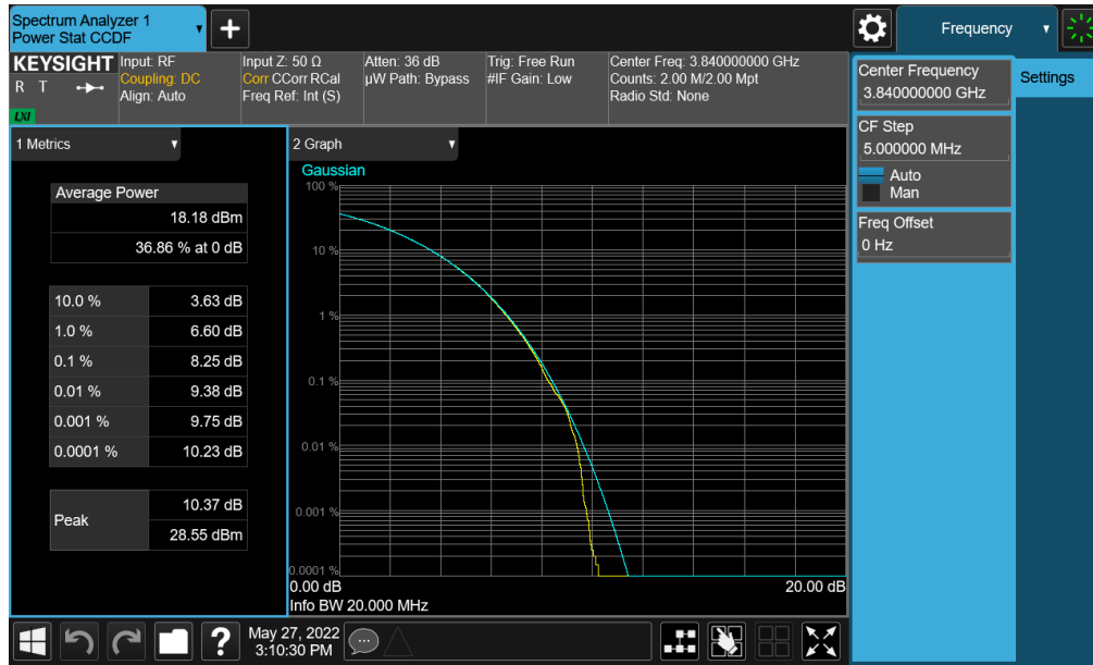
Plot 7-348. PAR Plot (NR Band n77 (C-Band) - 20MHz CP-OFDM 256-QAM - Full RB - Ant E)
