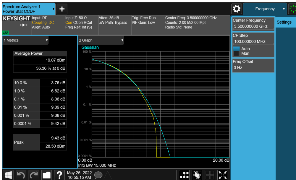
Plot 7-390. PAR Plot (NR Band n77 (DoD) - 15MHz CP-OFDM 256-QAM - Full RB - Ant F)
