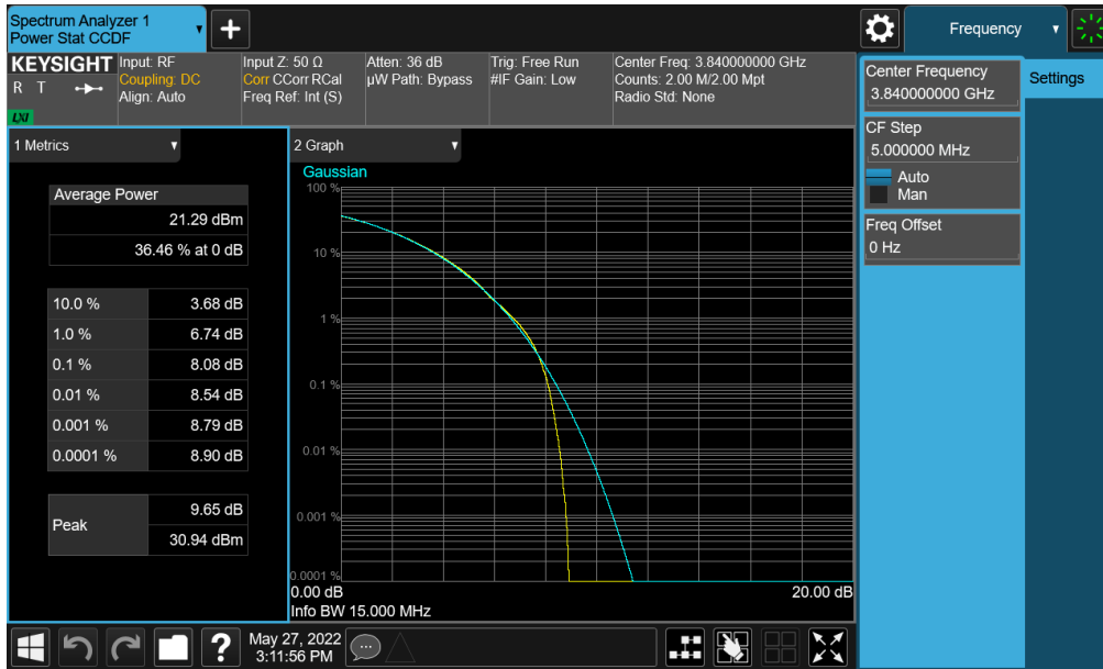
Plot 7-350. PAR Plot (NR Band n77 (C-Band) - 15MHz CP-OFDM QPSK - Full RB - Ant E)
