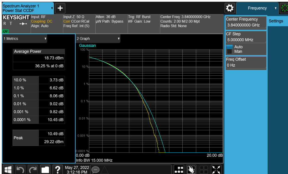
Plot 7-351. PAR Plot (NR Band n77 (C-Band) - 15MHz CP-OFDM 256-QAM - Full RB - Ant E)
