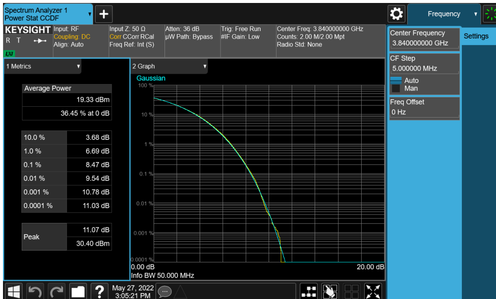
Plot 7-339. PAR Plot (NR Band n77 (C-Band) - 50MHz CP-OFDM 256-QAM - Full RB - Ant E)
