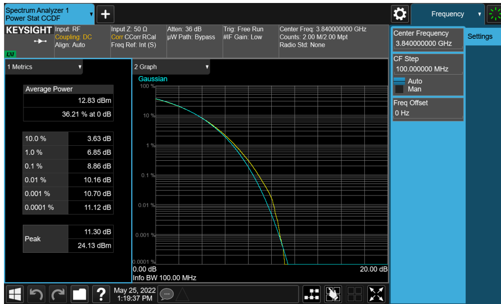
Plot 7-360. PAR Plot (NR Band n77 (C-Band) - 100MHz CP-OFDM 256-QAM - Full RB - Ant D)
