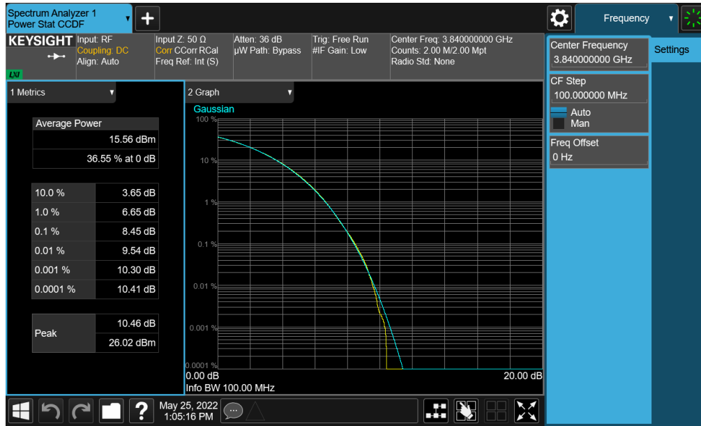
Plot 7-357. PAR Plot (NR Band n77 (C-Band) - 100MHz CP-OFDM 256-QAM - Full RB - Ant G)
