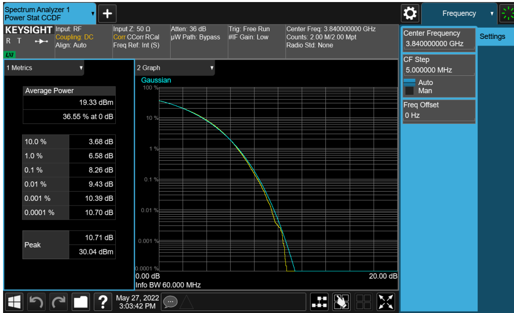
Plot 7-336. PAR Plot (NR Band n77 (C-Band) - 60MHz CP-OFDM 256-QAM - Full RB - Ant E)
