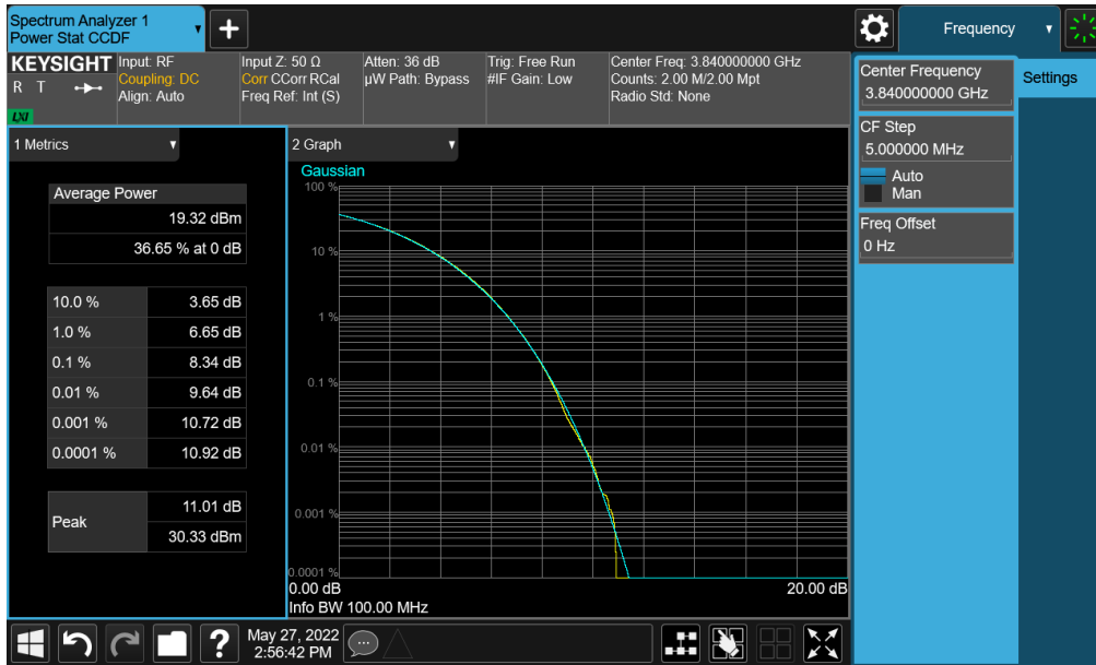
Plot 7-324. PAR Plot (NR Band n77 (C-Band) - 100MHz CP-OFDM 256-QAM - Full RB - Ant E)
