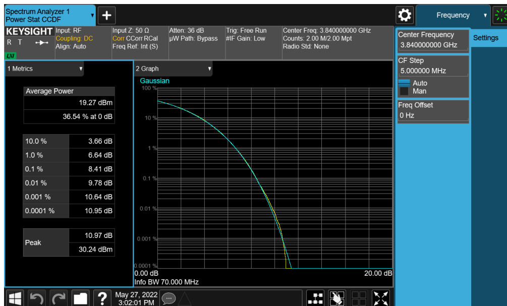
Plot 7-333. PAR Plot (NR Band n77 (C-Band) - 70MHz CP-OFDM 256-QAM - Full RB - Ant E)
