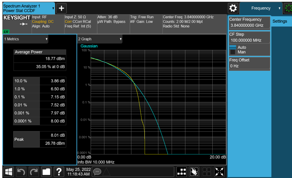
Plot 7-321. PAR Plot (NR Band n77 (C-Band) - 10MHz CP-OFDM 256-QAM - Full RB - Ant F)
