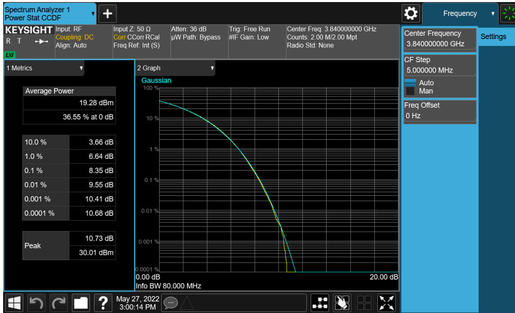
Plot 7-330. PAR Plot (NR Band n77 (C-Band) - 80MHz CP-OFDM 256-QAM - Full RB - Ant E)
