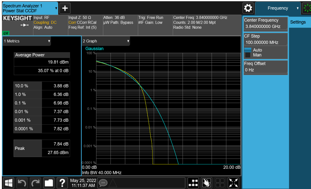
Plot 7-309. PAR Plot (NR Band n77 (C-Band) - 40MHz CP-OFDM 256-QAM - Full RB - Ant F)
