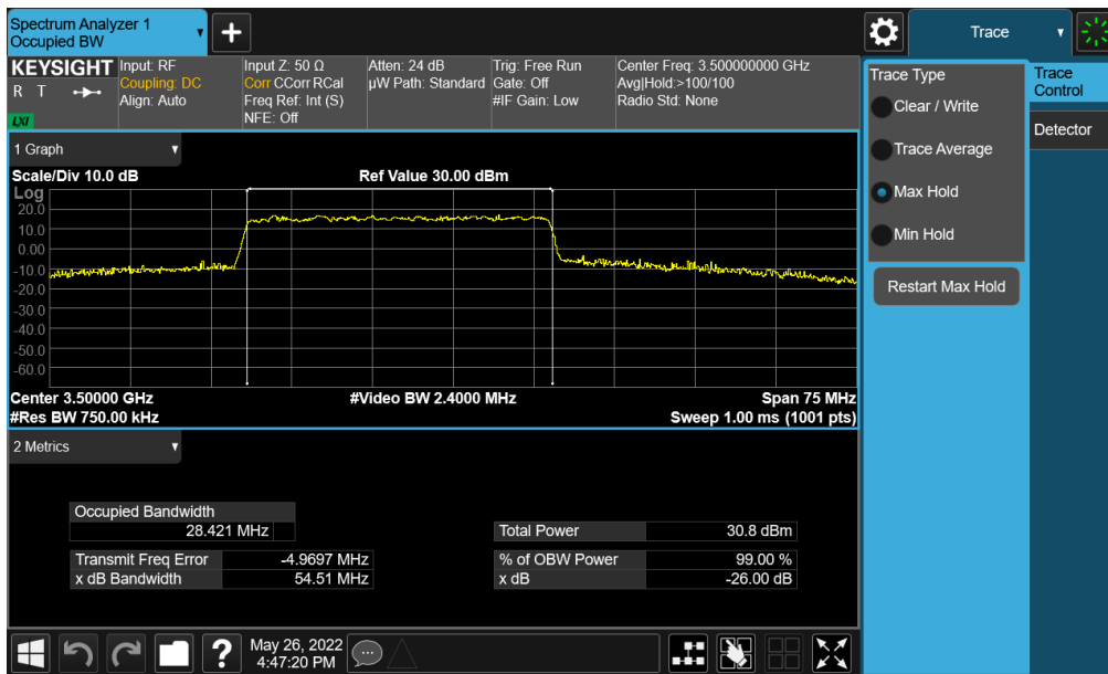
Plot 7-129. Occupied Bandwidth Plot (NR Band n77 (DoD) - 30MHz 16-QAM - Full RB - Ant E)
