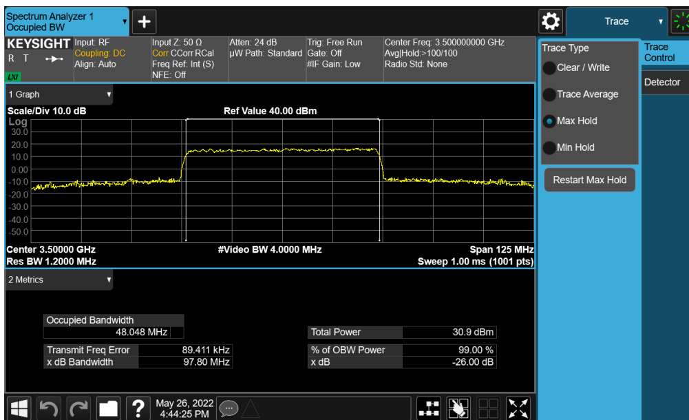
Plot 7-123. Occupied Bandwidth Plot (NR Band n77 (DoD) - 50MHz 16-QAM - Full RB - Ant E)
