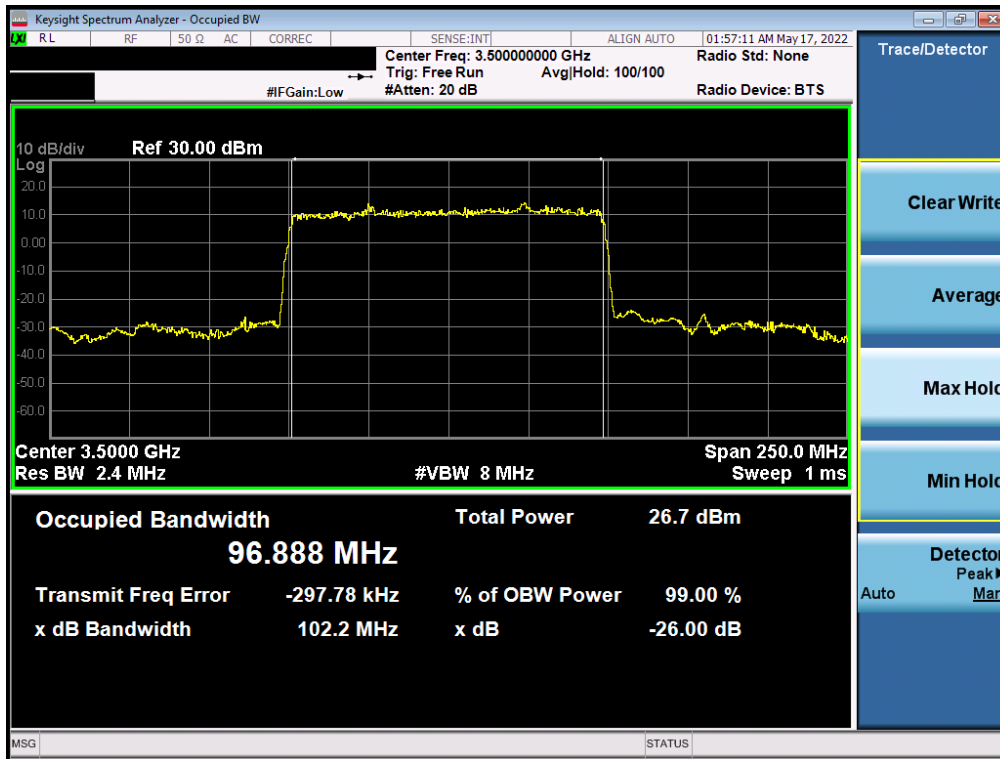
Plot 7-142. Occupied Bandwidth Plot (NR Band n77 (DoD) - 100MHz \pi/2 BPSK - Full RB - Ant D)
