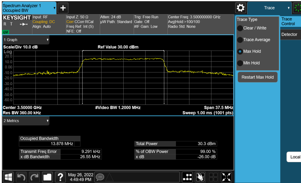
Plot 7-134. Occupied Bandwidth Plot (NR Band n77 (DoD) - 15MHz QPSK - Full RB - Ant E)
