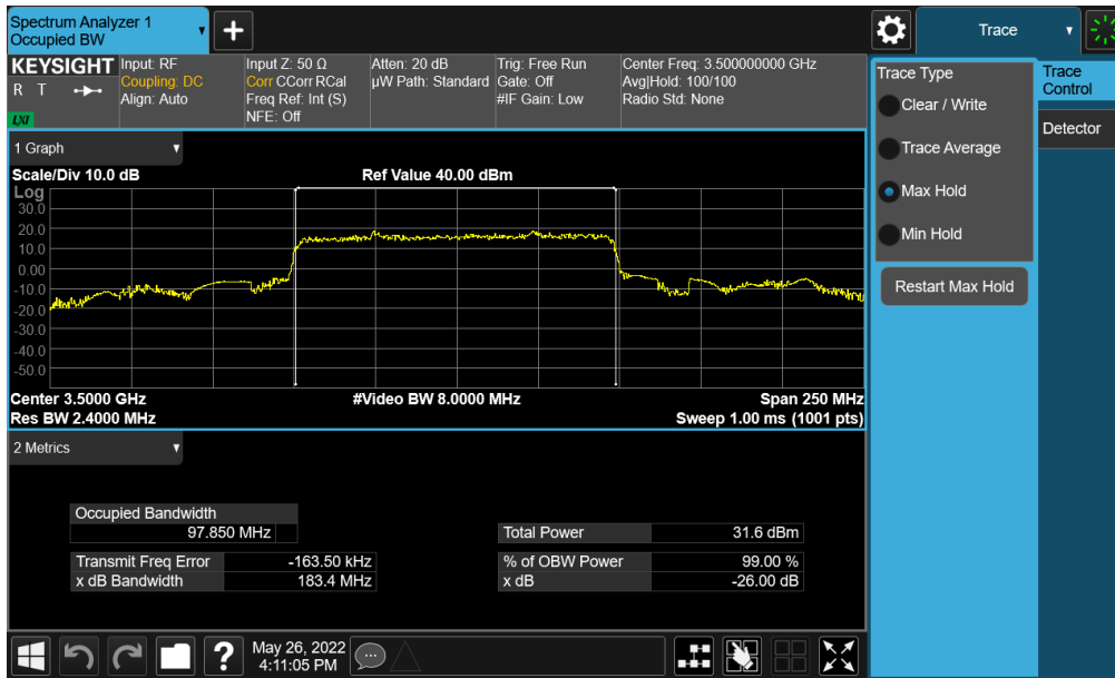
Plot 7-106. Occupied Bandwidth Plot (NR Band n77 (DoD) - 100MHz \pi/2 BPSK - Full RB - Ant E)
