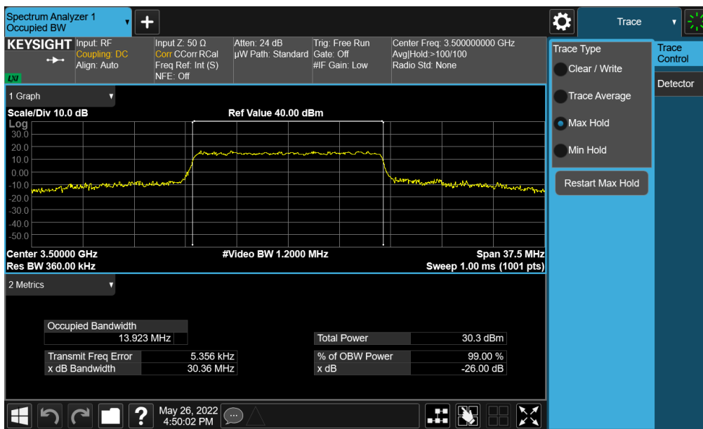
Plot 7-135. Occupied Bandwidth Plot (NR Band n77 (DoD) - 15MHz 16-QAM - Full RB - Ant E)
