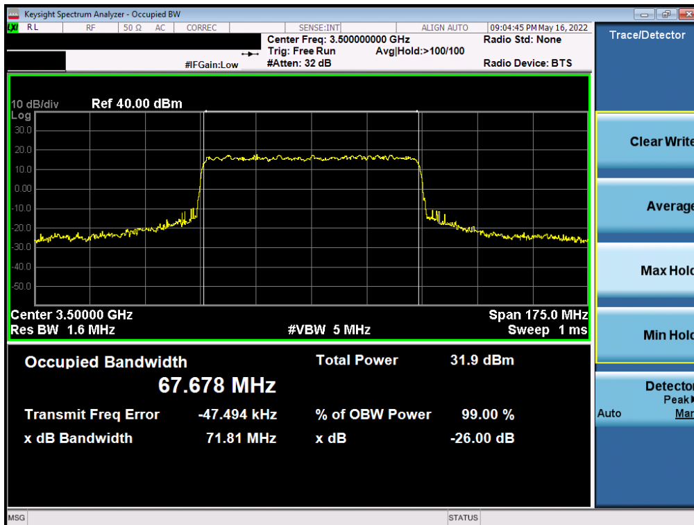
Plot 7-84. Occupied Bandwidth Plot (NR Band n77 (DoD) - 70MHz 16-QAM - Full RB - Ant F)
