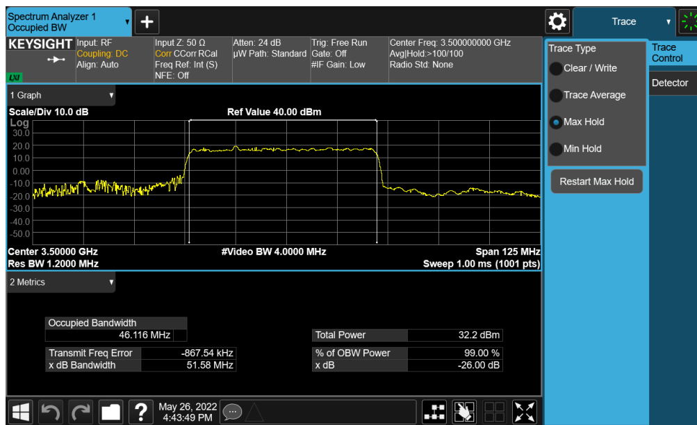
Plot 7-121. Occupied Bandwidth Plot (NR Band n77 (DoD) - 50MHz \pi/2 BPSK - Full RB - Ant E)
