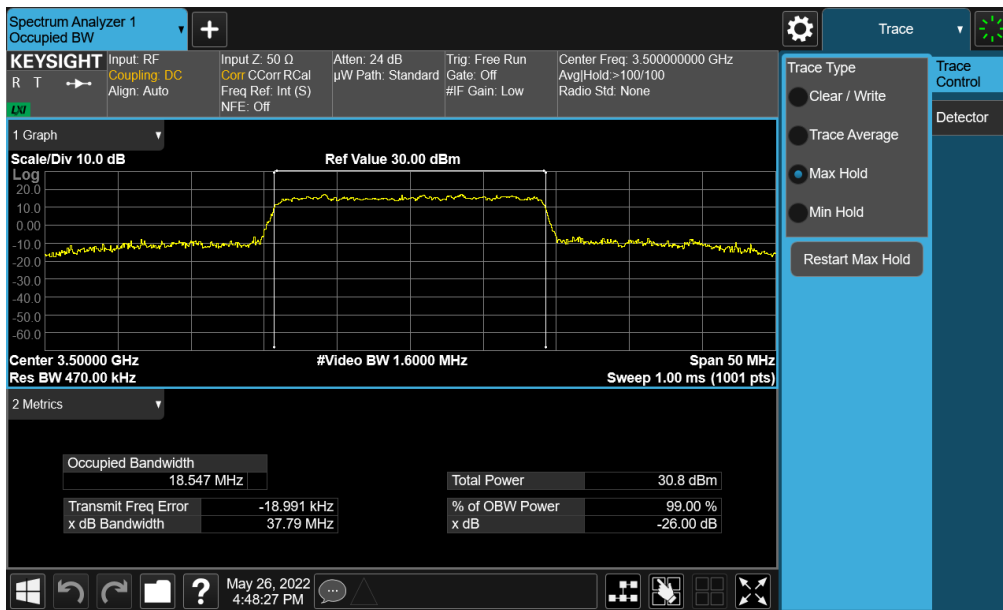
Plot 7-131. Occupied Bandwidth Plot (NR Band n77 (DoD) - 20MHz QPSK - Full RB - Ant E)
