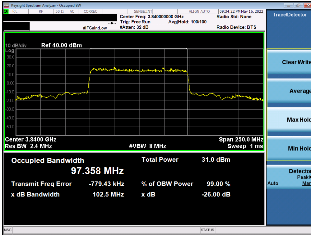
Plot 7-1. Occupied Bandwidth Plot (NR Band n77 (C-Band) - 100MHz \pi/2 BPSK - Full RB - Ant F)
