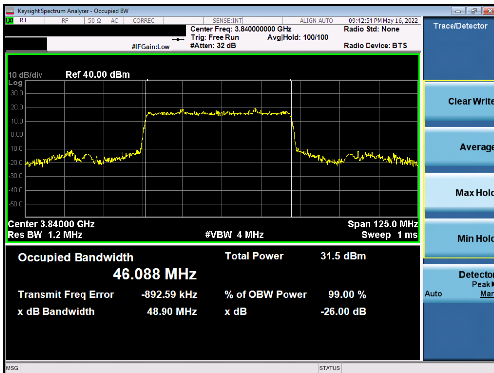
Plot 7-16. Occupied Bandwidth Plot (NR Band n77 (C-Band) - 50MHz \pi/2 BPSK - Full RB - Ant F)
