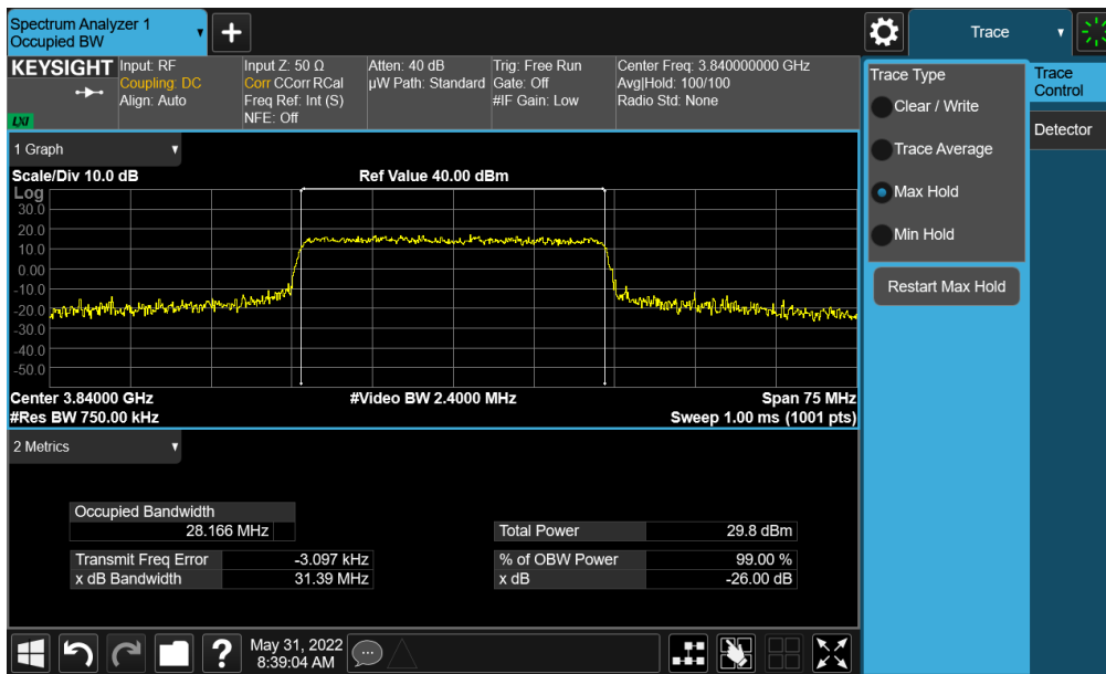
Plot 7-57. Occupied Bandwidth Plot (NR Band n77 (C-Band) - 30MHz 16-QAM - Full RB - Ant E)
