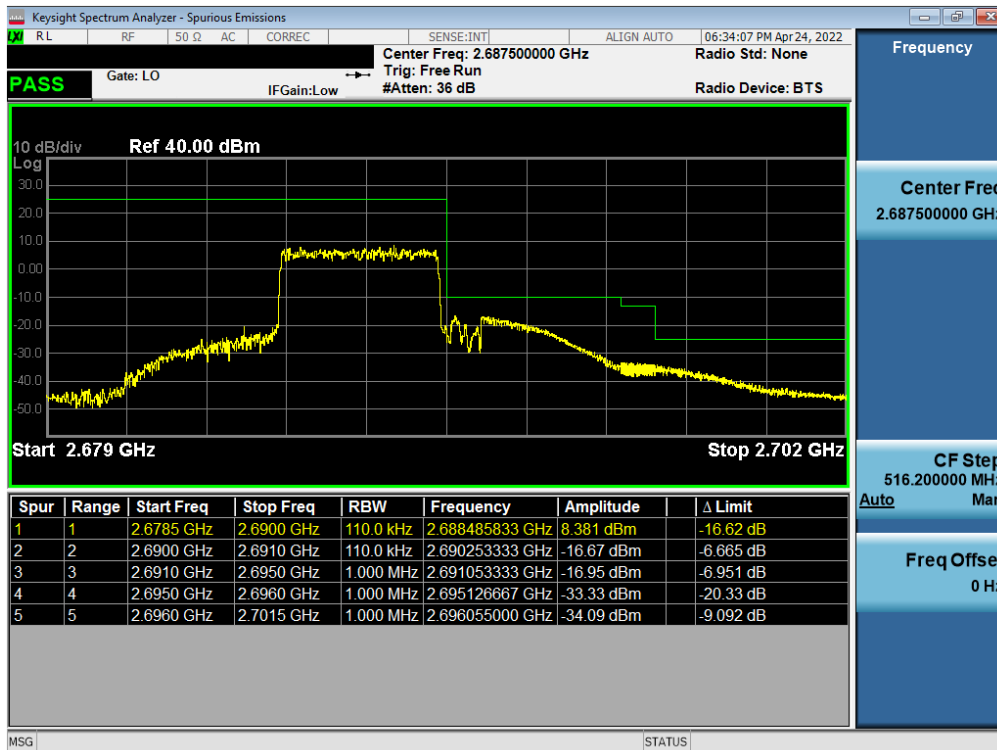
Plot 7-94. Upper ACP Plot (LTE Band 41(PC2) - 5MHz QPSK - Full RB - Ant F)
