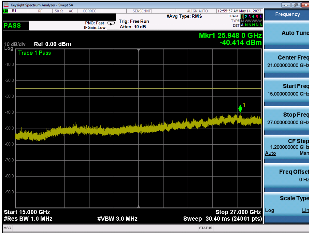
Plot 7-68. Conducted Spurious Plot (NR Band n41 - 100MHz QPSK - RB Size 1, RB Offset 0 - High Channel Ant B)
