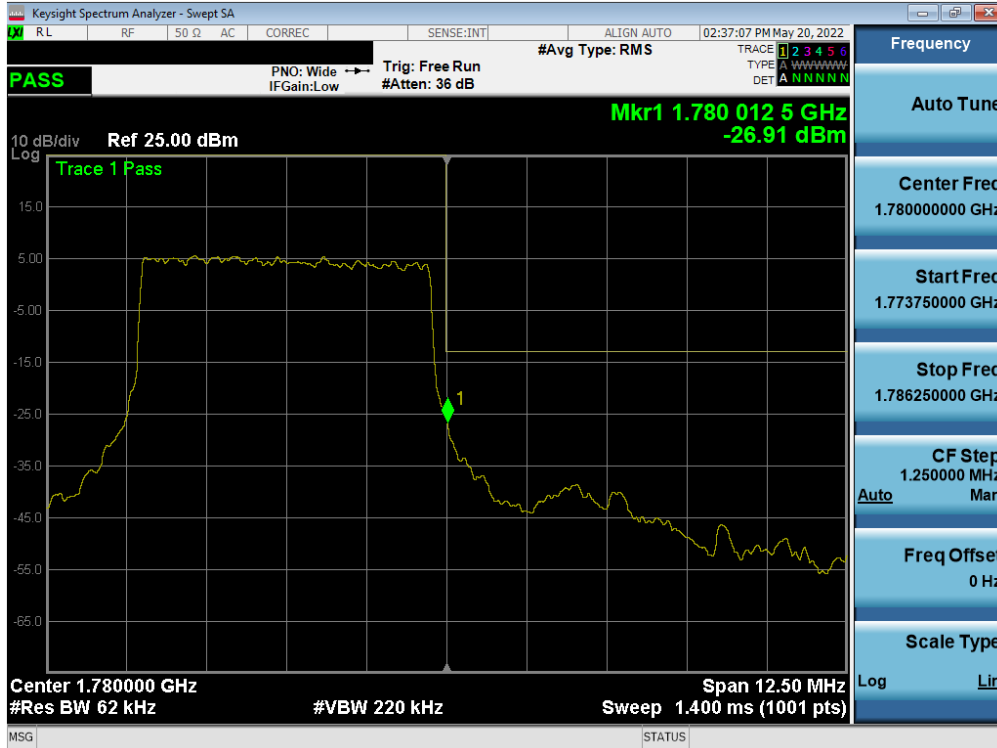
Plot 7-267. Upper Band Edge Plot (NR Band n66 – 5.0MHz - Full RB - Ant F)
