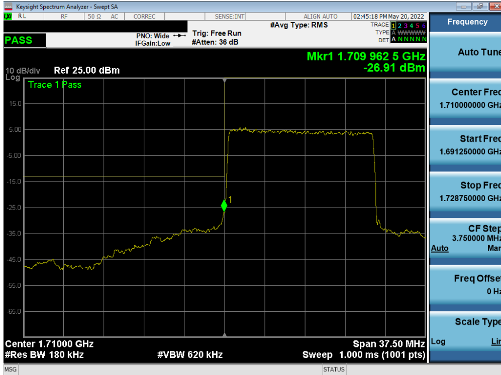
Plot 7-257. Lower Band Edge Plot (NR Band n66 – 15.0MHz - Full RB - Ant F)
