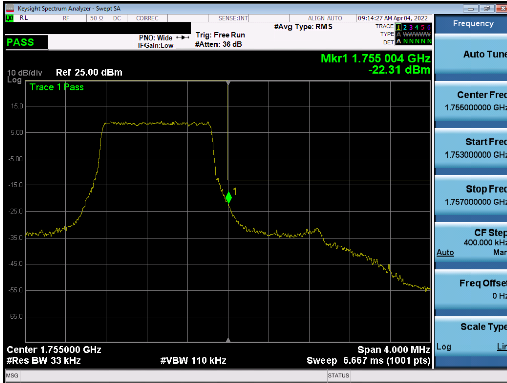
Plot 7-249. Upper Band Edge Plot (LTE Band 4 – 1.4MHz QPSK – Full RB - Ant F)
