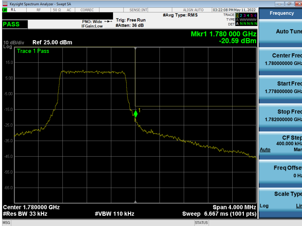
Plot 7-251. Upper Band Edge Plot (LTE Band 66 – 1.4MHz QPSK – Full RB - Ant F)
