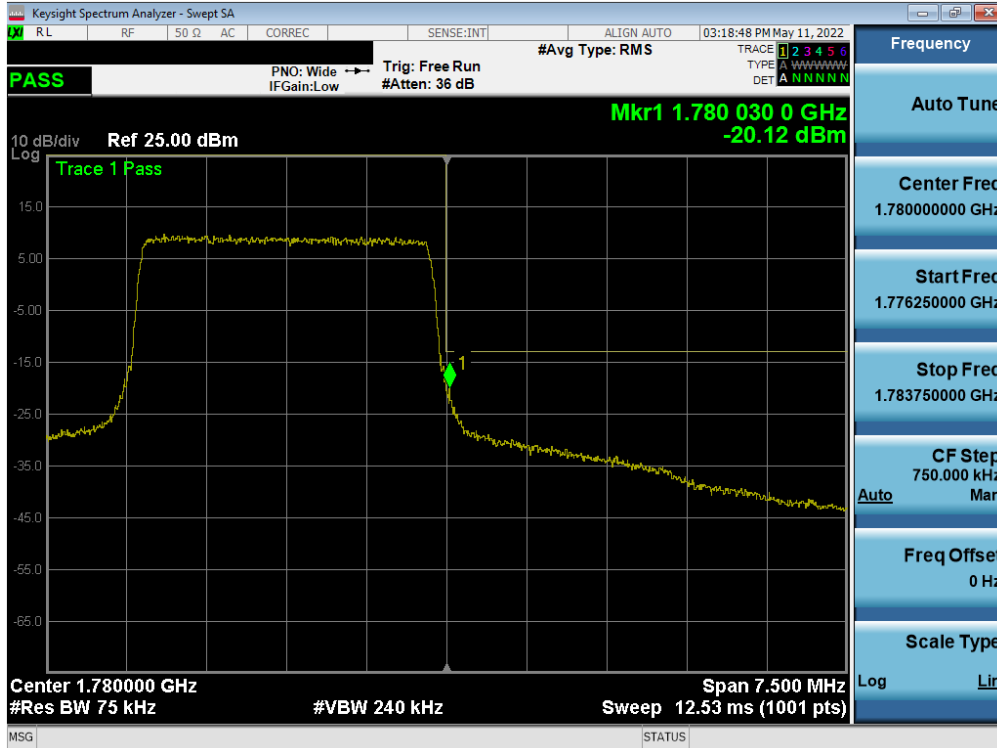
Plot 7-245. Upper Band Edge Plot (LTE Band 66 - 3MHz QPSK – Full RB - Ant F)
