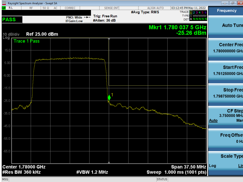
Plot 7-227. Upper Band Edge Plot (LTE Band 66 - 15MHz QPSK – Full RB - Ant F)
