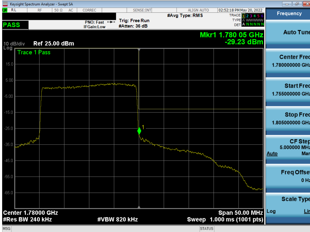
Plot 7-255. Upper Band Edge Plot (NR Band n66 – 20.0MHz - Full RB - Ant F)
