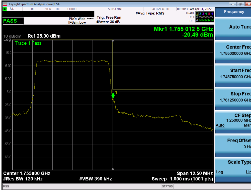
Plot 7-237. Upper Band Edge Plot (LTE Band 4 - 5MHz QPSK – Full RB - Ant F)
