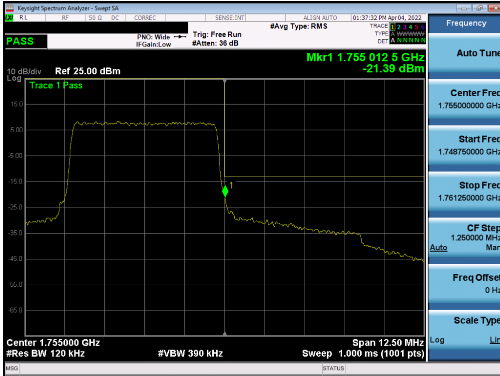
Plot 7-161. Upper Band Edge Plot (LTE Band 4 - 5MHz QPSK – Full RB - Ant B)
