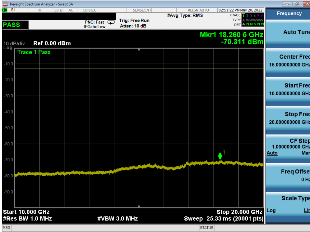
Plot 7-136. Conducted Spurious Plot (NR Band n66 - 20.0MHz - 1 RB - High Channel - Ant F)
