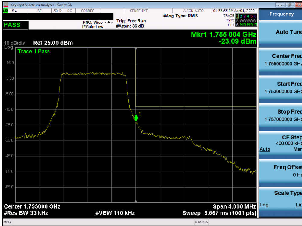
Plot 7-173. Upper Band Edge Plot (LTE Band 4 – 1.4MHz QPSK – Full RB - Ant B)
