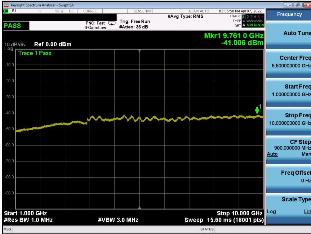
Plot 7-118. Conducted Spurious Plot (NR Band n12 - 15.0MHz - 1 RB - High Channel - Ant A)
