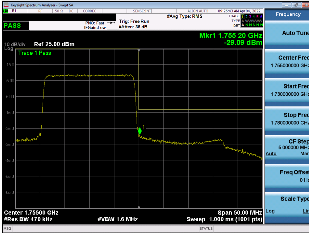
Plot 7-219. Upper Band Edge Plot (LTE Band 4 - 20MHz QPSK – Full RB - Ant F)
