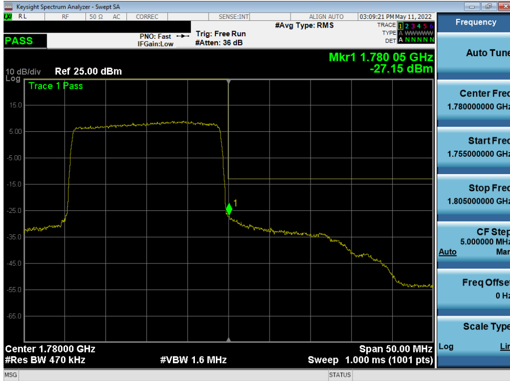
Plot 7-221. Upper Band Edge Plot (LTE Band 66 - 20MHz QPSK - Full RB - Ant F)
