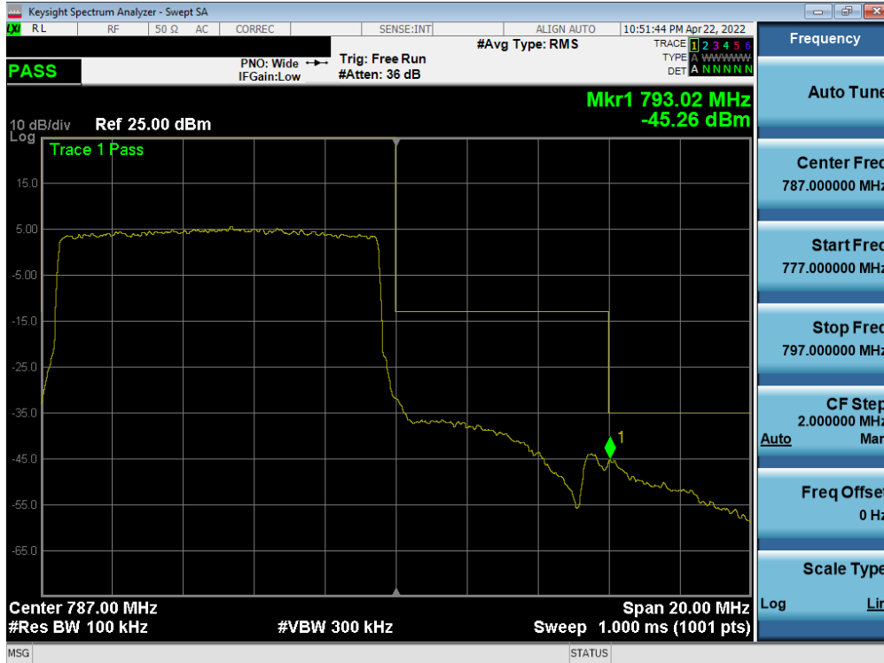
Plot 7-205. Upper Band Edge Plot (LTE Band 13 - 10MHz QPSK – Full RB - Ant A)
