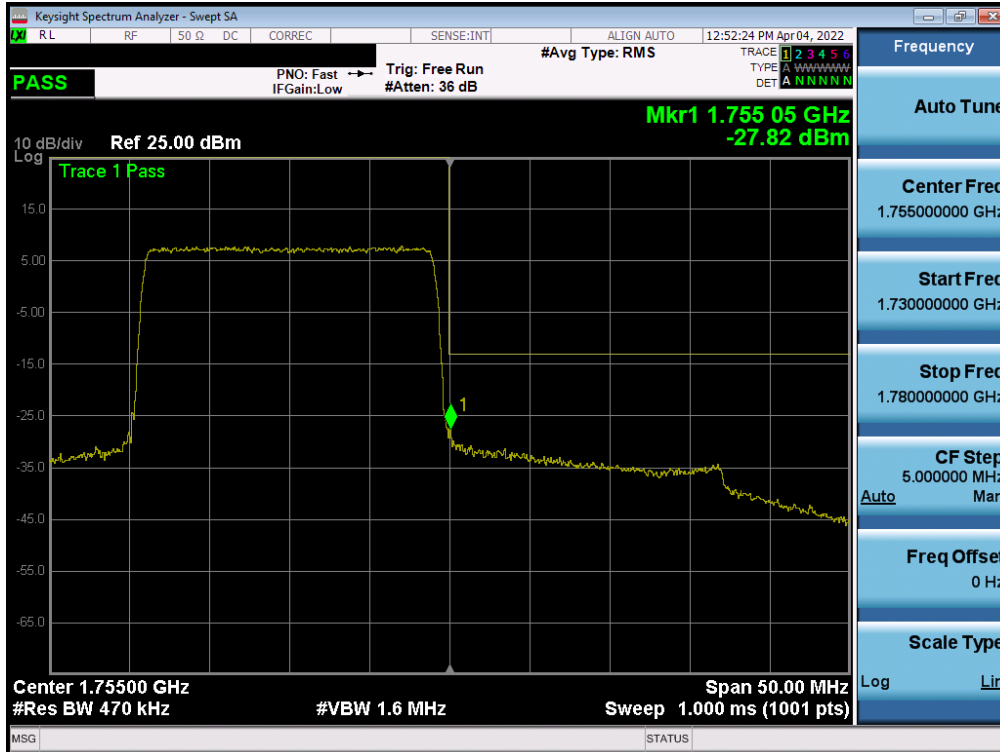
Plot 7-143. Upper Band Edge Plot (LTE Band 4 - 20MHz QPSK – Full RB - Ant B)
