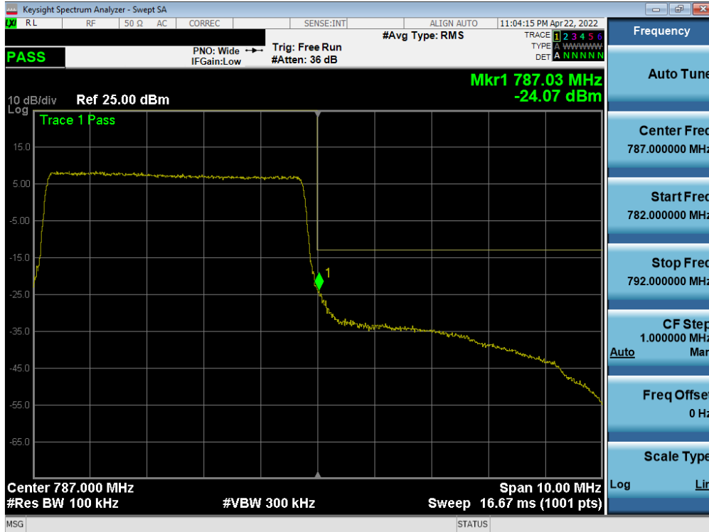
Plot 7-209. Upper Band Edge Plot (LTE Band 13 - 5MHz QPSK - Full RB - Ant A)
