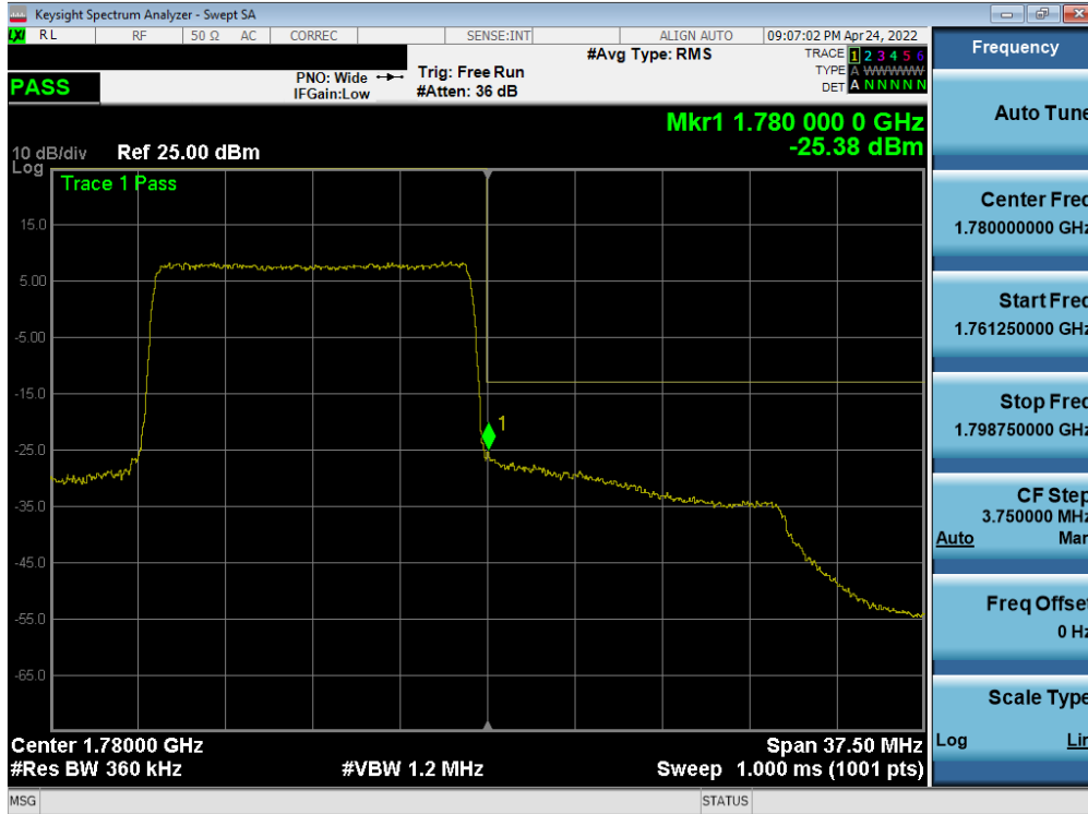
Plot 7-151. Upper Band Edge Plot (LTE Band 66 - 15MHz QPSK – Full RB - Ant B)
