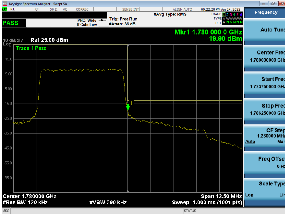
Plot 7-163. Upper Band Edge Plot (LTE Band 66 - 5MHz QPSK – Full RB - Ant B)
