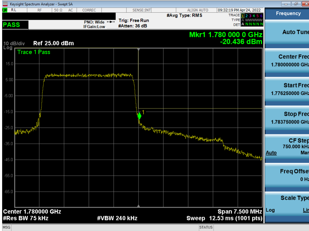
Plot 7-169. Upper Band Edge Plot (LTE Band 66 - 3MHz QPSK – Full RB - Ant B)
