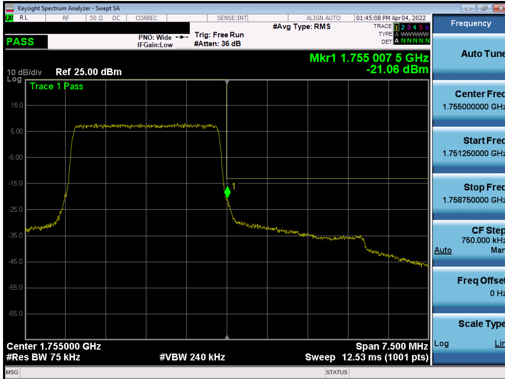
Plot 7-167. Upper Band Edge Plot (LTE Band 4 - 3MHz QPSK – Full RB - Ant B)
