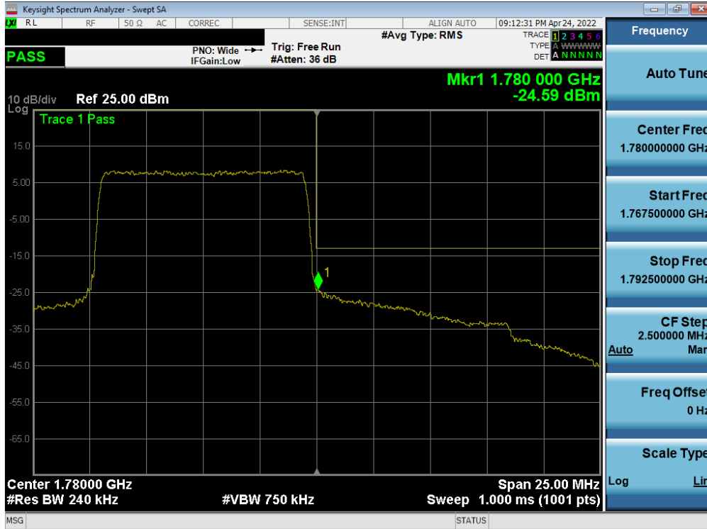
Plot 7-157. Upper Band Edge Plot (LTE Band 66 - 10MHz QPSK – Full RB - Ant B)
