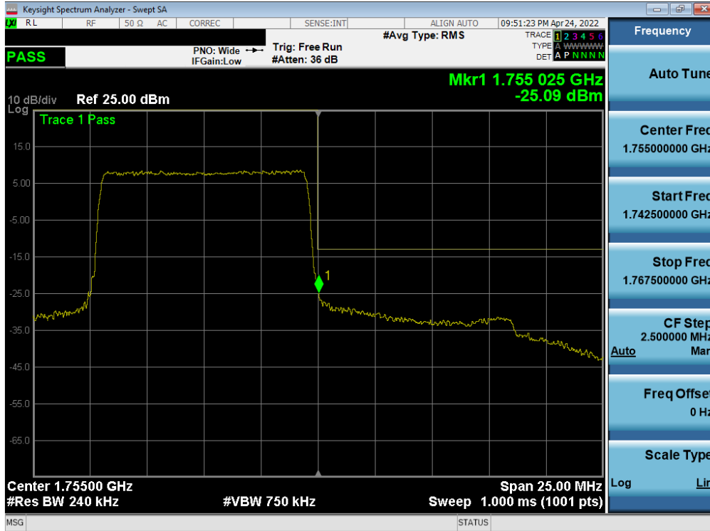
Plot 7-155. Upper Band Edge Plot (LTE Band 4 - 10MHz QPSK – Full RB - Ant B)
