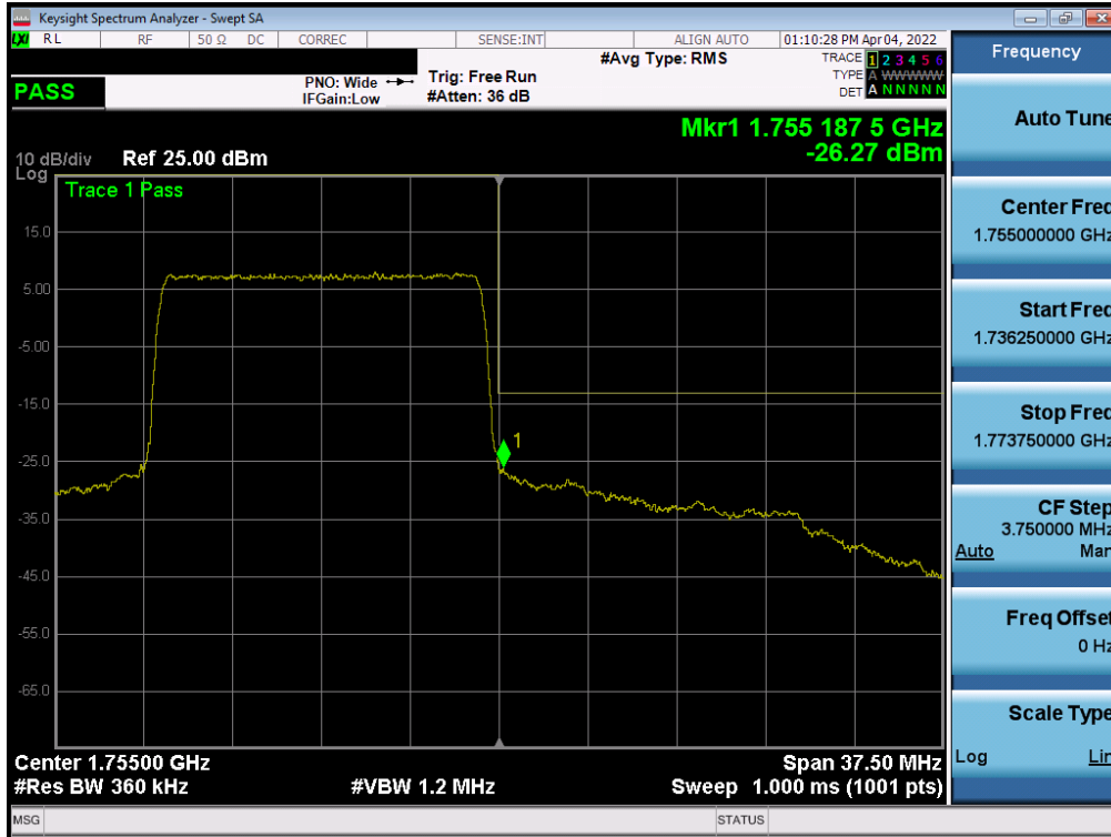
Plot 7-149. Upper Band Edge Plot (LTE Band 4 - 15MHz QPSK – Full RB - Ant B)
