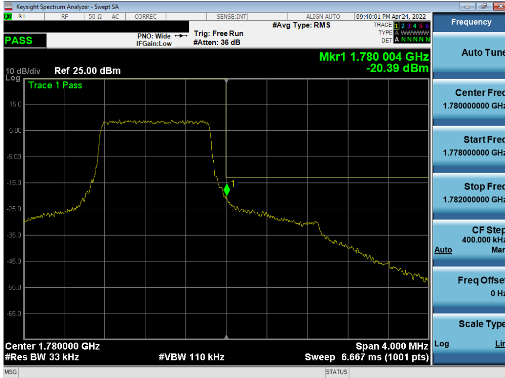
Plot 7-175. Upper Band Edge Plot (LTE Band 66 – 1.4MHz QPSK – Full RB - Ant B)
