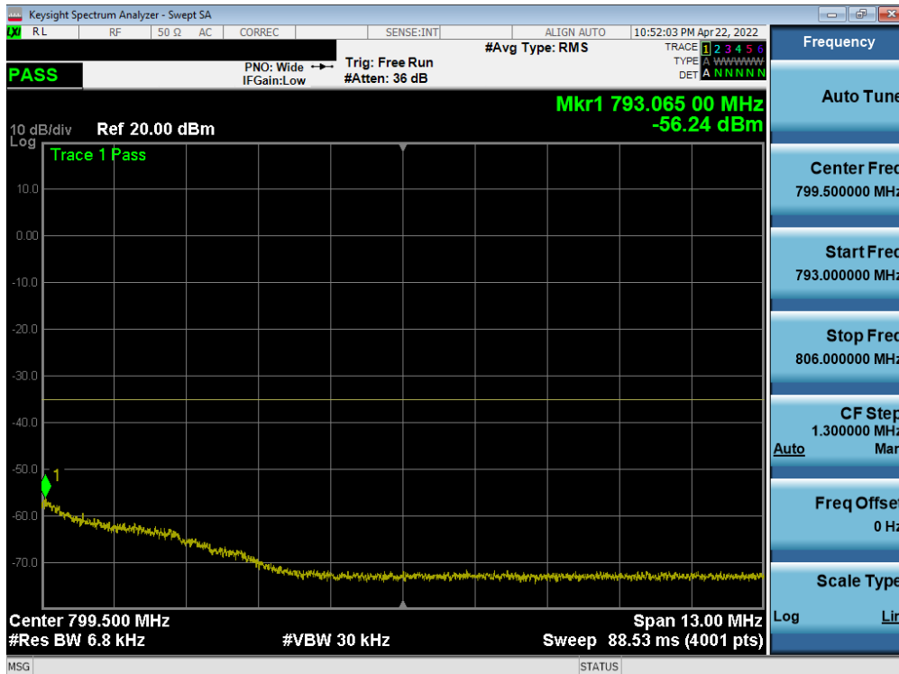
Plot 7-206. Upper Emission Mask Plot (LTE Band 13 - 10MHz QPSK – Full RB - Ant A)
