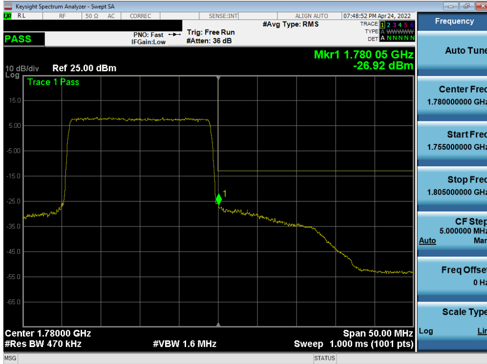
Plot 7-145. Upper Band Edge Plot (LTE Band 66 - 20MHz QPSK - Full RB - Ant B)
