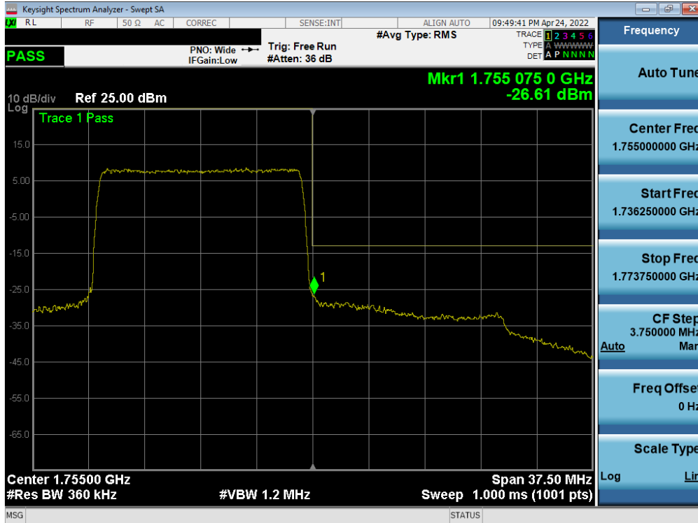
Plot 7-225. Upper Band Edge Plot (LTE Band 4 - 15MHz QPSK – Full RB - Ant F)
