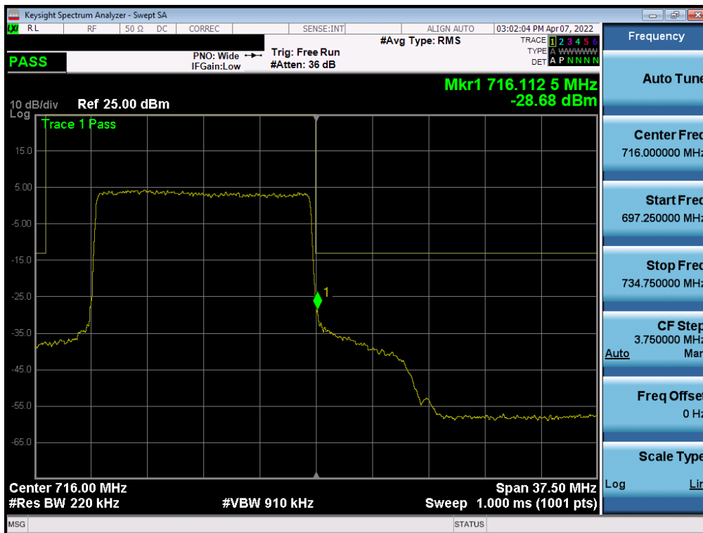
Plot 7-212. Upper Band Edge Plot (NR Band n12 – 15.0MHz - Full RB - Ant A)
