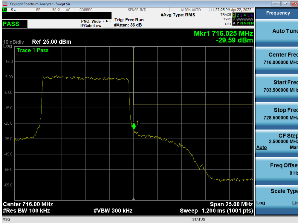
Plot 7-195. Upper Band Edge Plot (LTE Band 12/17 - 10MHz QPSK - Full RB - Ant A)
