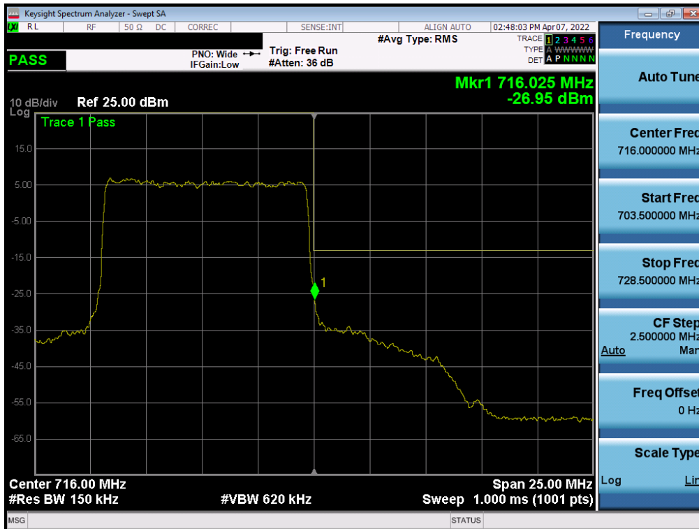
Plot 7-214. Upper Band Edge Plot (NR Band n12 – 10.0MHz - Full RB - Ant A)
