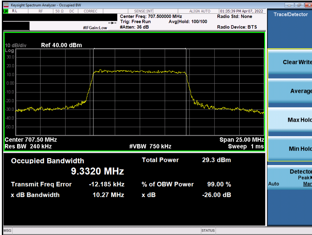
Plot 7-42. Occupied Bandwidth Plot (NR Band n12 - 10MHz CP-OFDM QPSK - Full RB – Ant A)
