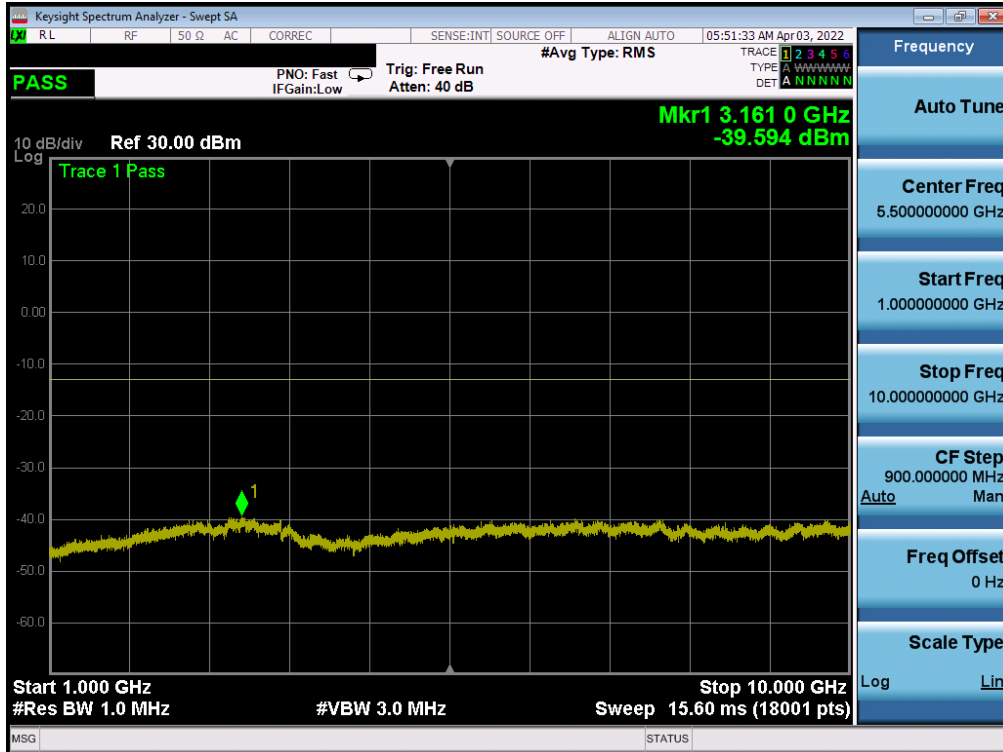
Plot 7-106. Conducted Spurious Plot (LTE Band 12/17 - 10MHz QPSK - 1 RB - High Channel - Ant A)
