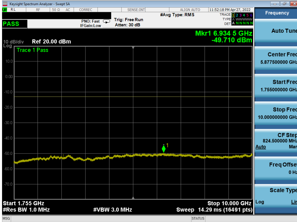
Plot 7-75. Conducted Spurious Plot (WCDMA Ch. 1413- Mid Channel - Ant B)
