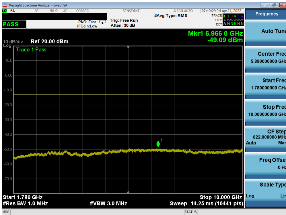
Plot 7-81. Conducted Spurious Plot (LTE Band 66/4 - 20MHz QPSK - 1 RB - Low Channel – Ant B)
