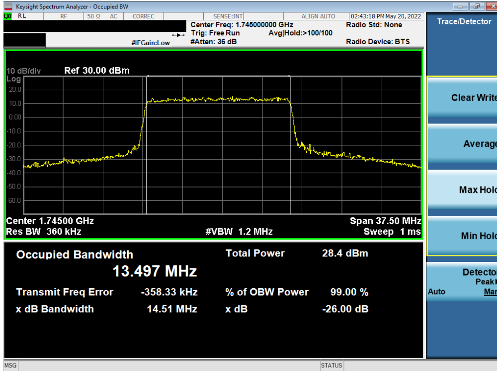
Plot 7-63. Occupied Bandwidth Plot (NR Band n66 - 15.0MHz CP-OFDM QPSK - Full RB - Ant F)
