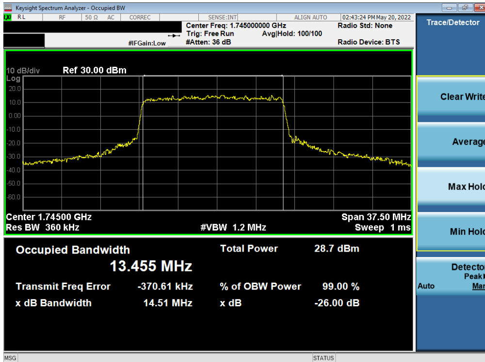
Plot 7-64. Occupied Bandwidth Plot (NR Band n66 - 15.0MHz CP-OFDM 16QAM - Full RB - Ant F)
