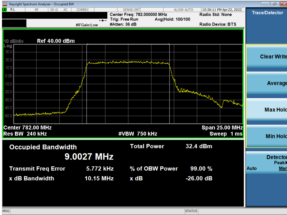
Plot 7-34. Occupied Bandwidth Plot (LTE Band 13 - 10MHz QPSK - Full RB – Ant A)
