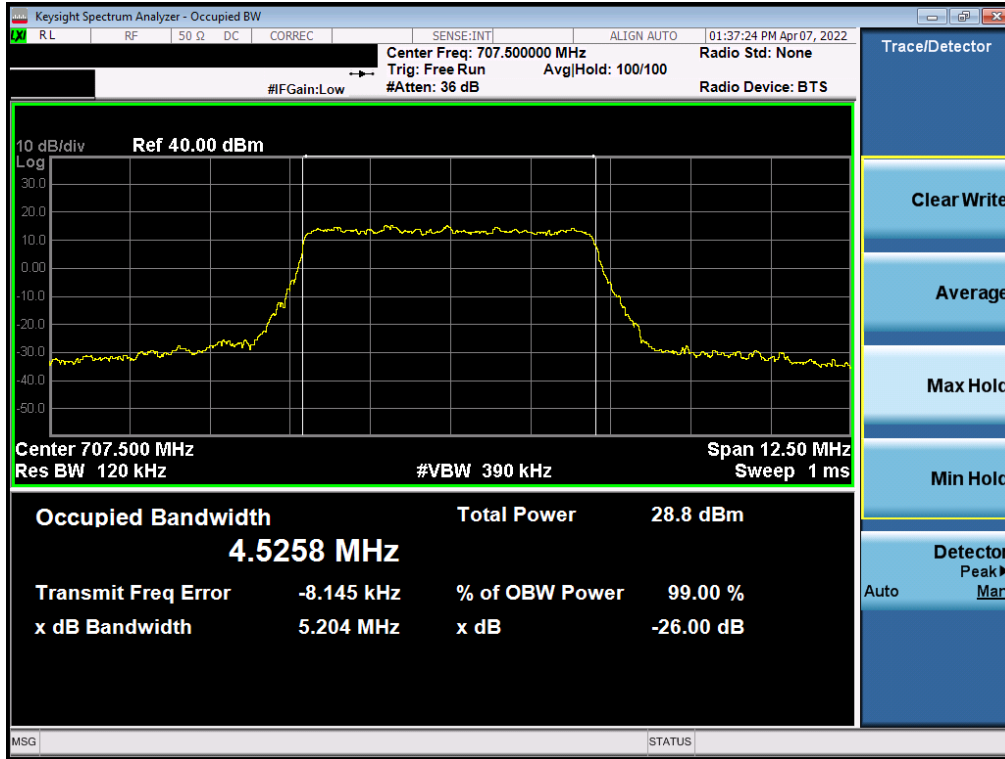
Plot 7-46. Occupied Bandwidth Plot (NR Band n12 - 5MHz CP-OFDM 16-QAM - Full RB – Ant A)
