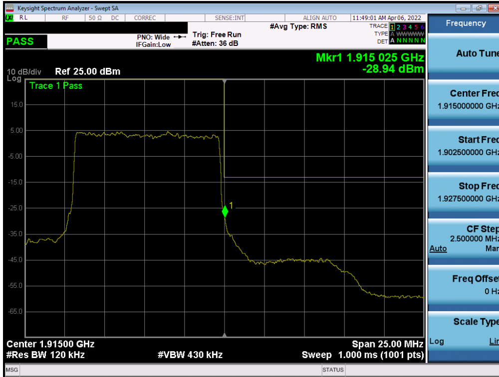
Plot 7-116. Upper Band Edge Plot (NR Band n25 - 10MHz QPSK – Full RB - Ant B)
