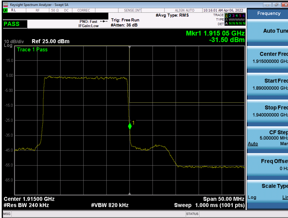
Plot 7-104. Upper Band Edge Plot (NR Band n25 - 20MHz QPSK – Full RB - Ant B)
