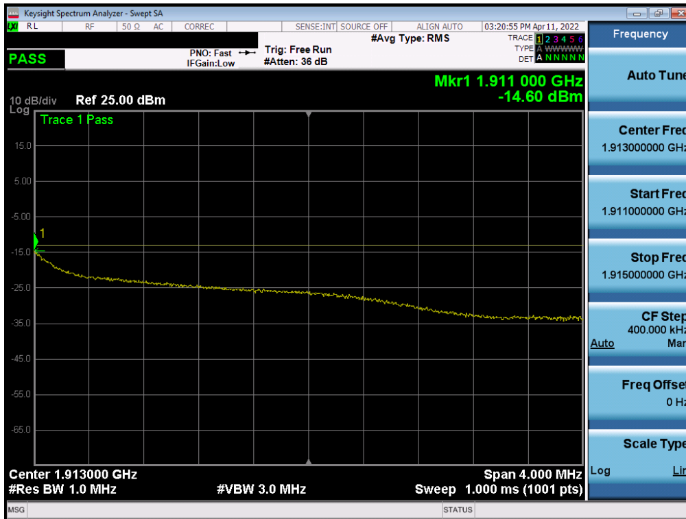
Plot 7-129. Extended Upper Band Edge Plot (WCDMA PCS – Ch. 9538 - Ant B)
