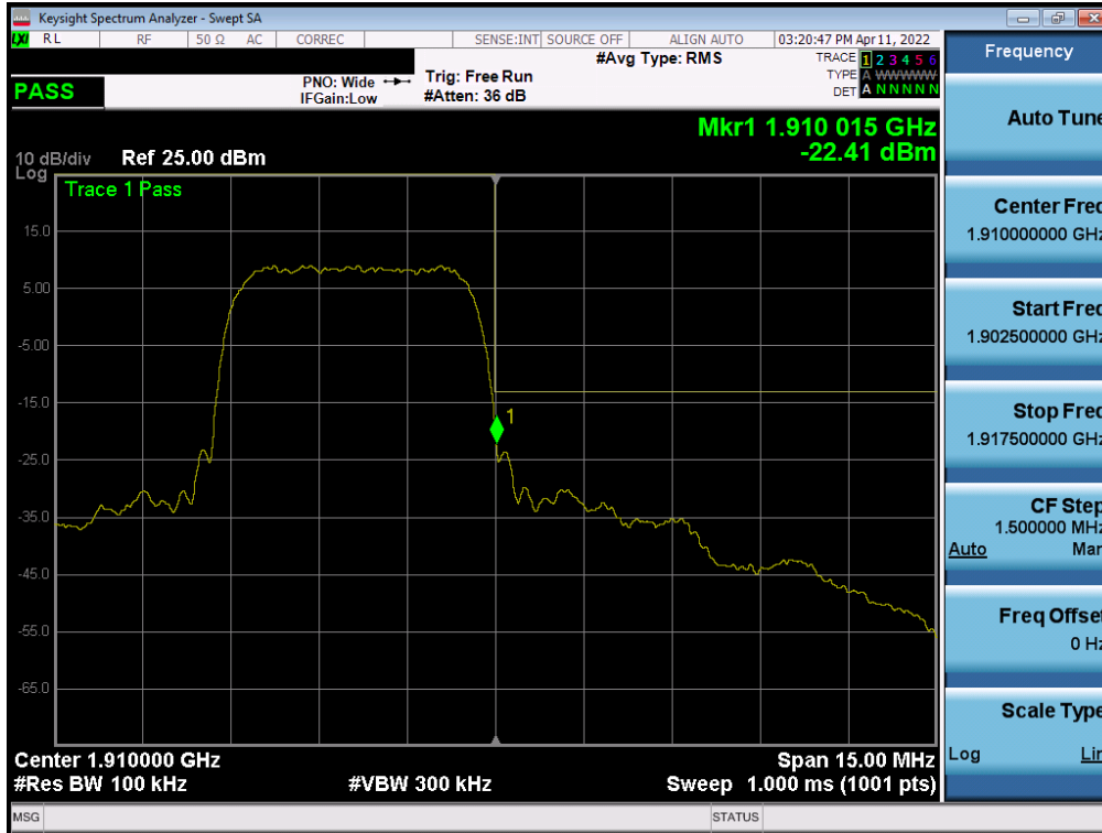
Plot 7-128. Upper Band Edge Plot (WCDMA PCS – Ch. 9538 - Ant B)
