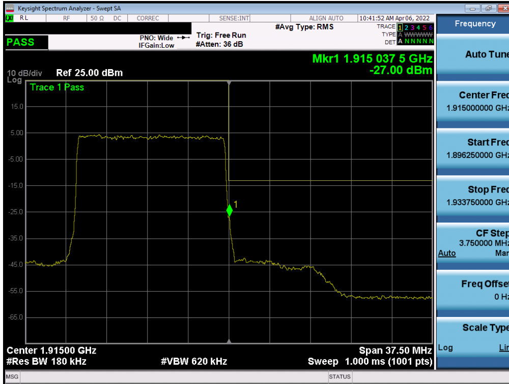
Plot 7-110. Upper Band Edge Plot (NR Band n25 - 15MHz QPSK – Full RB - Ant B)
