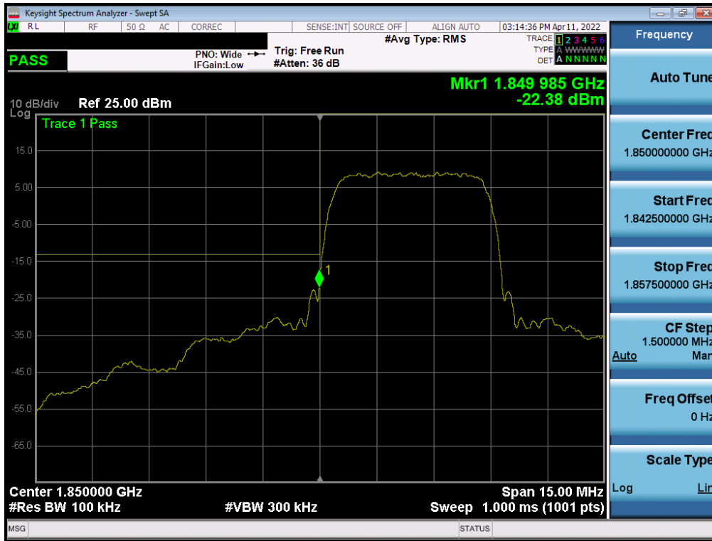
Plot 7-126. Lower Band Edge Plot (WCDMA PCS – Ch. 9262 - Ant B)
