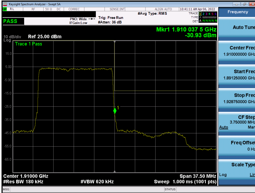
Plot 7-108. Upper Band Edge Plot (NR Band n2 - 15MHz QPSK – Full RB - Ant B)
