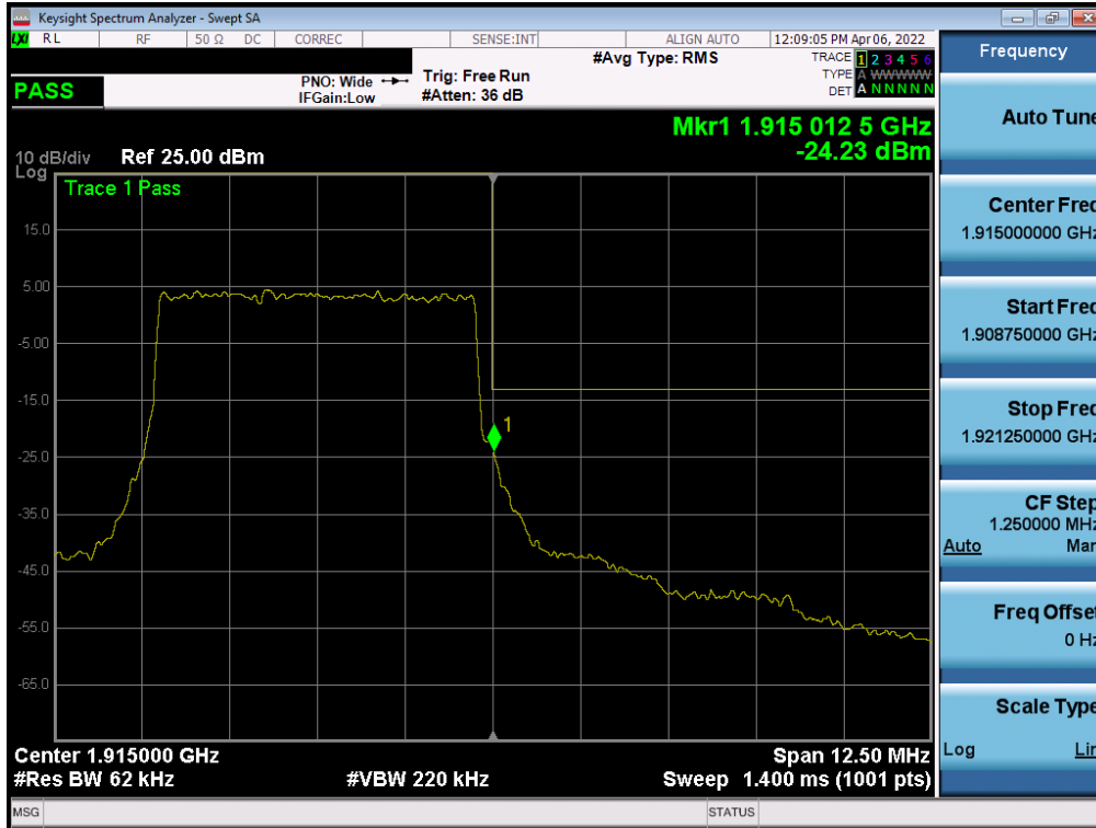
Plot 7-122. Upper Band Edge Plot (NR Band n25 – 5MHz QPSK – Full RB - Ant B)
