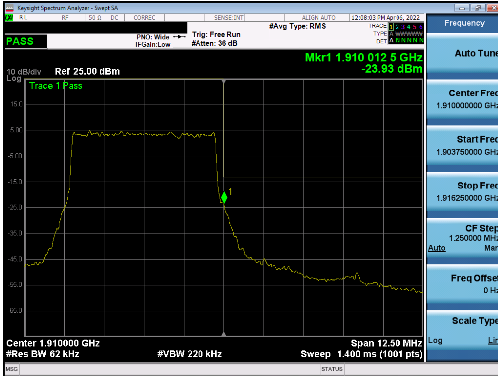
Plot 7-120. Upper Band Edge Plot (NR Band n2 – 5MHz QPSK – Full RB - Ant B)
