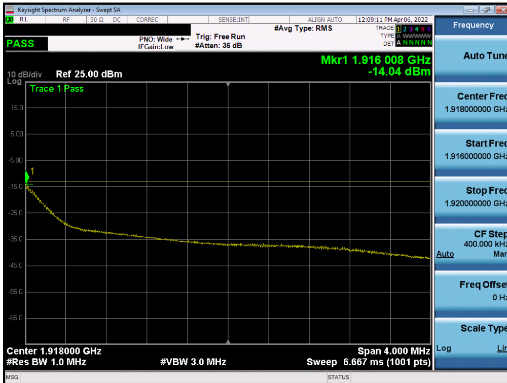
Plot 7-123. Extended Upper Band Edge Plot (NR Band n25 – 5MHz QPSK – Full RB - Ant B)
