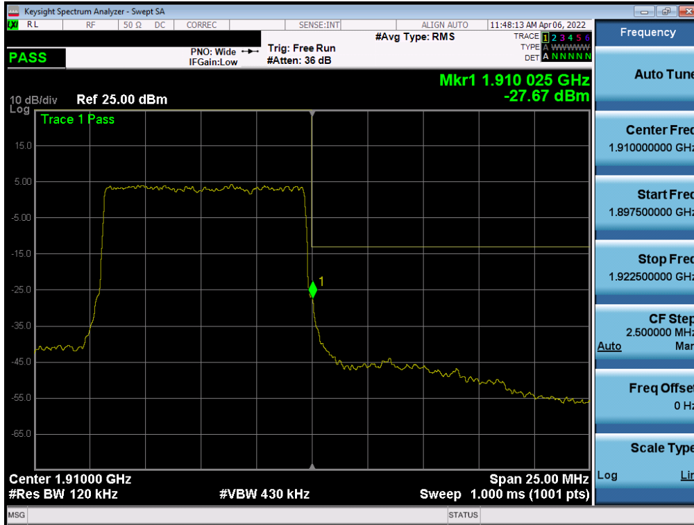
Plot 7-114. Upper Band Edge Plot (NR Band n2 - 10MHz QPSK – Full RB - Ant B)
