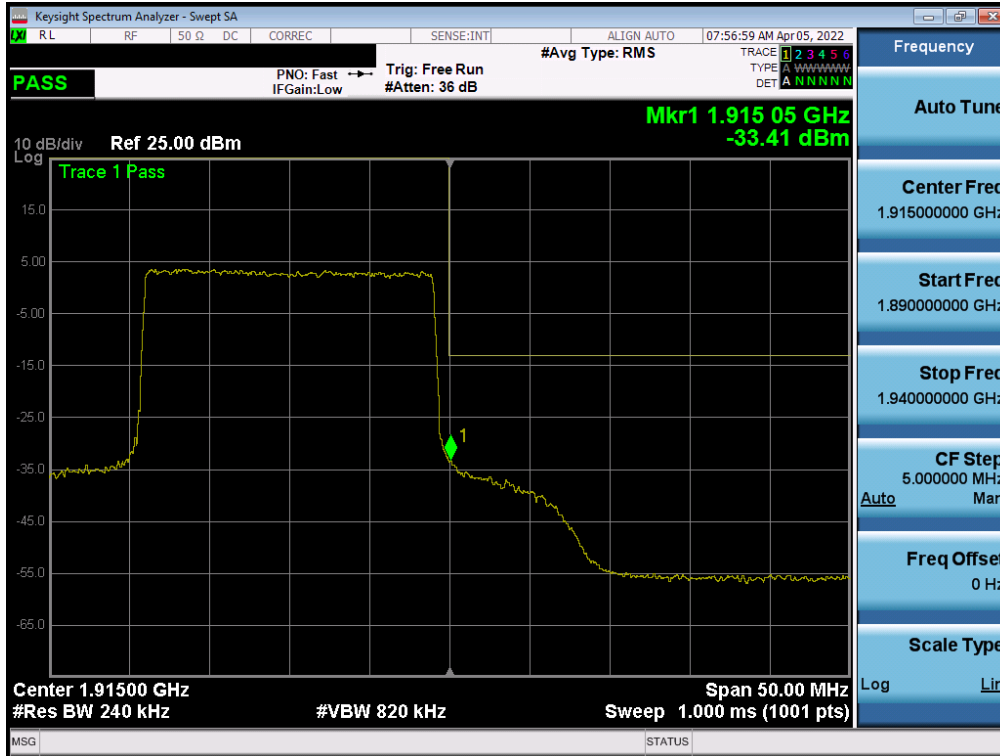
Plot 7-68. Upper Band Edge Plot (LTE Band 25 - 20MHz QPSK – Full RB - Ant B)
