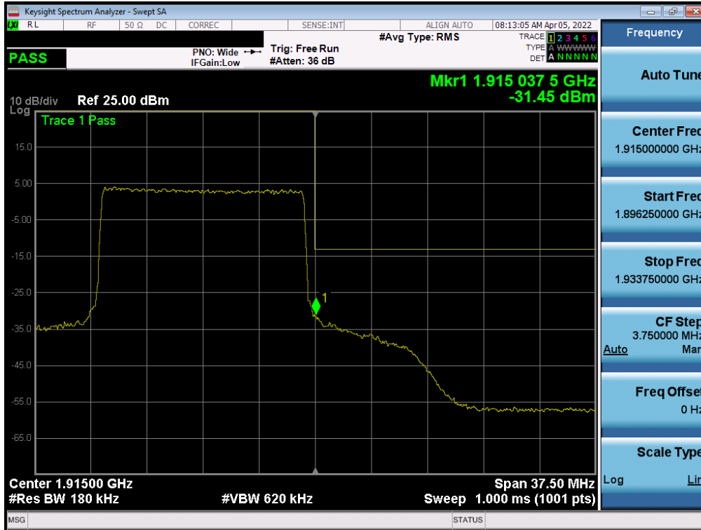
Plot 7-74. Upper Band Edge Plot (LTE Band 25 - 15MHz QPSK – Full RB - Ant B)
