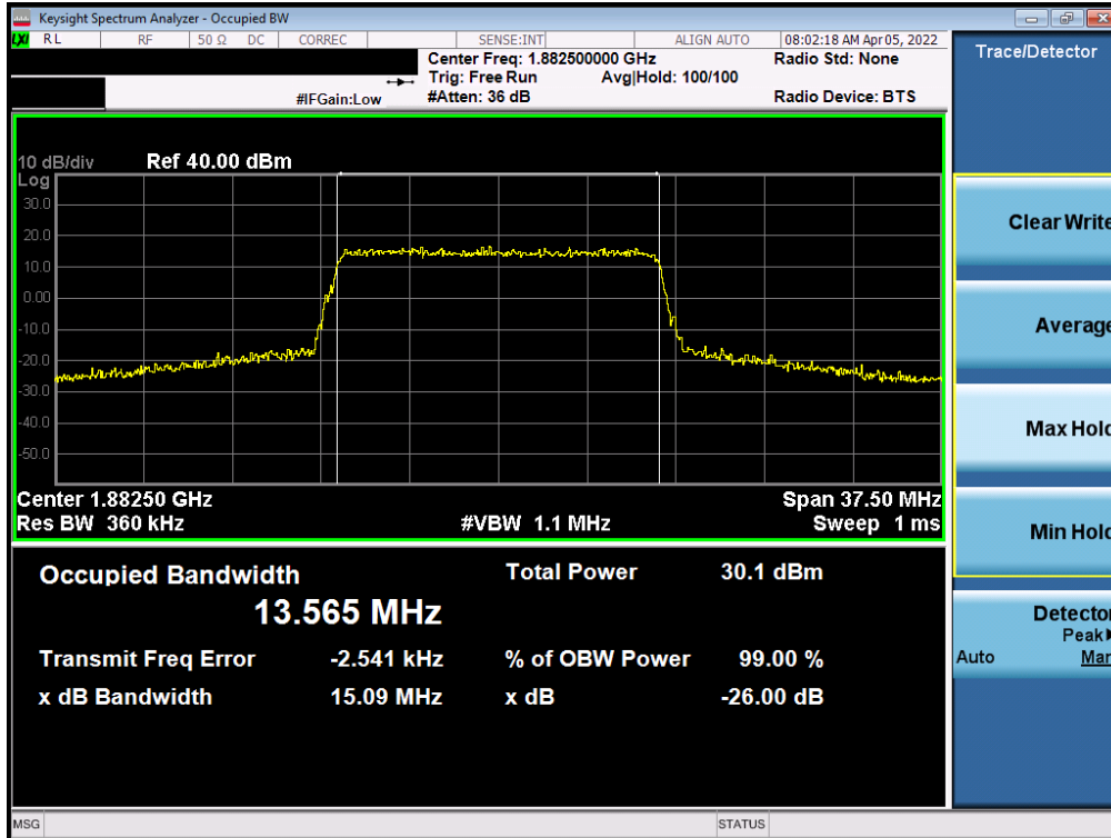
Plot 7-6. Occupied Bandwidth Plot (LTE Band 25/2 - 15MHz QPSK - Full RB - Ant B)
