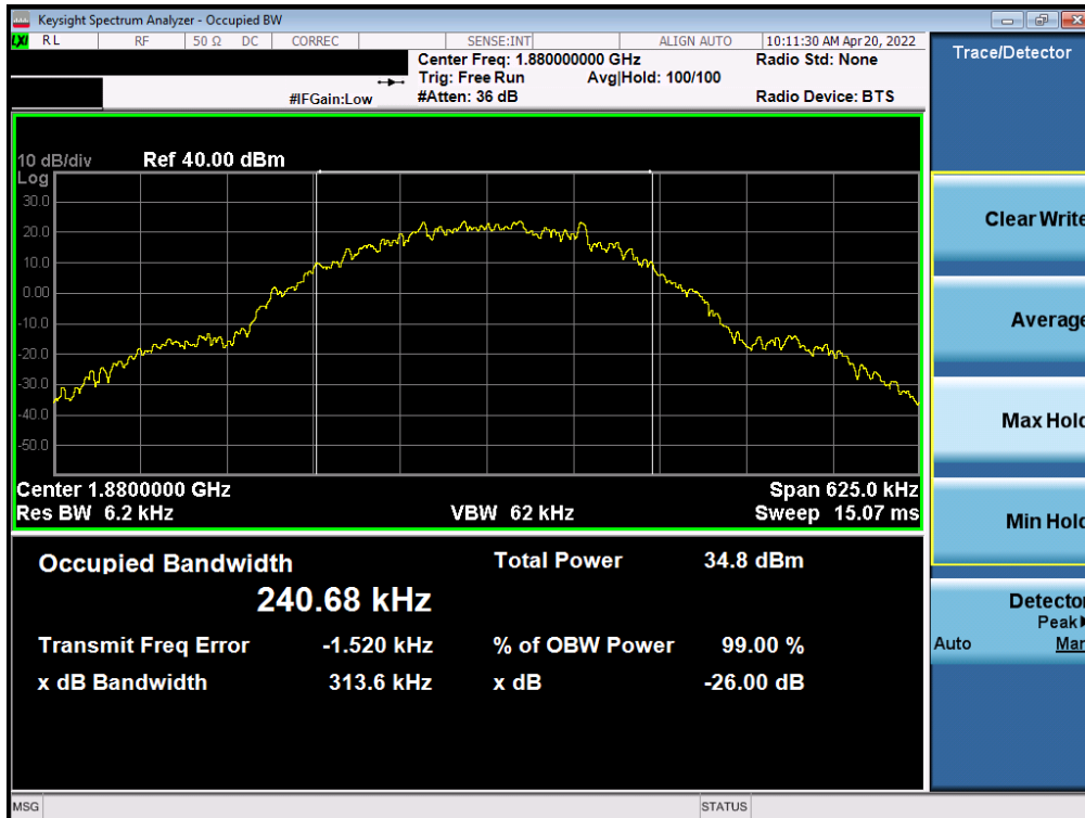
Plot 7-2. Occupied Bandwidth Plot (EDGE, Ch. 661 - Ant B)
