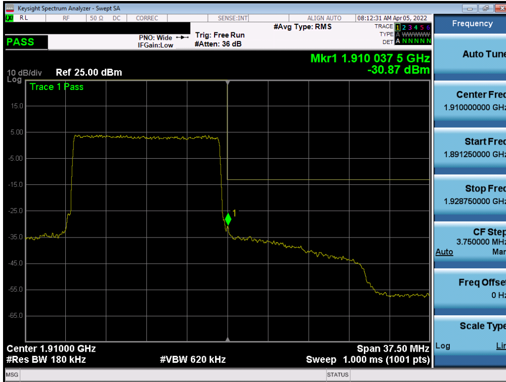
Plot 7-72. Upper Band Edge Plot (LTE Band 2 - 15MHz QPSK – Full RB - Ant B)
