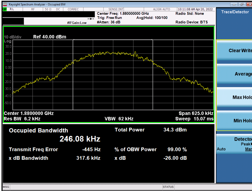
Plot 7-1. Occupied Bandwidth Plot (GPRS, Ch. 661 - Ant B)
