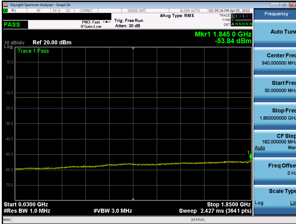
Plot 7-43. Conducted Spurious Plot (NR Band n25/2 - 20.0MHz - 1RB - High Channel - Ant B)
