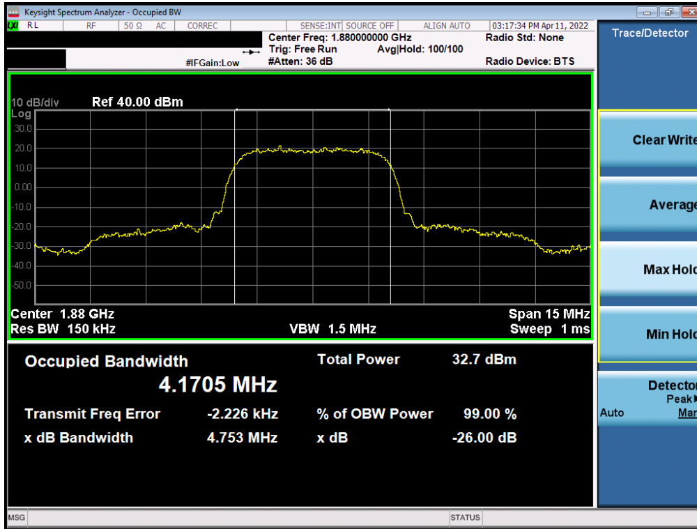
Plot 7-3. Occupied Bandwidth Plot (WCDMA, Ch. 9400 - Ant B)
