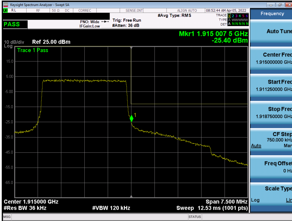
Plot 7-92. Upper Band Edge Plot (LTE Band 25 - 3MHz QPSK – Full RB - Ant B)
