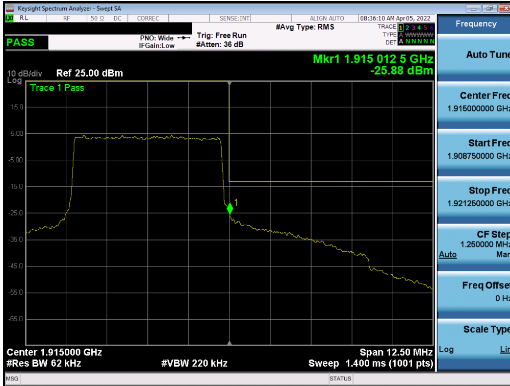
Plot 7-86. Upper Band Edge Plot (LTE Band 25 - 5MHz QPSK – Full RB - Ant B)
