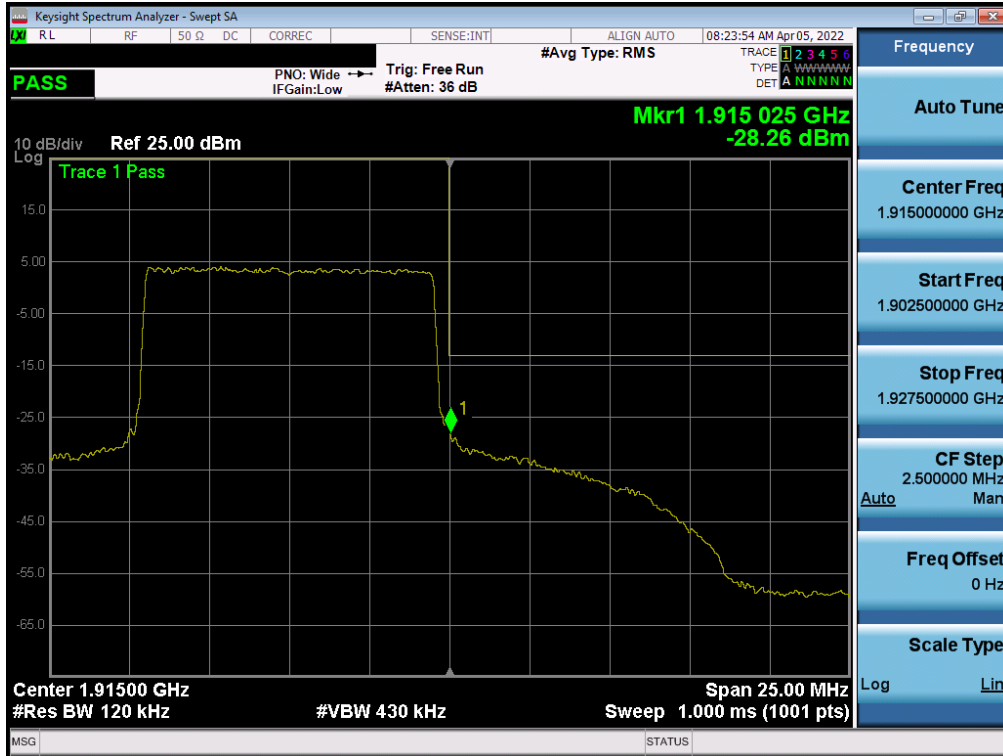
Plot 7-80. Upper Band Edge Plot (LTE Band 25 - 10MHz QPSK – Full RB - Ant B)
