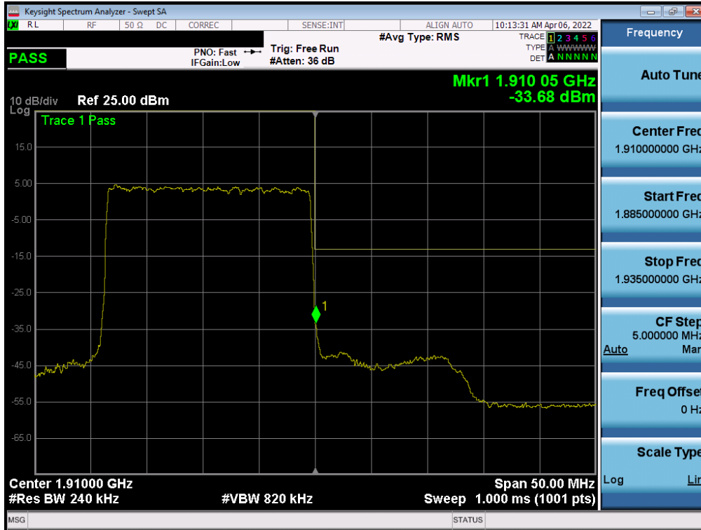
Plot 7-102. Upper Band Edge Plot (NR Band n2 - 20MHz QPSK – Full RB - Ant B)
