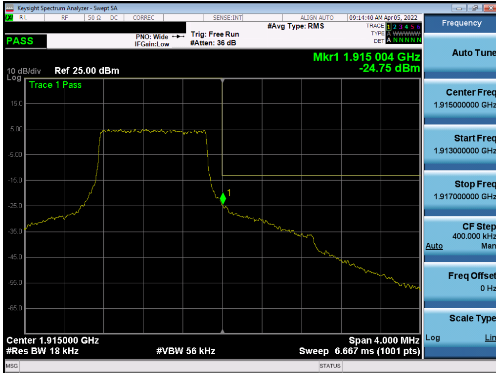
Plot 7-98. Upper Band Edge Plot (LTE Band 25 – 1.4MHz QPSK – Full RB - Ant B)
