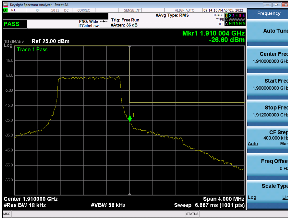
Plot 7-96. Upper Band Edge Plot (LTE Band 2 – 1.4MHz QPSK – Full RB - Ant B)
