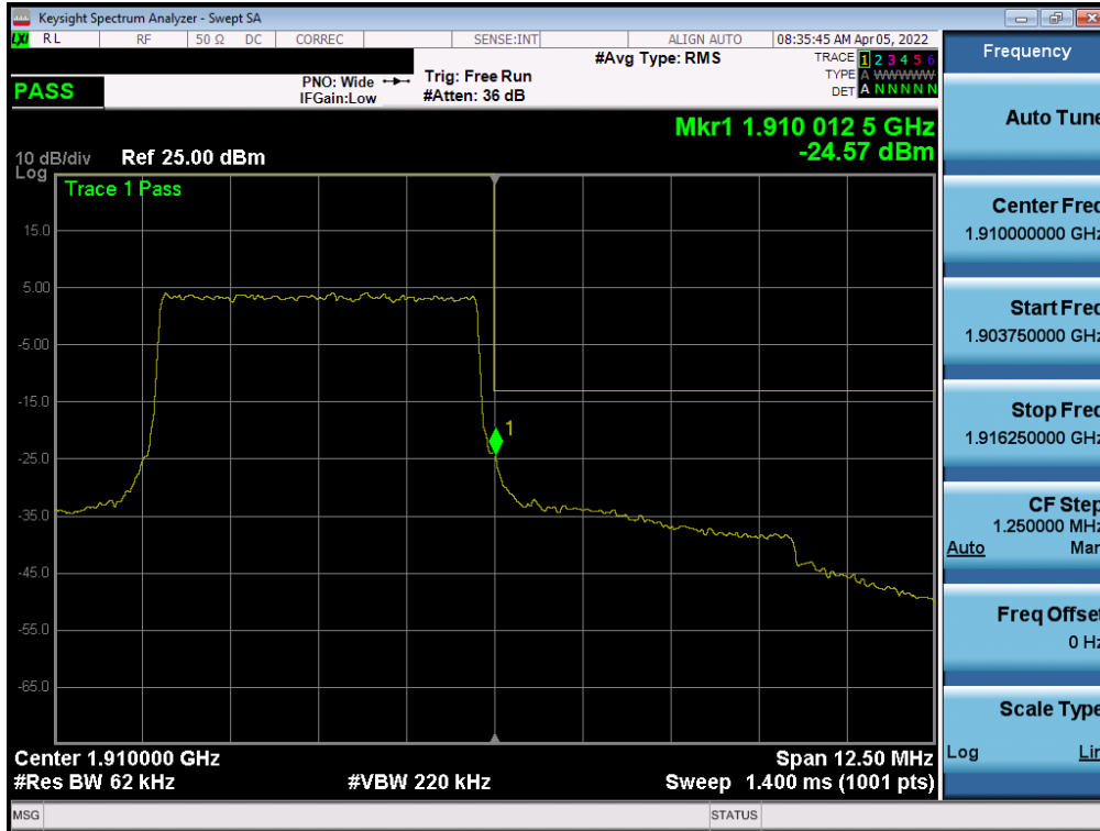
Plot 7-84. Upper Band Edge Plot (LTE Band 2 - 5MHz QPSK – Full RB - Ant B)
