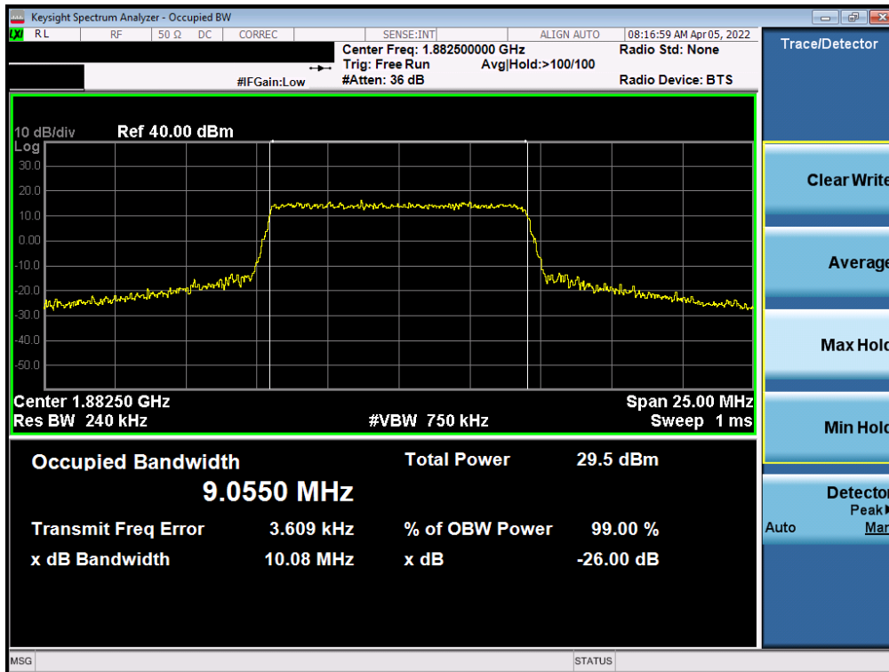
Plot 7-9. Occupied Bandwidth Plot (LTE Band 25/2 - 10MHz 16-QAM - Full RB - Ant B)
