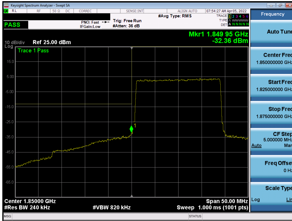
Plot 7-64. Lower Band Edge Plot (LTE Band 25/2 - 20MHz QPSK – Full RB - Ant B)
