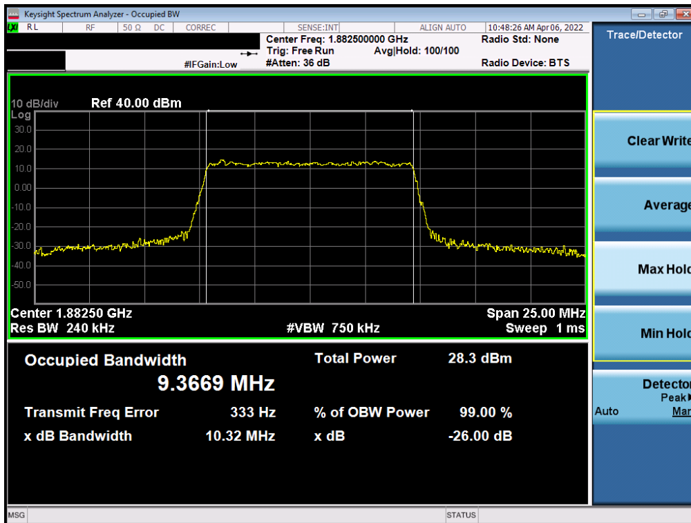
Plot 7-23. Occupied Bandwidth Plot (NR Band n25/2 - 10.0MHz CP-OFDM QPSK - Full RB - Ant B)
