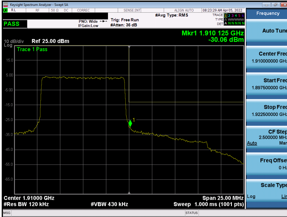
Plot 7-78. Upper Band Edge Plot (LTE Band 2 - 10MHz QPSK – Full RB - Ant B)
