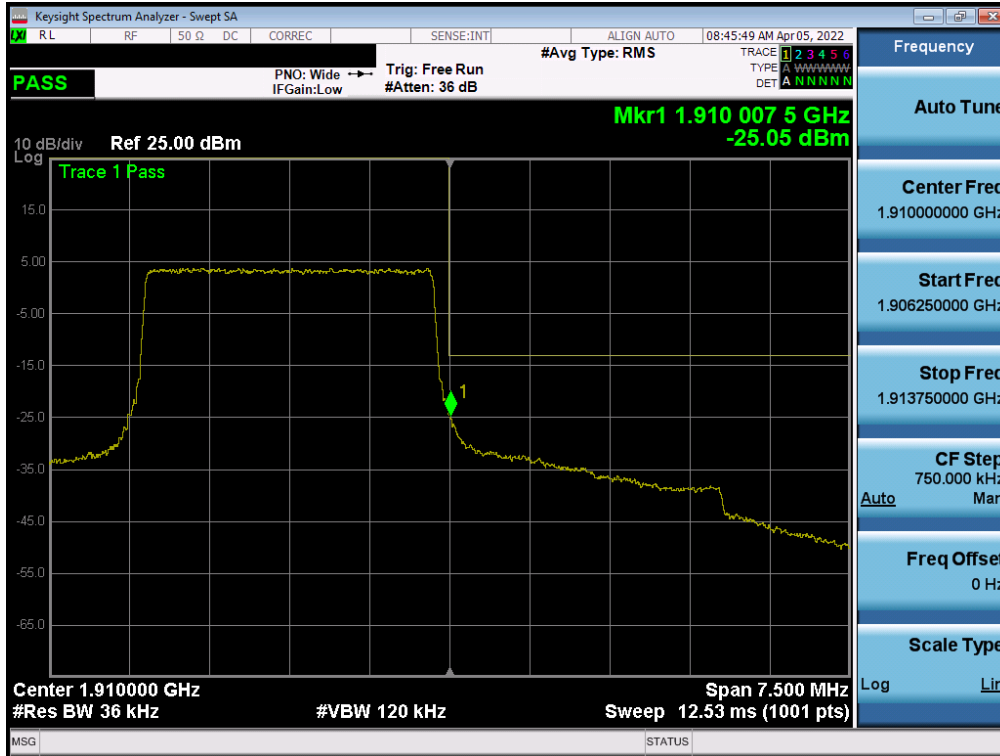
Plot 7-90. Upper Band Edge Plot (LTE Band 2 - 3MHz QPSK – Full RB - Ant B)
