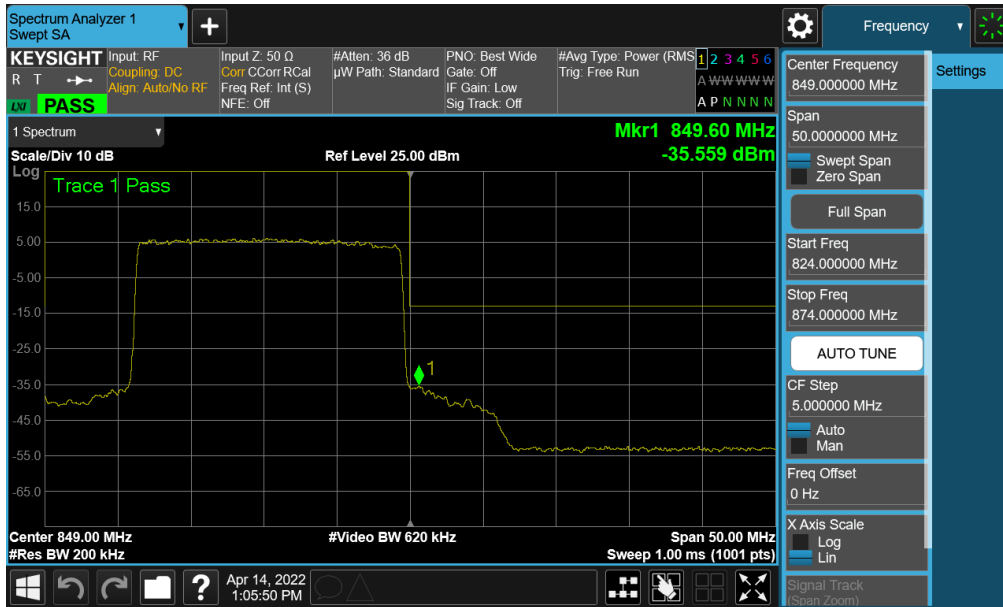
Plot 7-73. Upper Band Edge Plot (NR Band n5 – 20.0MHz - Full RB)
