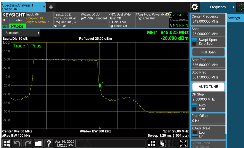
Plot 7-77. Upper Band Edge Plot (NR Band n5 – 10.0MHz - Full RB)
